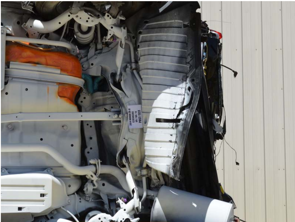
FIGURE 26. Post-Test Rear Underbody View of Test Vehicle
