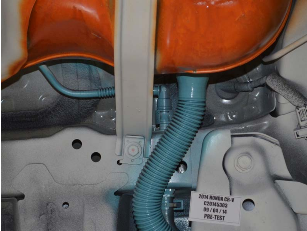
FIGURE 29. Pre-Test Underbody View of Fuel Filler Neck
