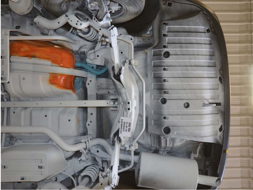
FIGURE 25. Pre-Test Rear Underbody View of Test Vehicle
