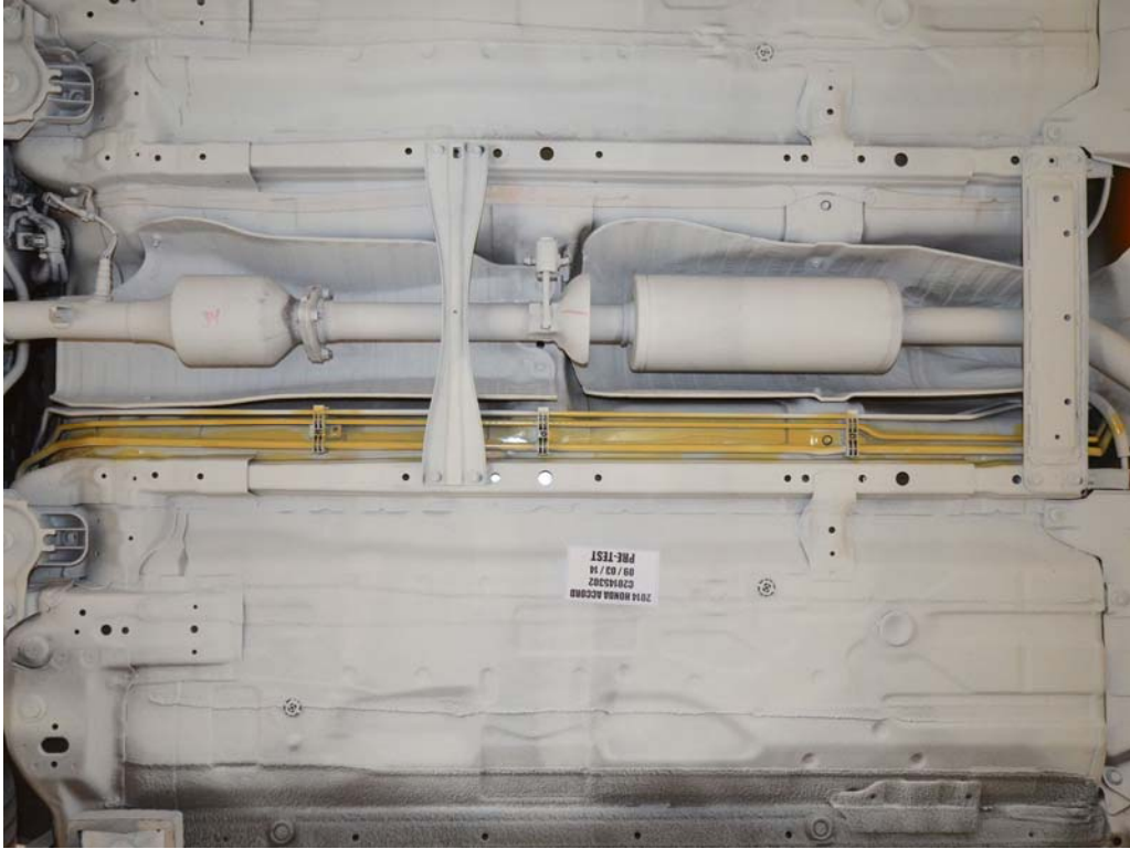
FIGURE 31. Pre-Test Underbody View of Fuel Lines
