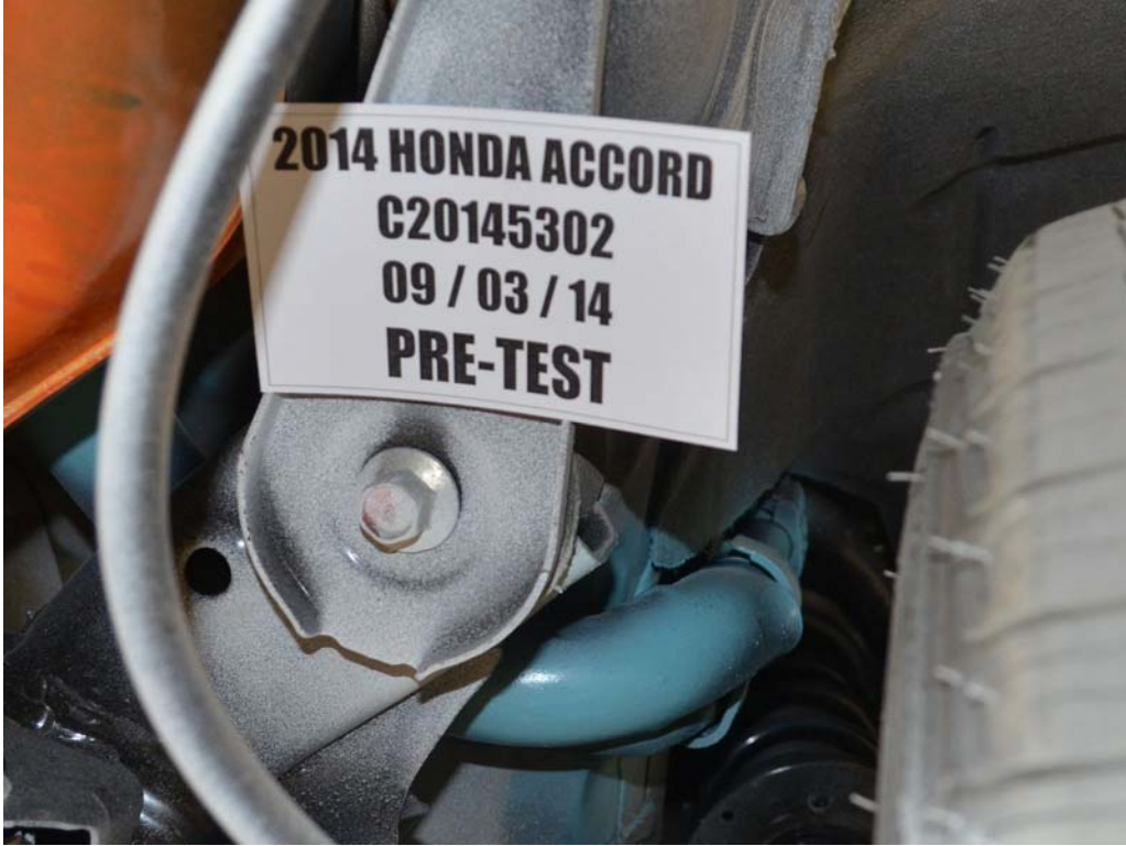
FIGURE 29. Pre-Test Underbody View of Fuel Filler Neck
