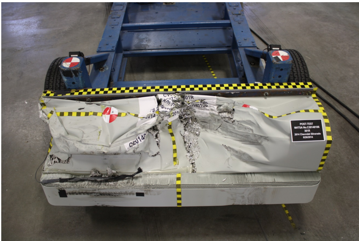
Figure A-26: Post-Test MDB Top View
