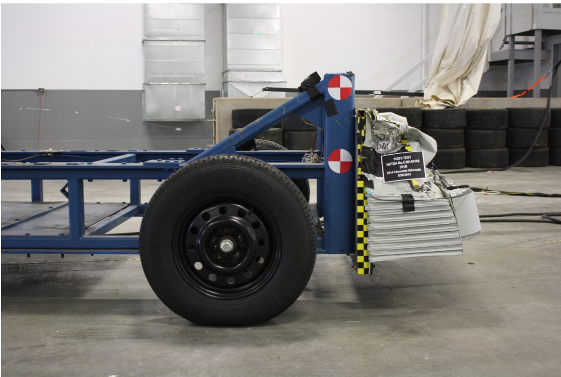
Figure A-24: Post-Test MDB Right Side View
