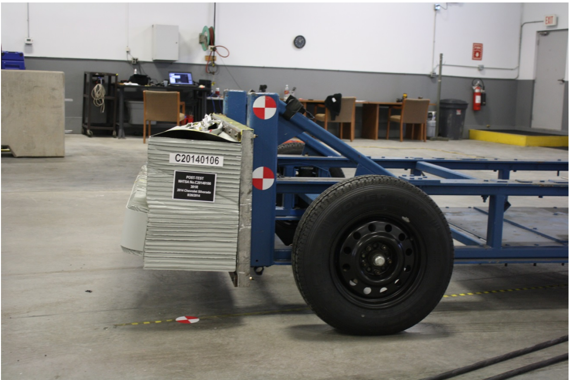
Figure A-22: Post-Test MDB Left Side View
