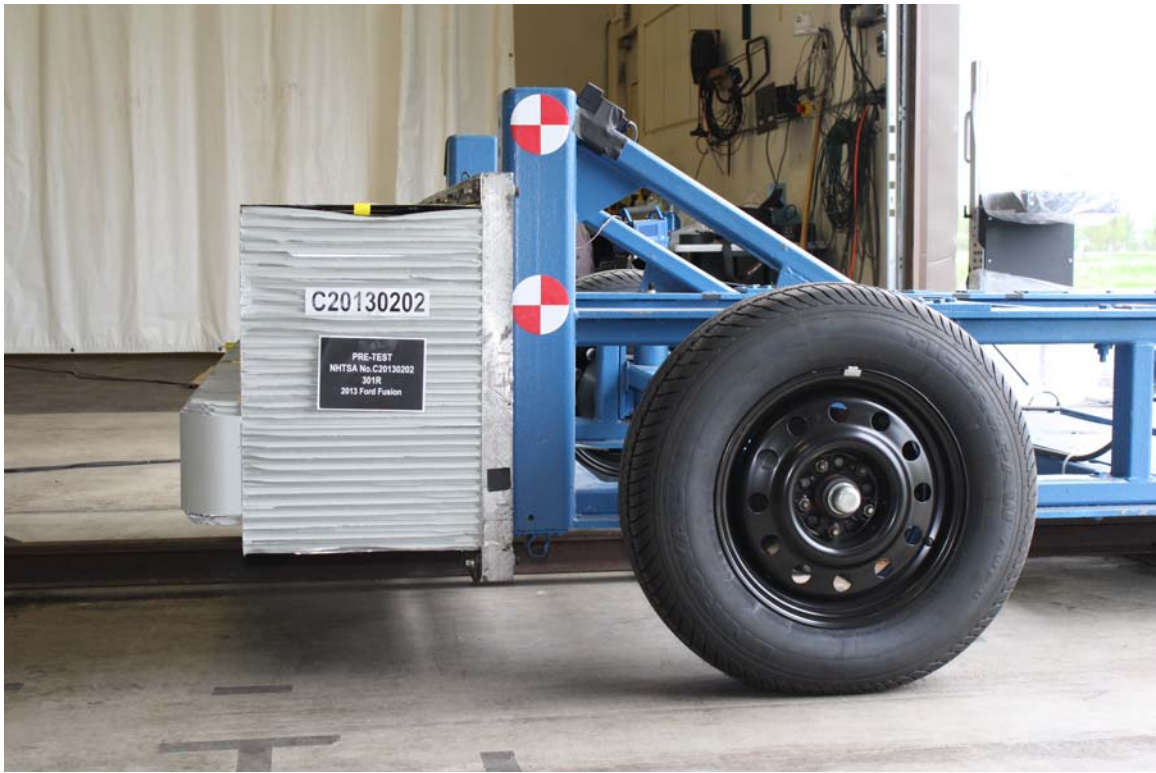
Figure A-21: Pre-Test MDB Left Side View
