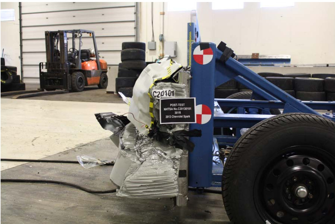
Figure A-22: Post-Test MDB Left Side View
