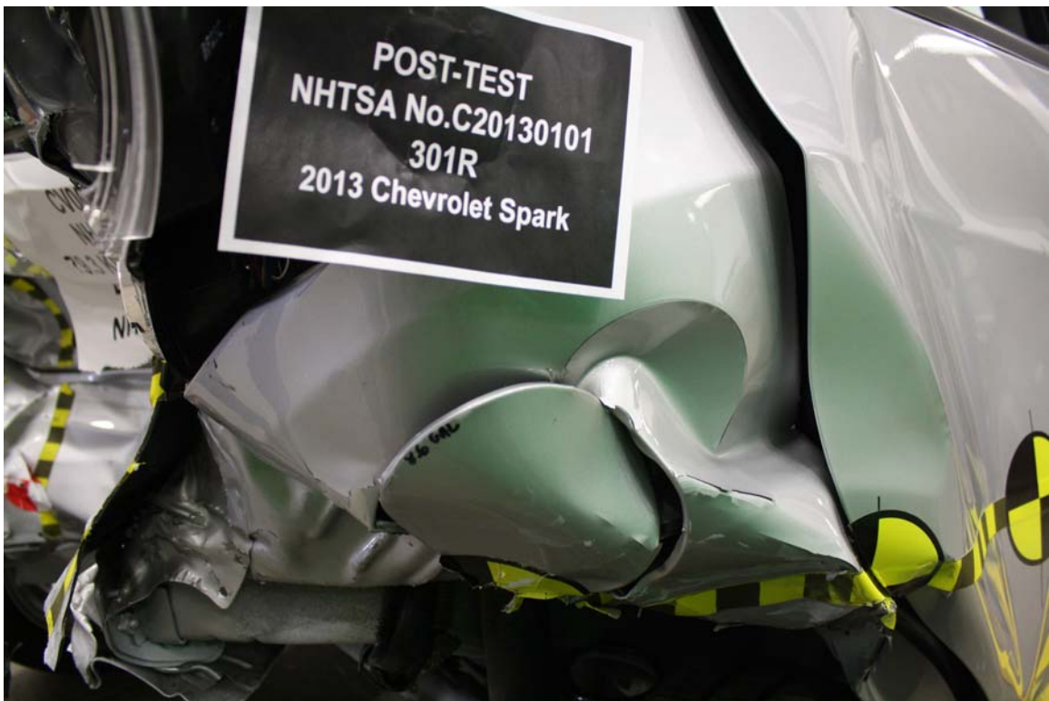
Figure A-36: Post-Test Fuel Filler Cap View
