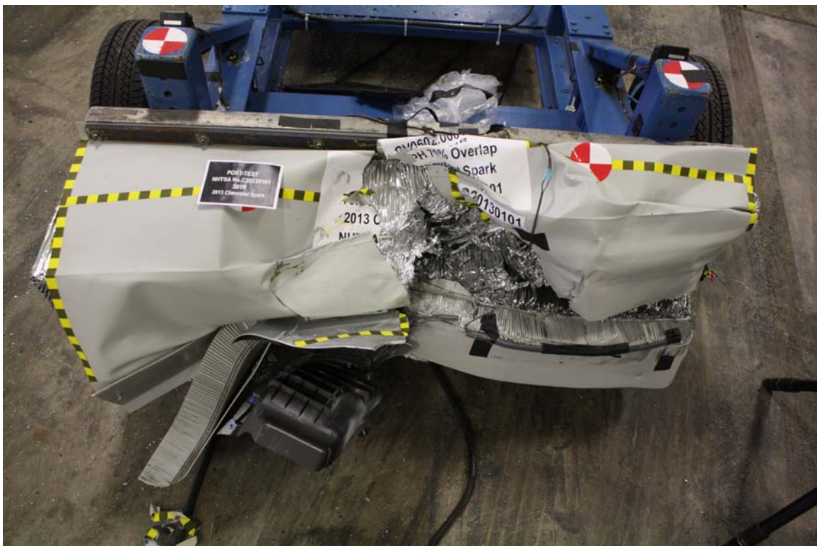
Figure A-26: Post-Test MDB Top View
