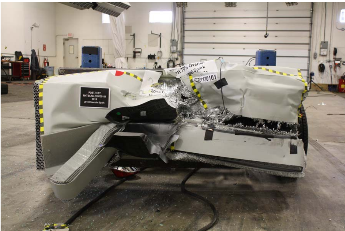
Figure A-20: Post-Test MDB Front View
