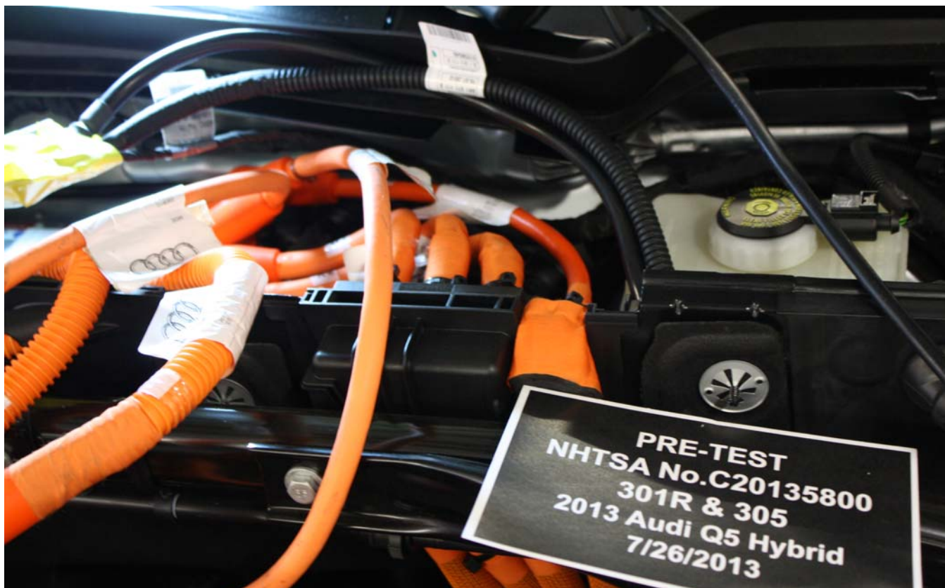
Figure A-63: Pre-Impact Close-Up View of High Voltage Leads Attached
