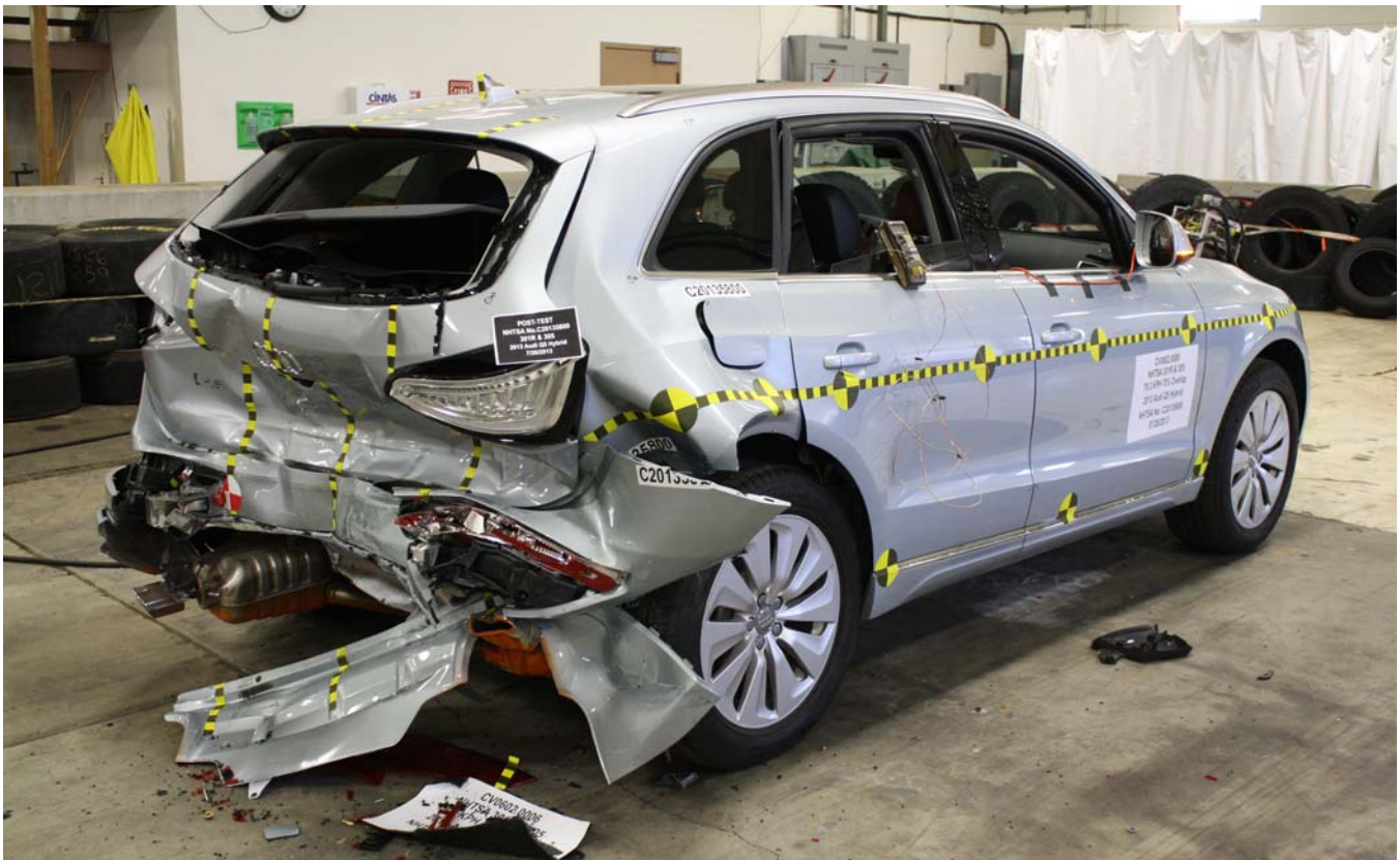
Figure A-18: Post-Test Right Rear 3/4 View
