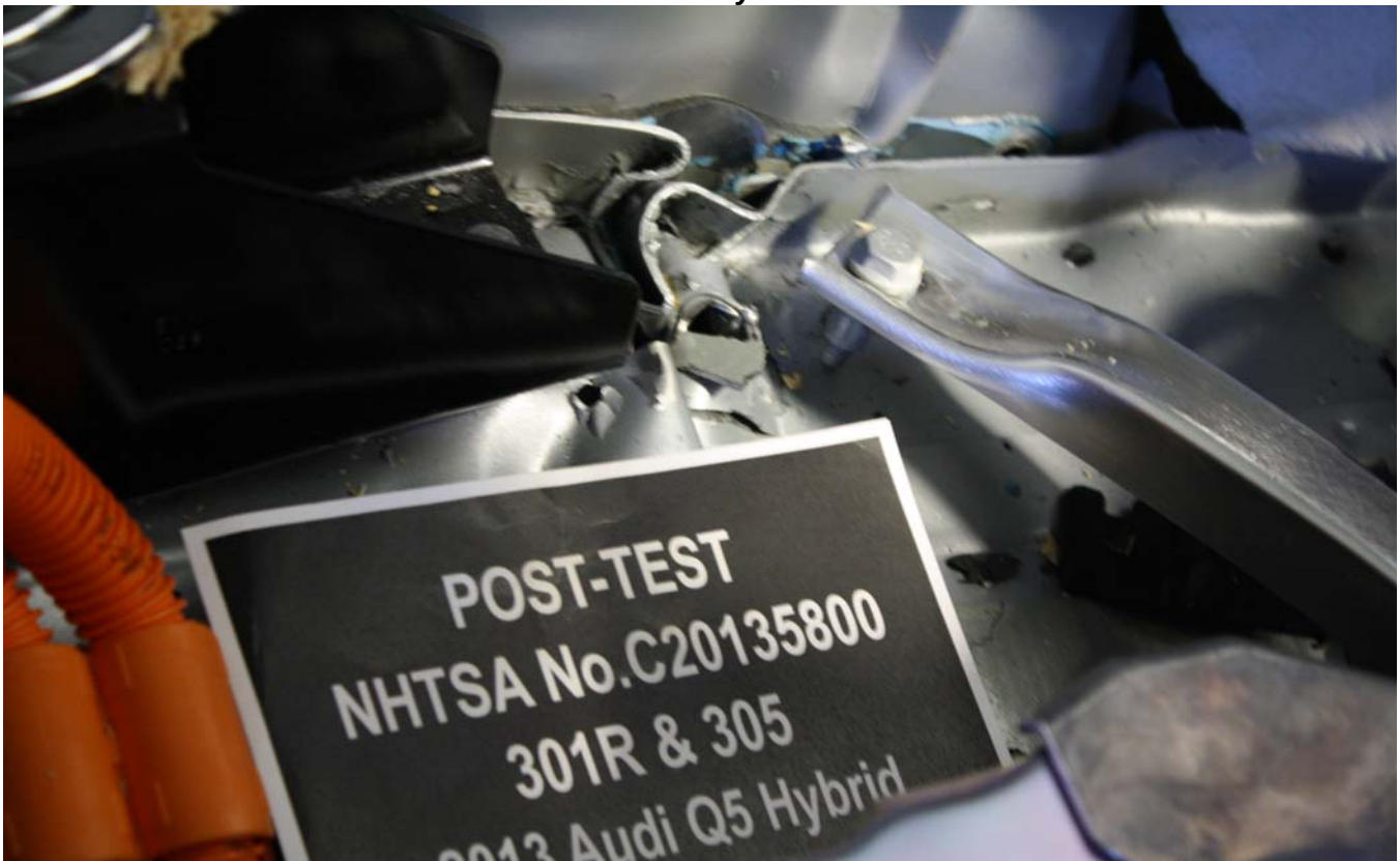
Figure A-78: Post-Impact Propulsion Battery System Mounting and/or Intrusion Failure(s)
