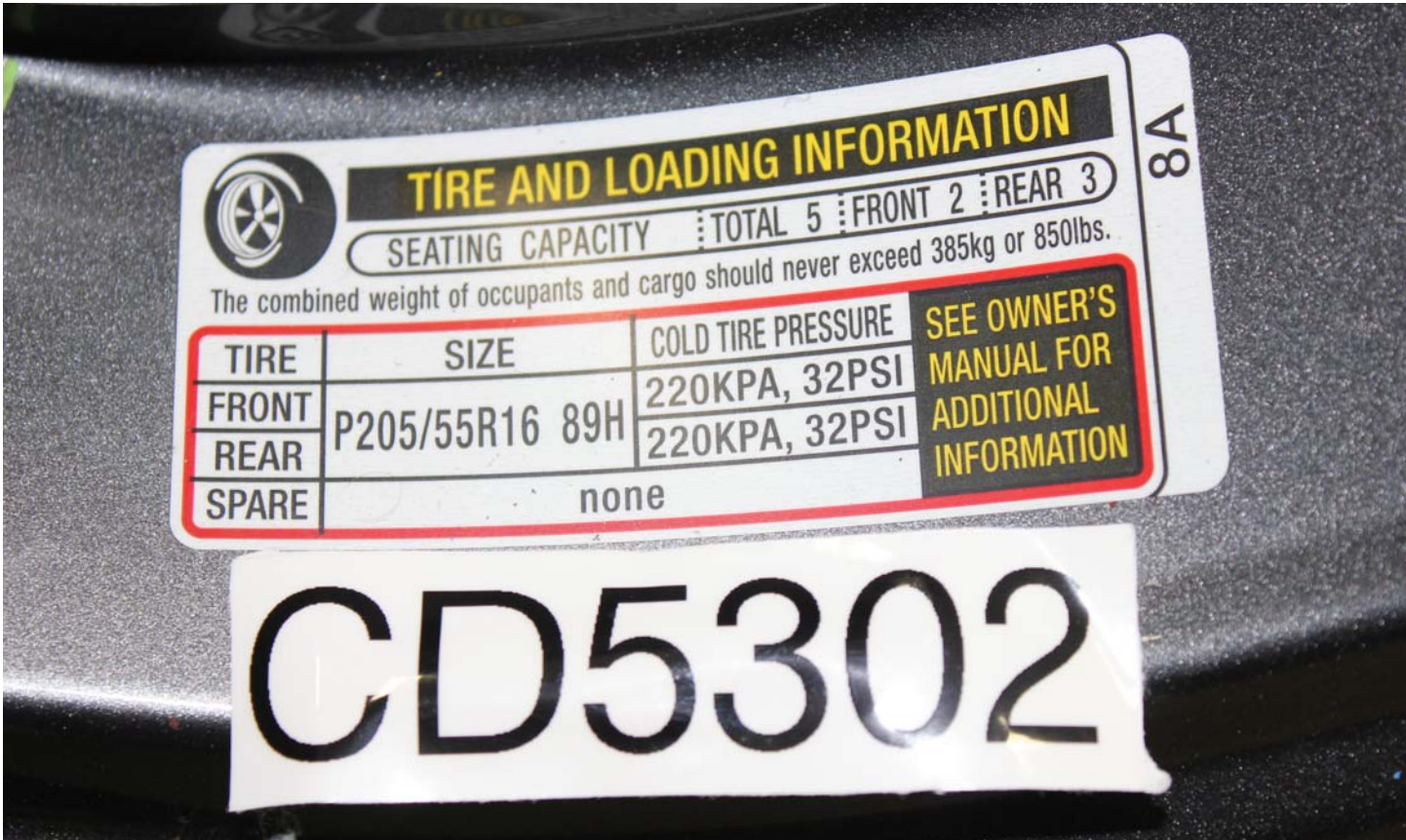
Vehicle's Tire Information Placard or Label
