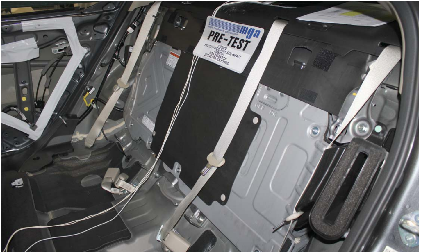
Pre-Impact View of Propulsion Battery With Cover
