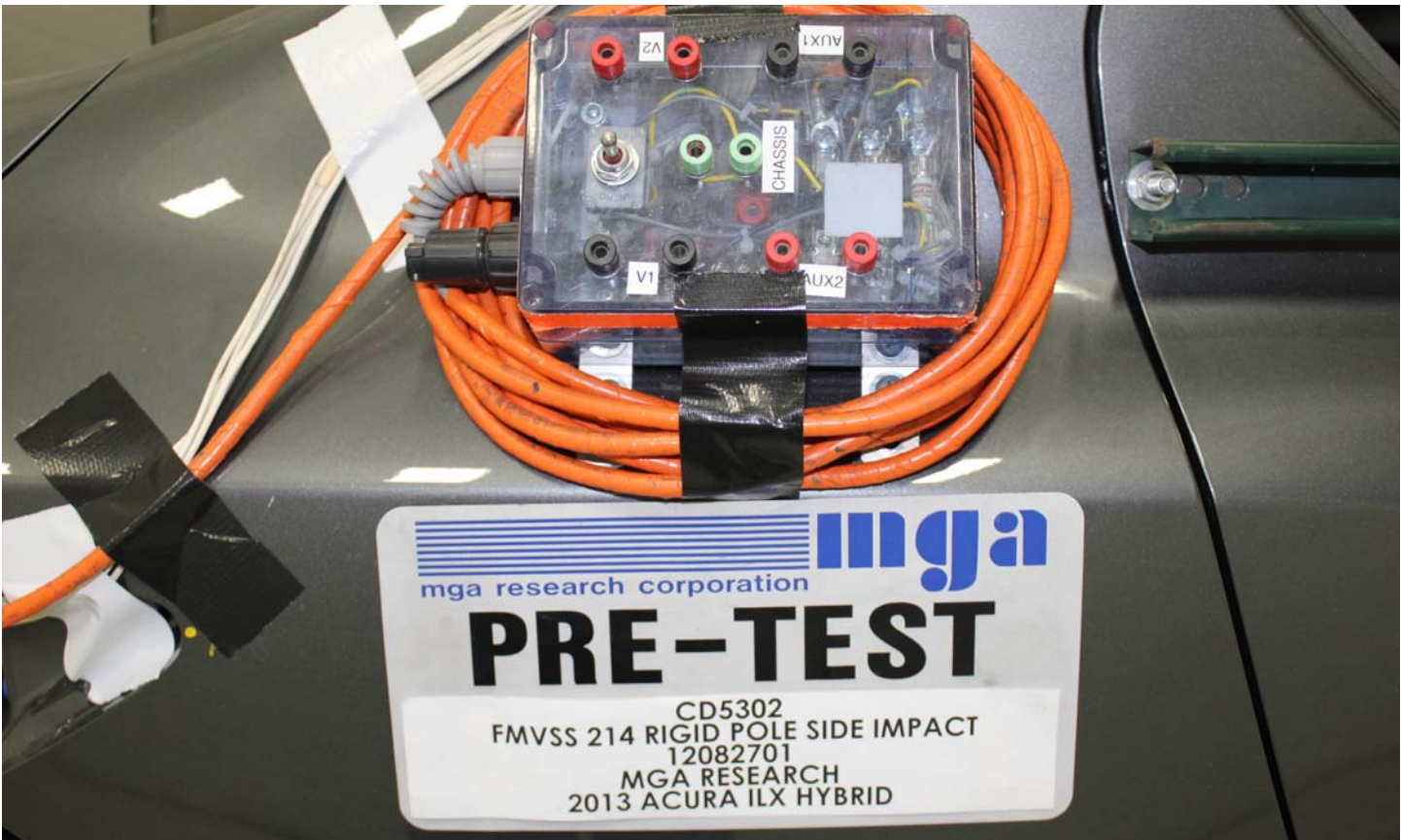
Pre-Impact View of Installed Impact Interface Port
