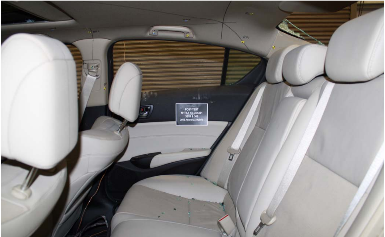
Figure A-77: Post-Impact View of the Vehicle Passenger Compartment Adjacent to Propulsion Battery
