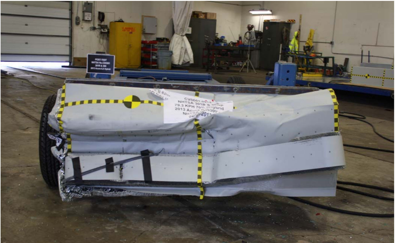
Figure A-22: Post-Test MDB Front View
