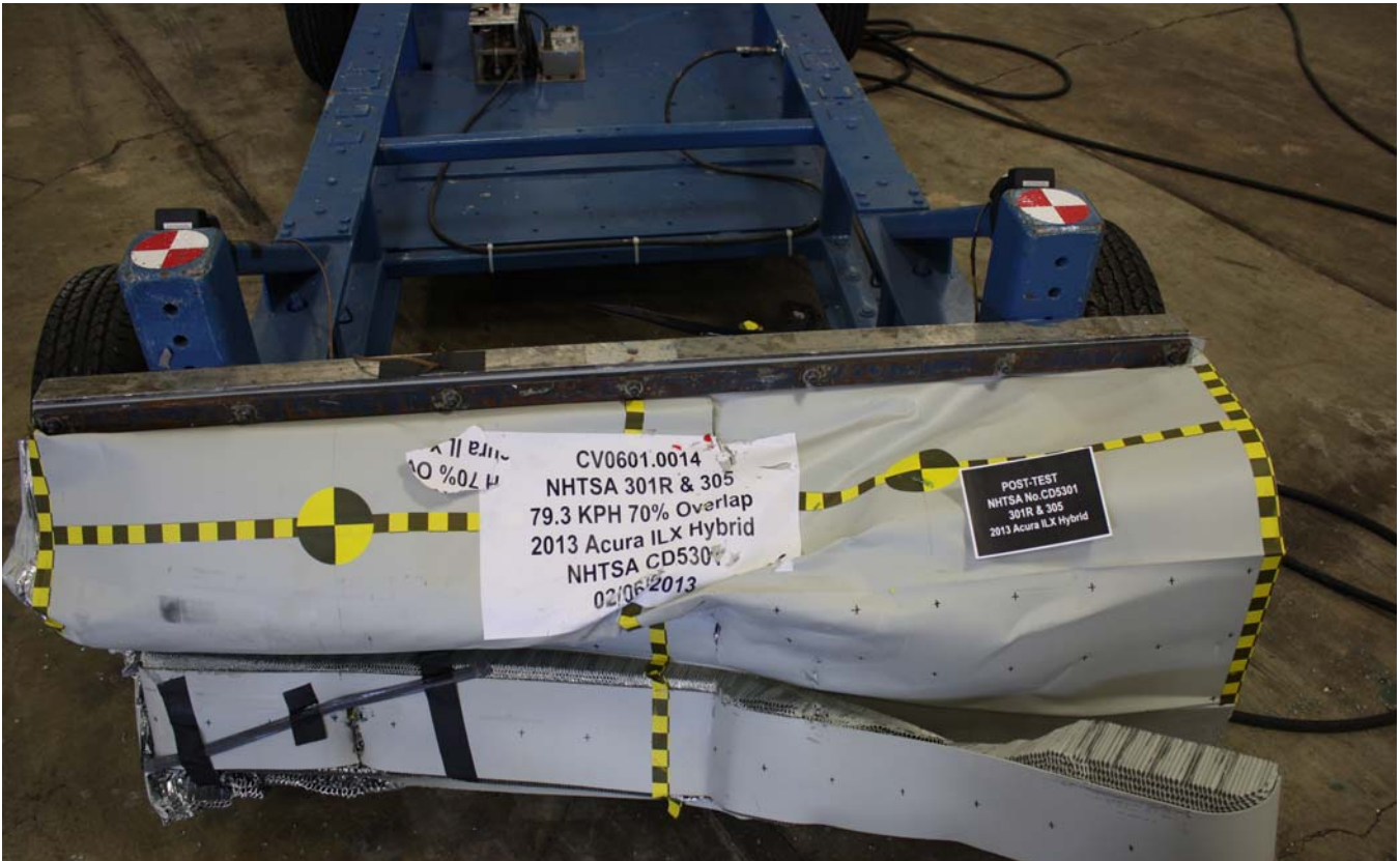
Figure A-28: Post-Test MDB Top View
