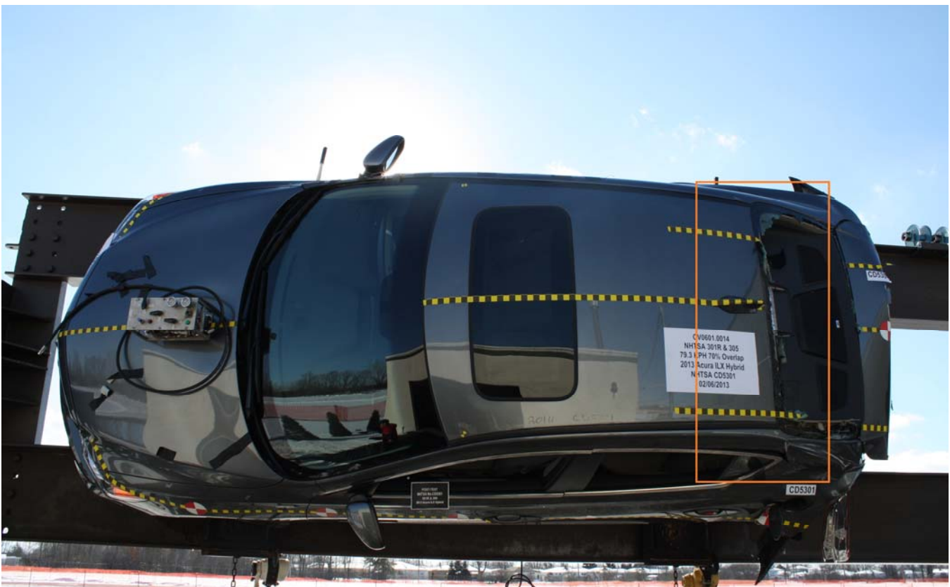
Figure A-72: FMVSS No. 305 Static Rollover at 90° Highlighting Propulsion Battery Location
