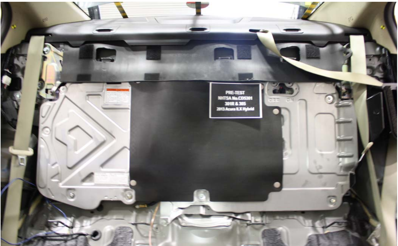
Figure A-52: Pre-Impact View of Battery Box(s) or Container(s) Which Holds Individual Battery Modules
