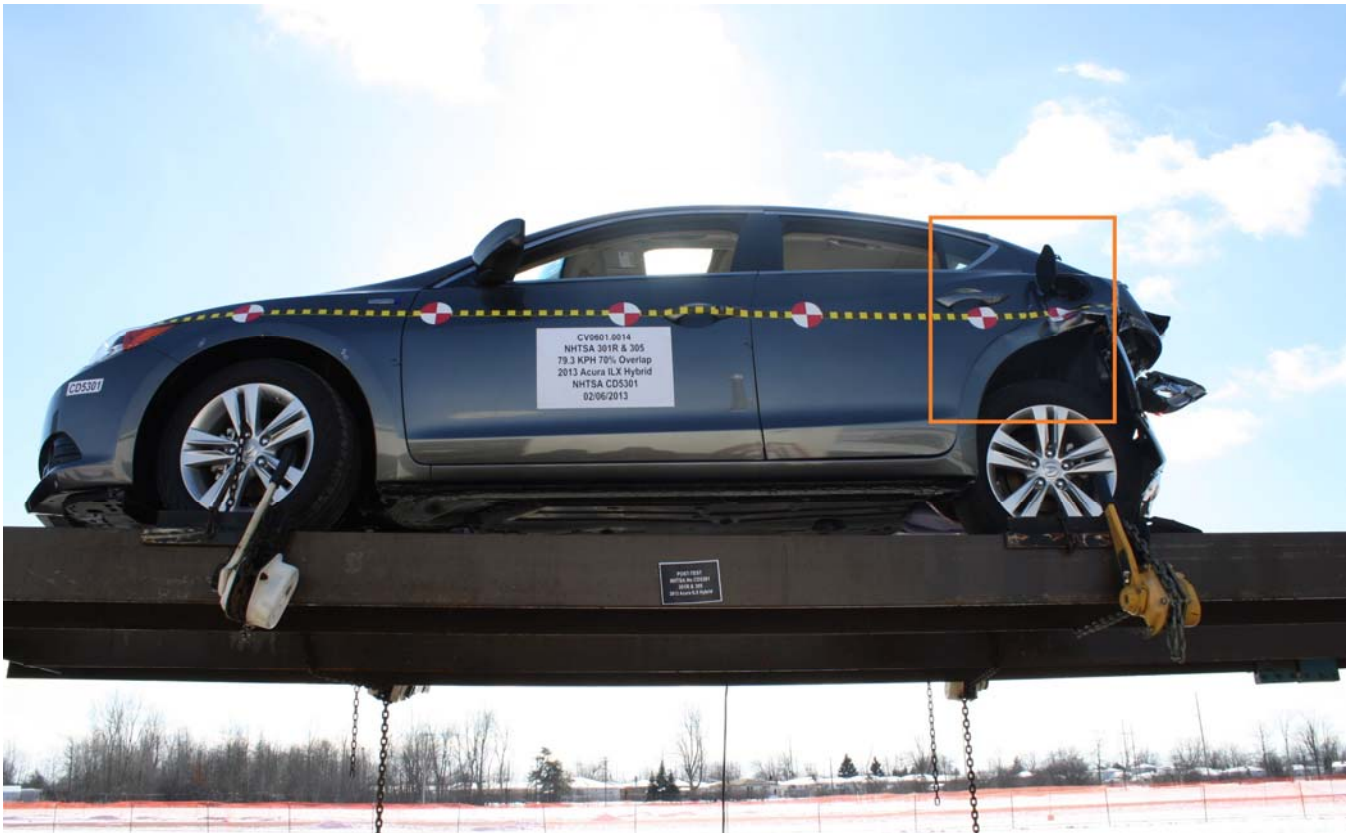
Figure A-75: FMVSS No. 305 Static Rollover at 360° Highlighting Propulsion Battery Location
