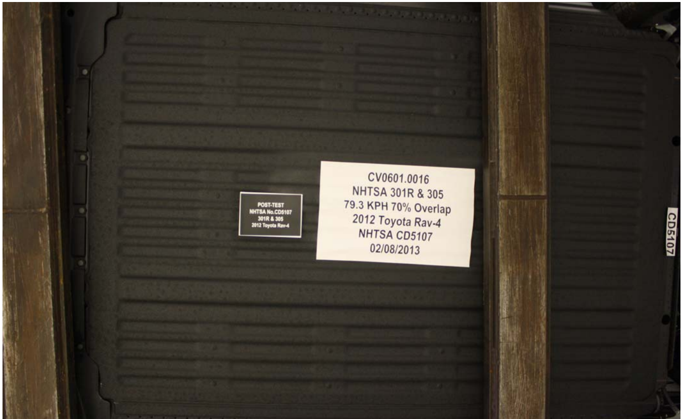
Figure A-53: Post-Impact View of Battery Box(s) or Container(s) Which Holds Individual Battery Modules
