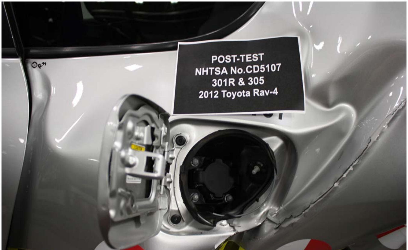
Figure A-38: Post-Test Fuel Filler Cap View
