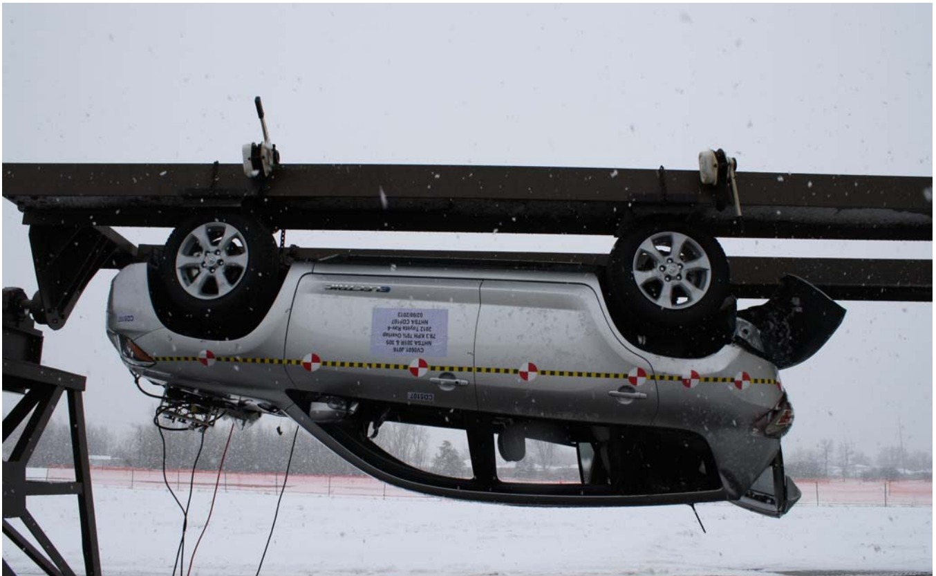
Figure A-69: FMVSS No. 301 Static Rollover 180° View
