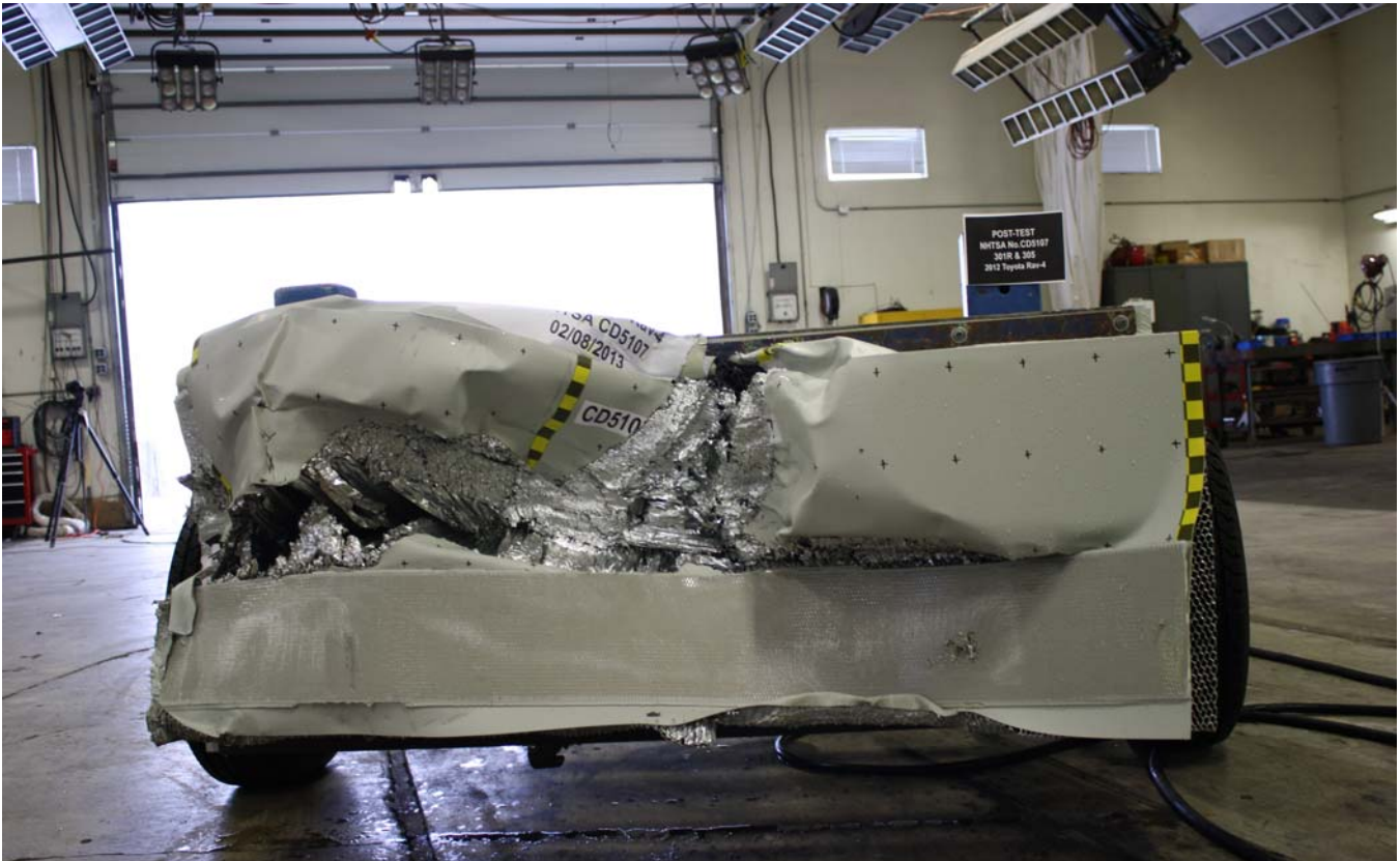
Figure A-22: Post-Test MDB Front View
