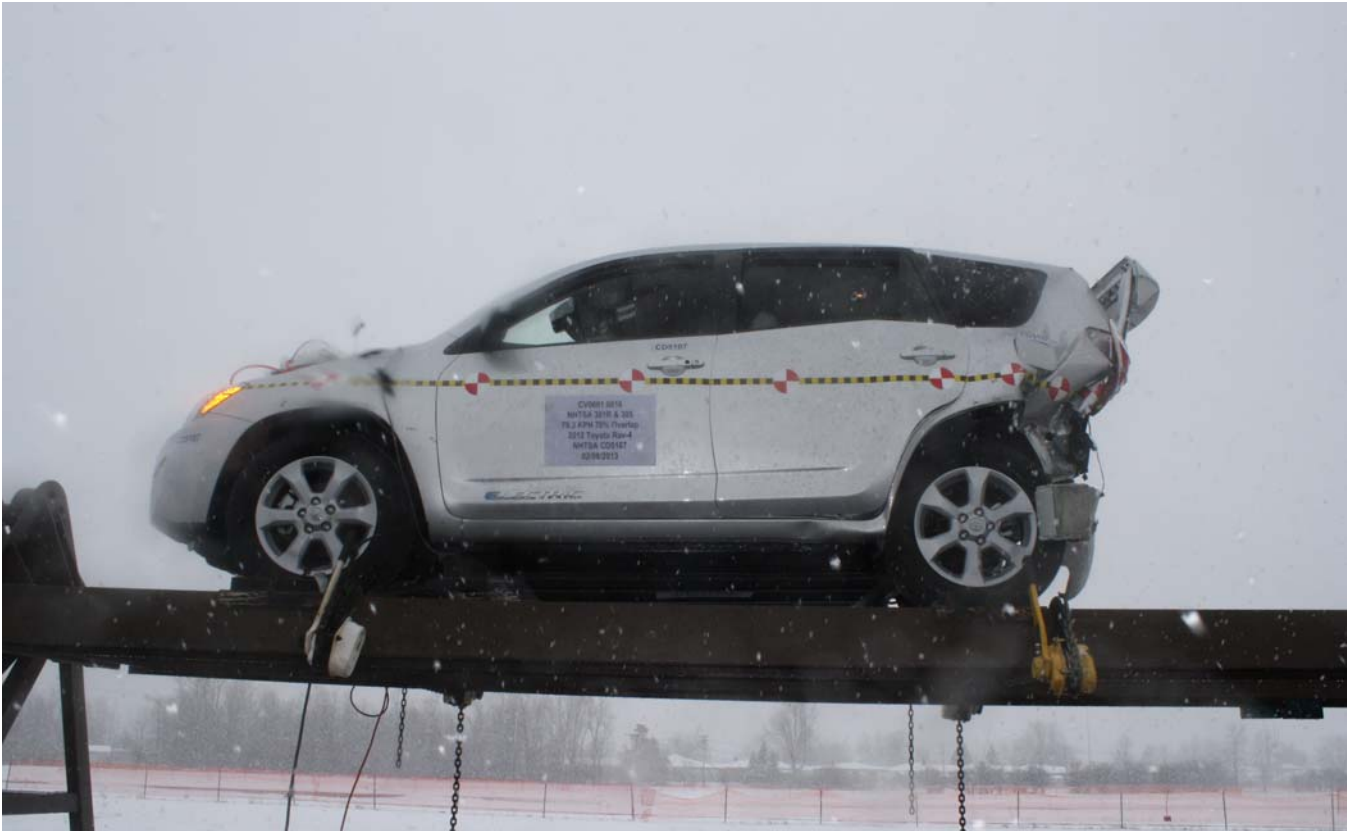
Figure A-71: FMVSS No. 301 Static Rollover 360° View
