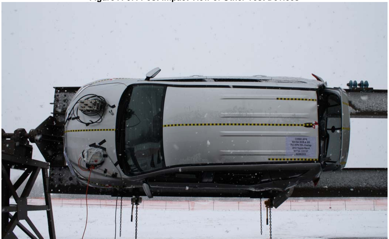
Figure A-68: FMVSS No. 301 Static Rollover 90° View
