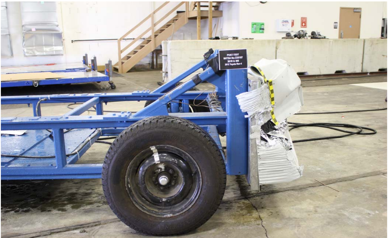
Figure A-26: Post-Test MDB Right Side View
