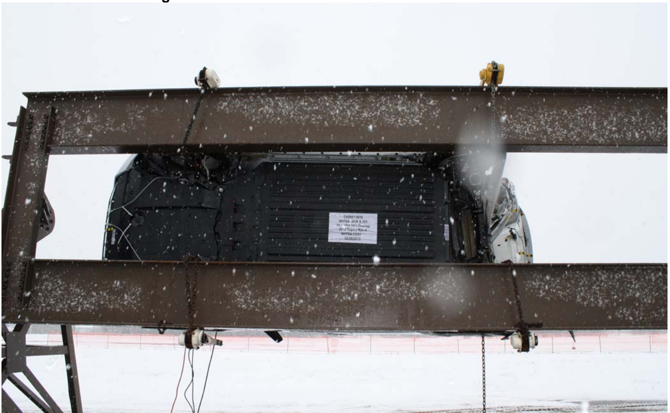
Figure A-70: FMVSS No. 301 Static Rollover 270° View
