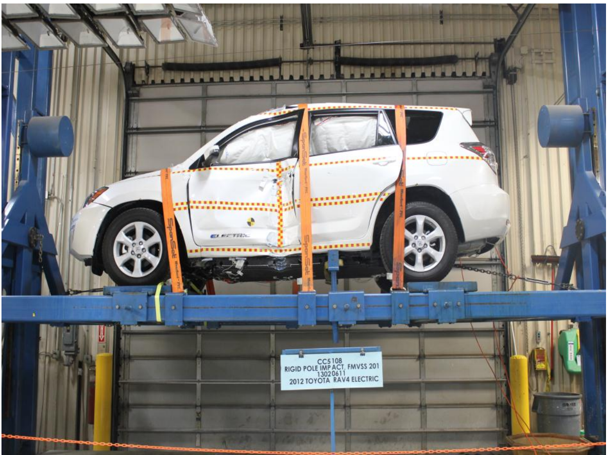
FMVSS No. 305 Static Rollover at 360°
