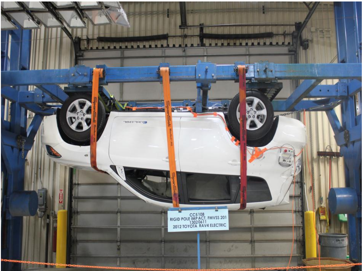
FMVSS No. 305 Static Rollover at 180°
