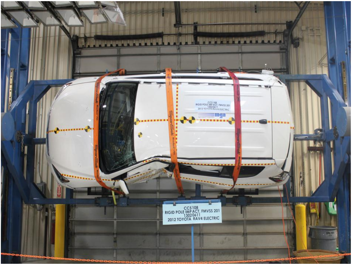
FMVSS No. 305 Static Rollover at 90°
