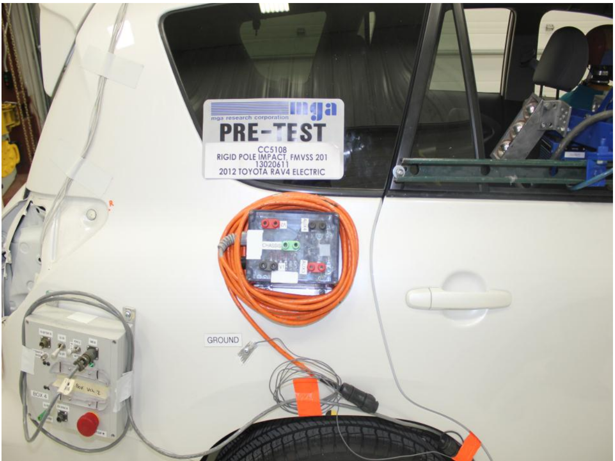
Pre-Impact View of Installed Impact Interface Port
