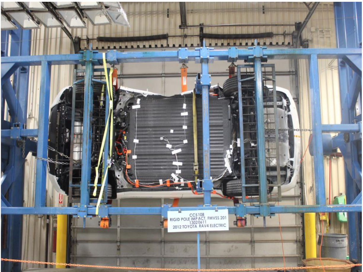
FMVSS No. 305 Static Rollover at 270°
