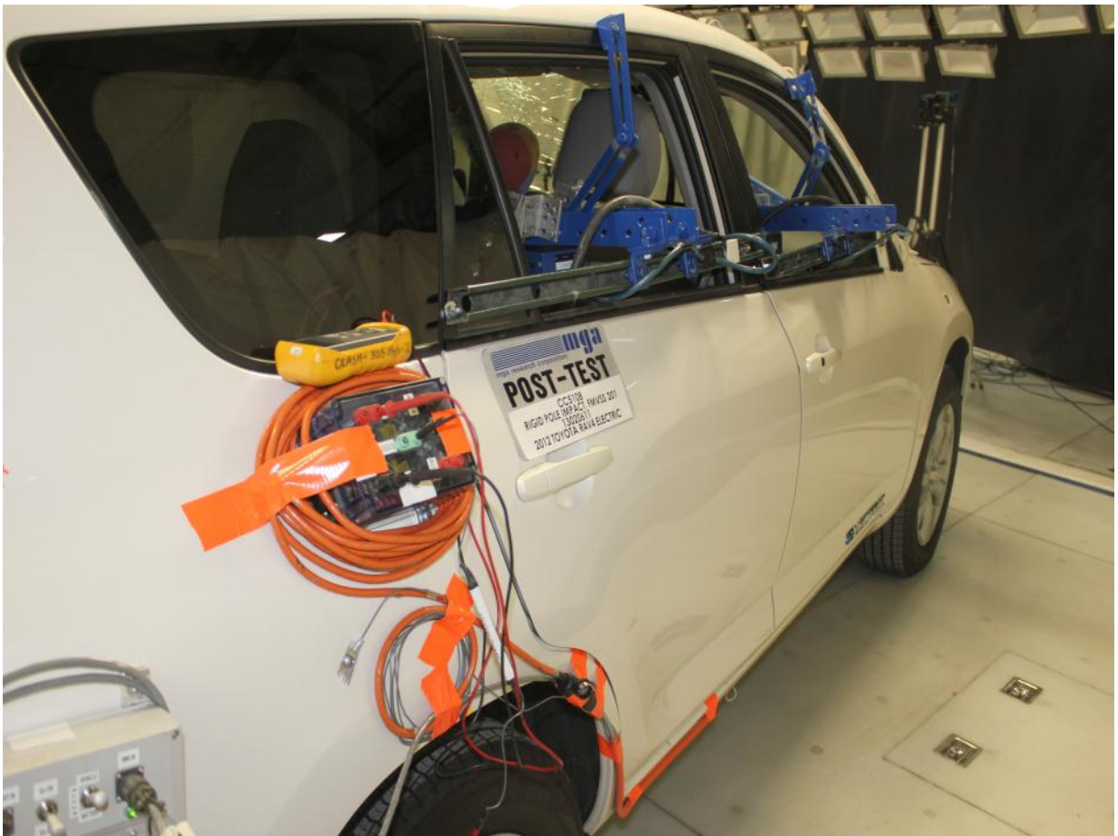
Post-Impact View of Installed Impact Interface Port
