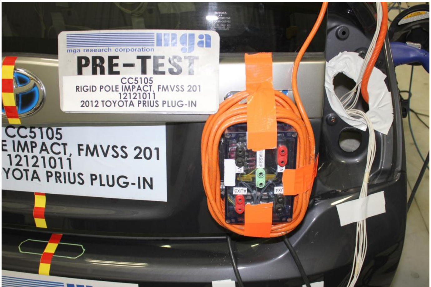
Pre-Impact View of Installed Impact Interface Port
