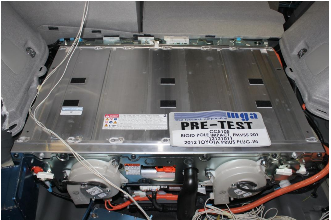
Pre-Impact View of Propulsion Battery
