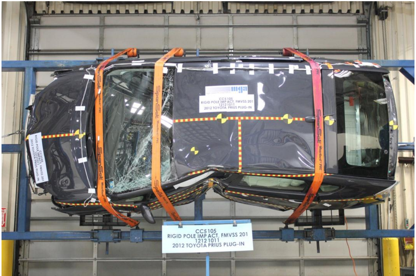
FMVSS No. 305 Static Rollover at 90°
