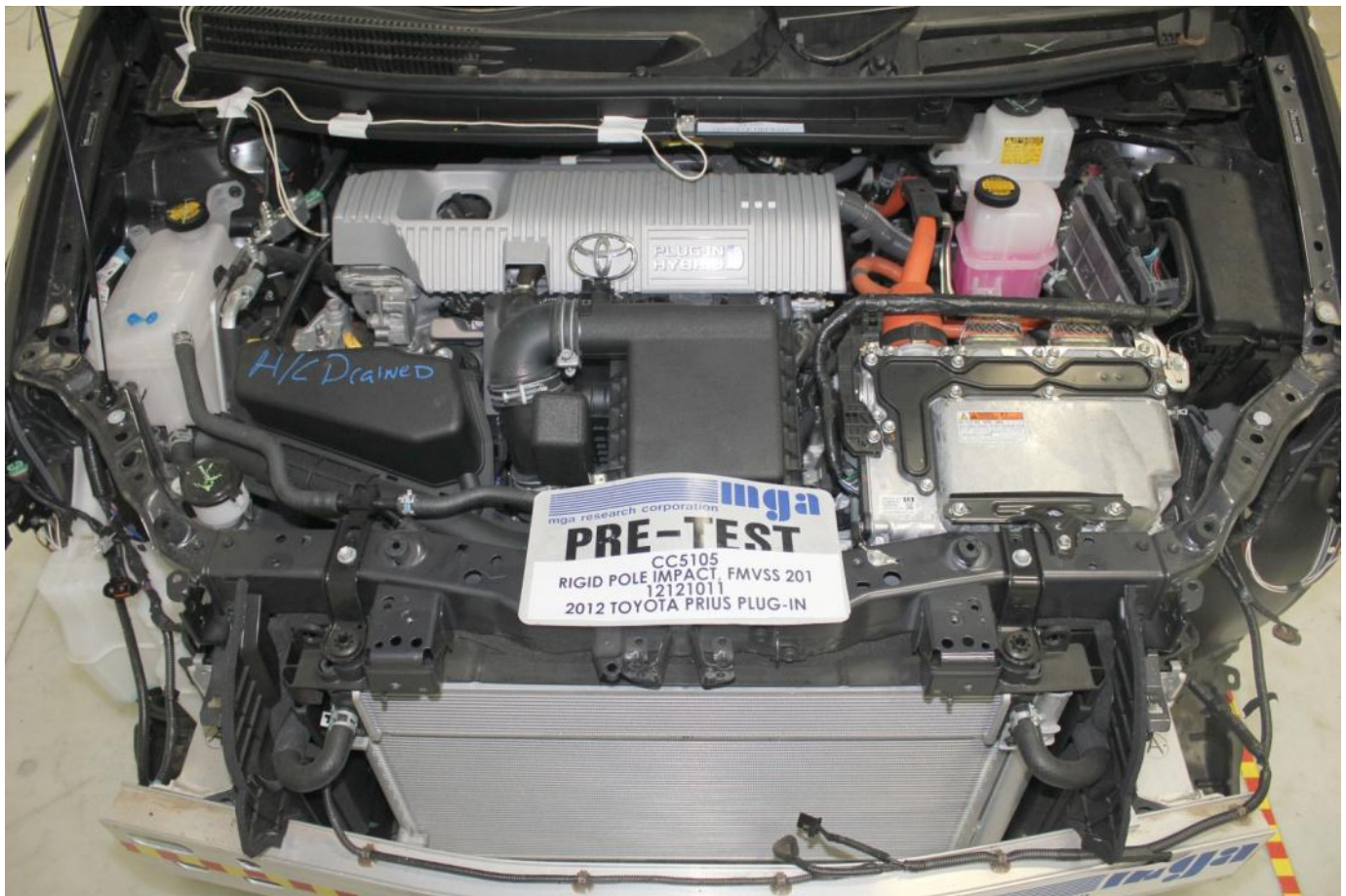
Pre-Impact View of Electric Propulsion Drive
