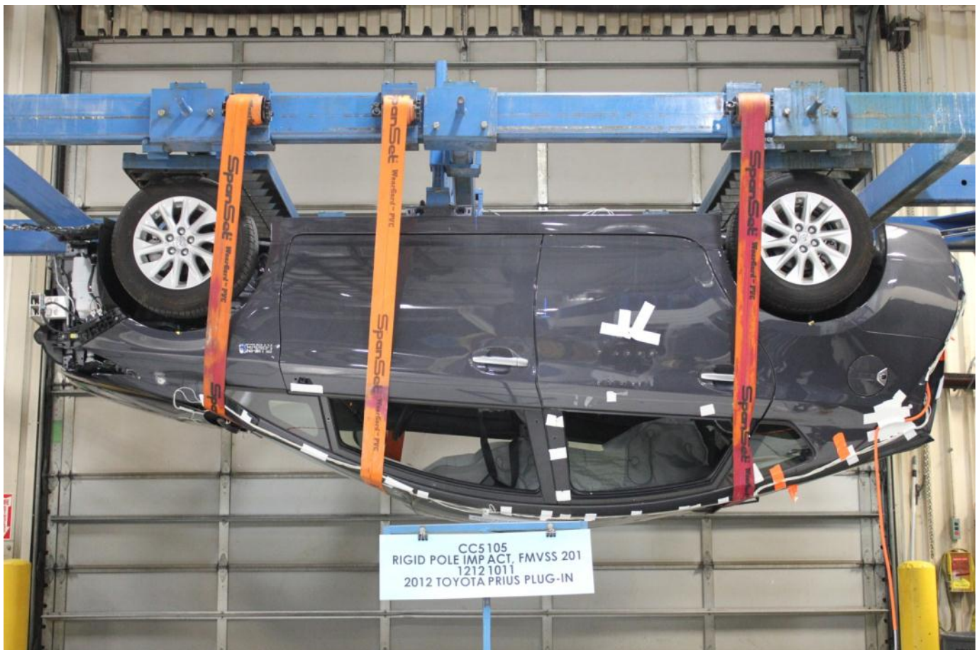
FMVSS No. 305 Static Rollover at 180°
