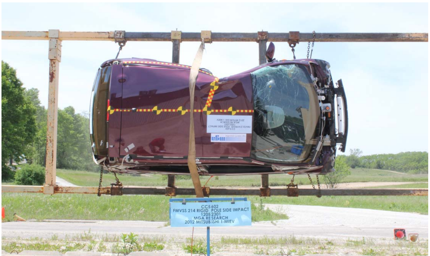
No. 012 FMVSS No. 305 Static Rollover at 90°
