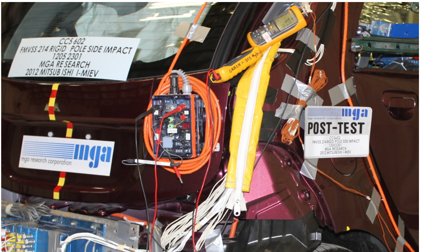
No. 011 Post-Impact View of Installed Impact Interface Port
