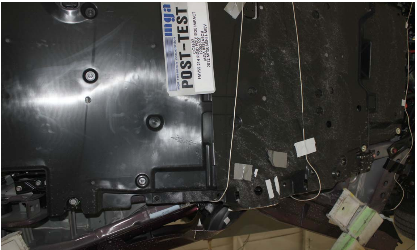
No. 017 Post-Impact View of Battery Module Movement or Retention Loss
