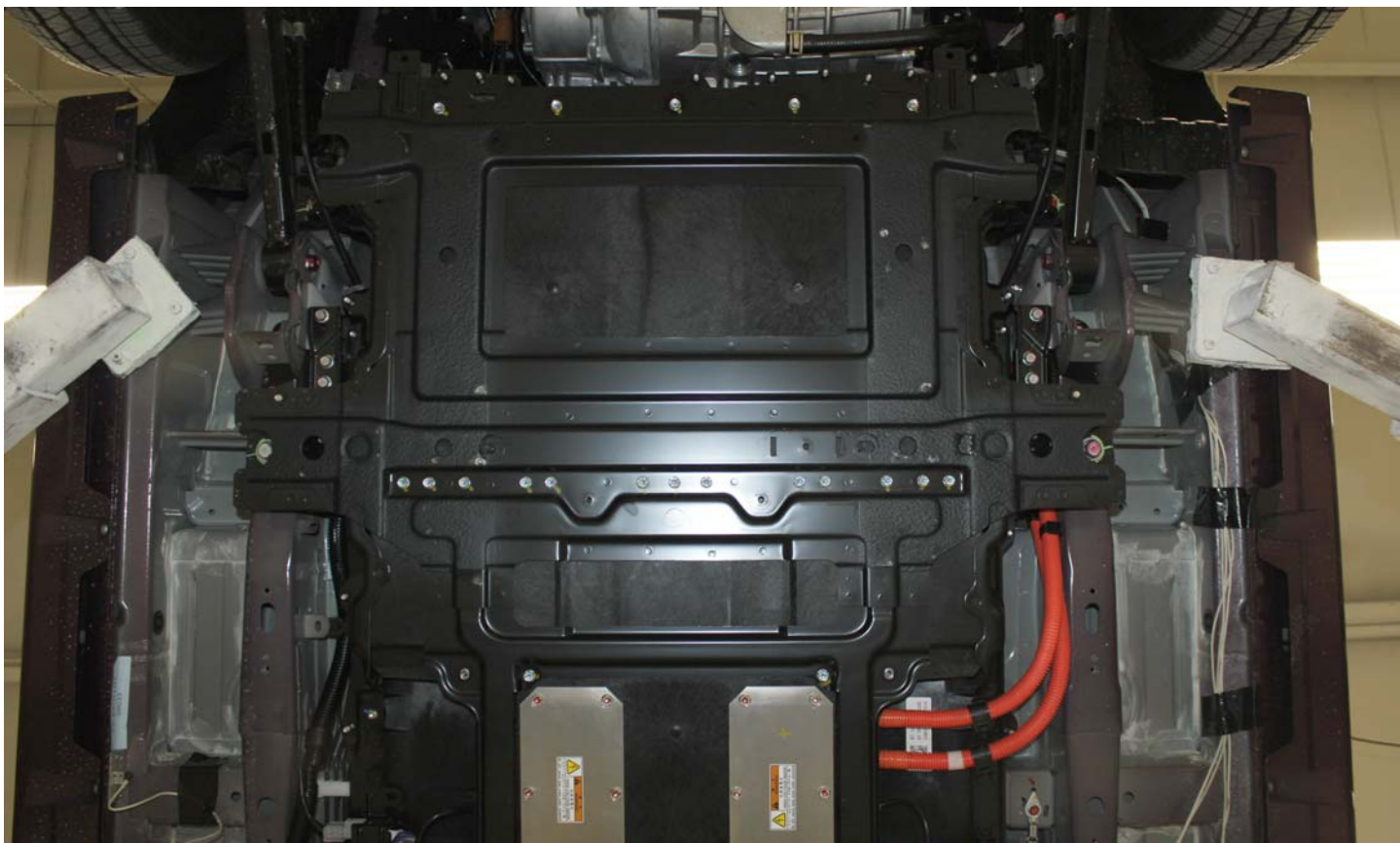
No. 003 Pre-Impact Rear View of Propulsion Battery
