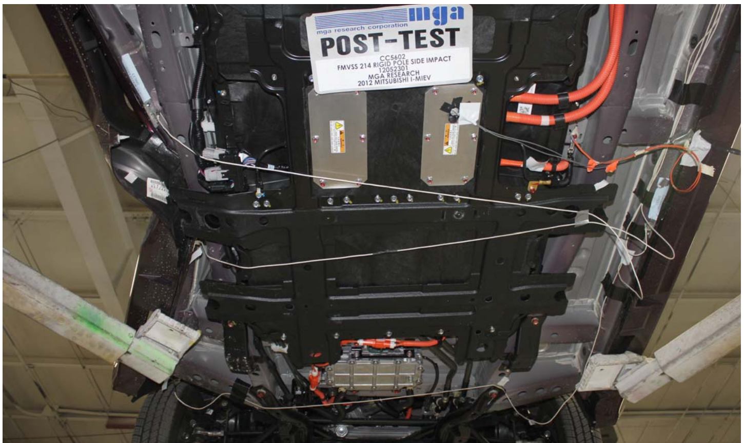
No. 016 Post-Impact View of Battery Module Movement or Retention Loss
