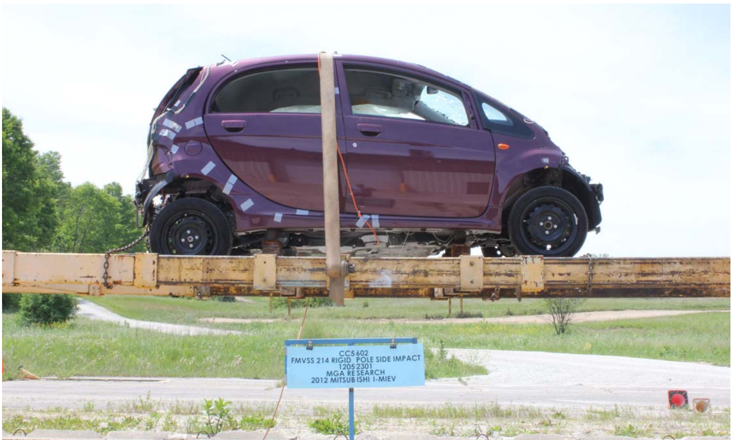
No. 015 FMVSS No. 305 Static Rollover at 360°
