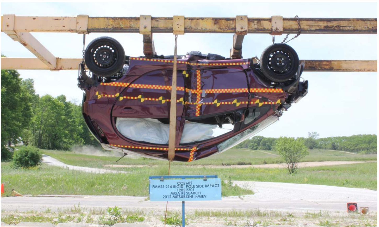
No. 013 FMVSS No. 305 Static Rollover at 180°
