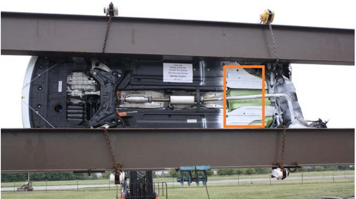
Figure A-74: FMVSS No. 305 Static Rollover at 270° Highlighting Propulsion Battery Location
