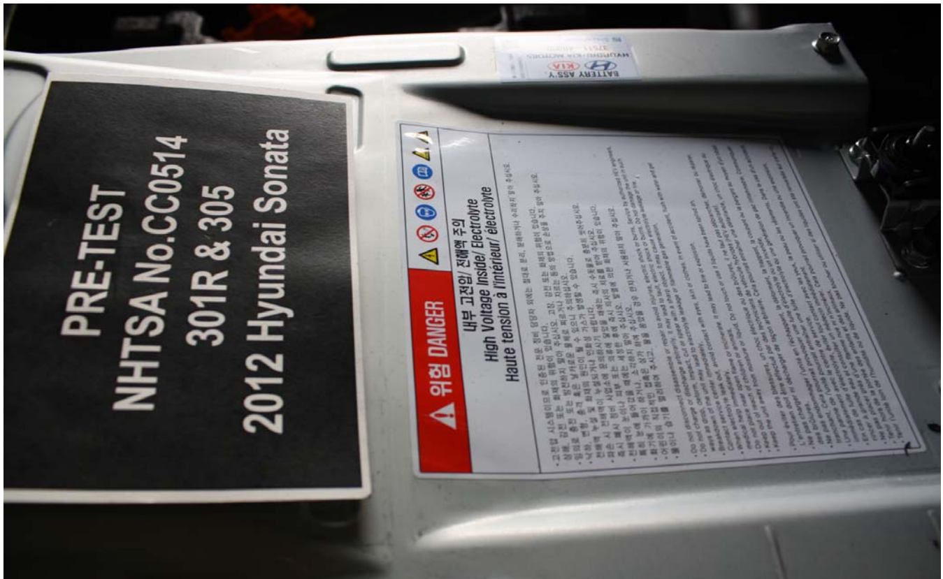
Figure A-42: Power Inverter Warning Label
