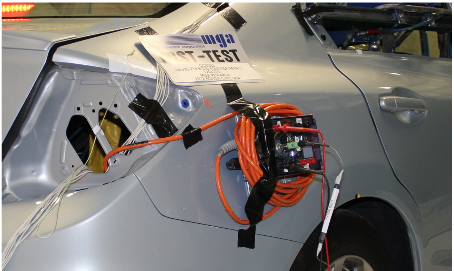
Post-Impact View of Installed Impact Interface Port
