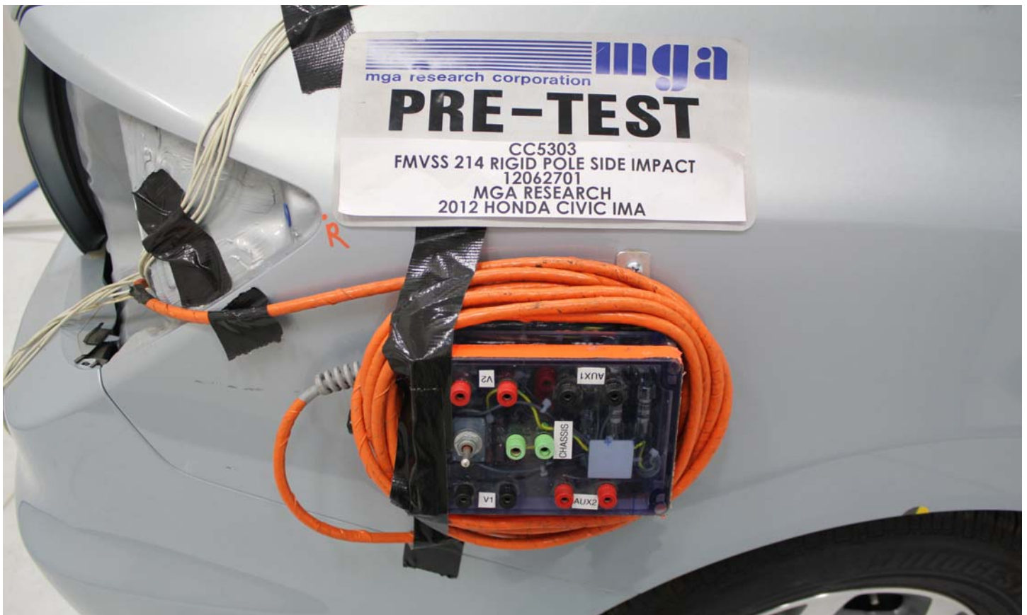
Pre-Impact View of Installed Impact Interface Port
