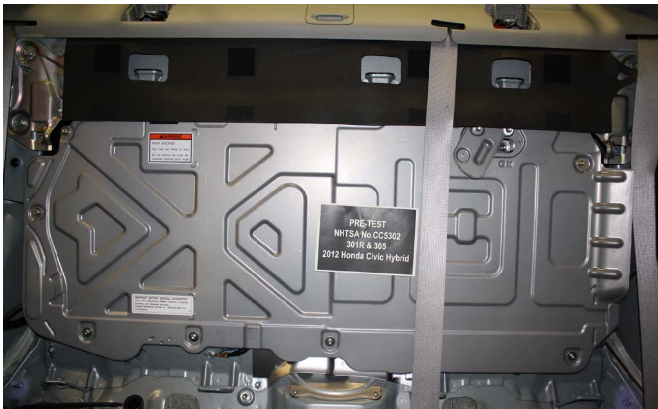
Figure A-48: Manual High Voltage Service Disconnect Removed (Location where removed)
