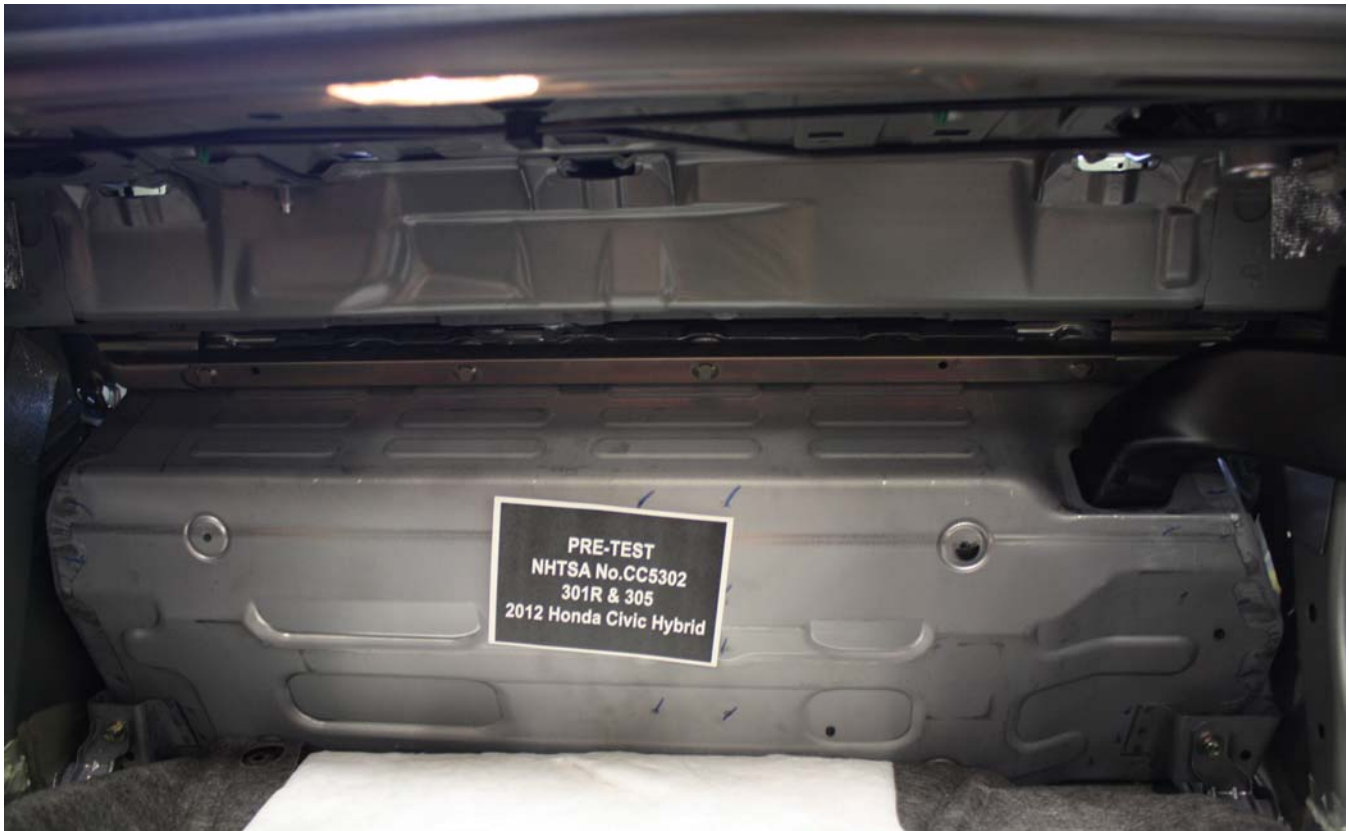
Figure A-49: Pre-Impact View of Propulsion Battery
