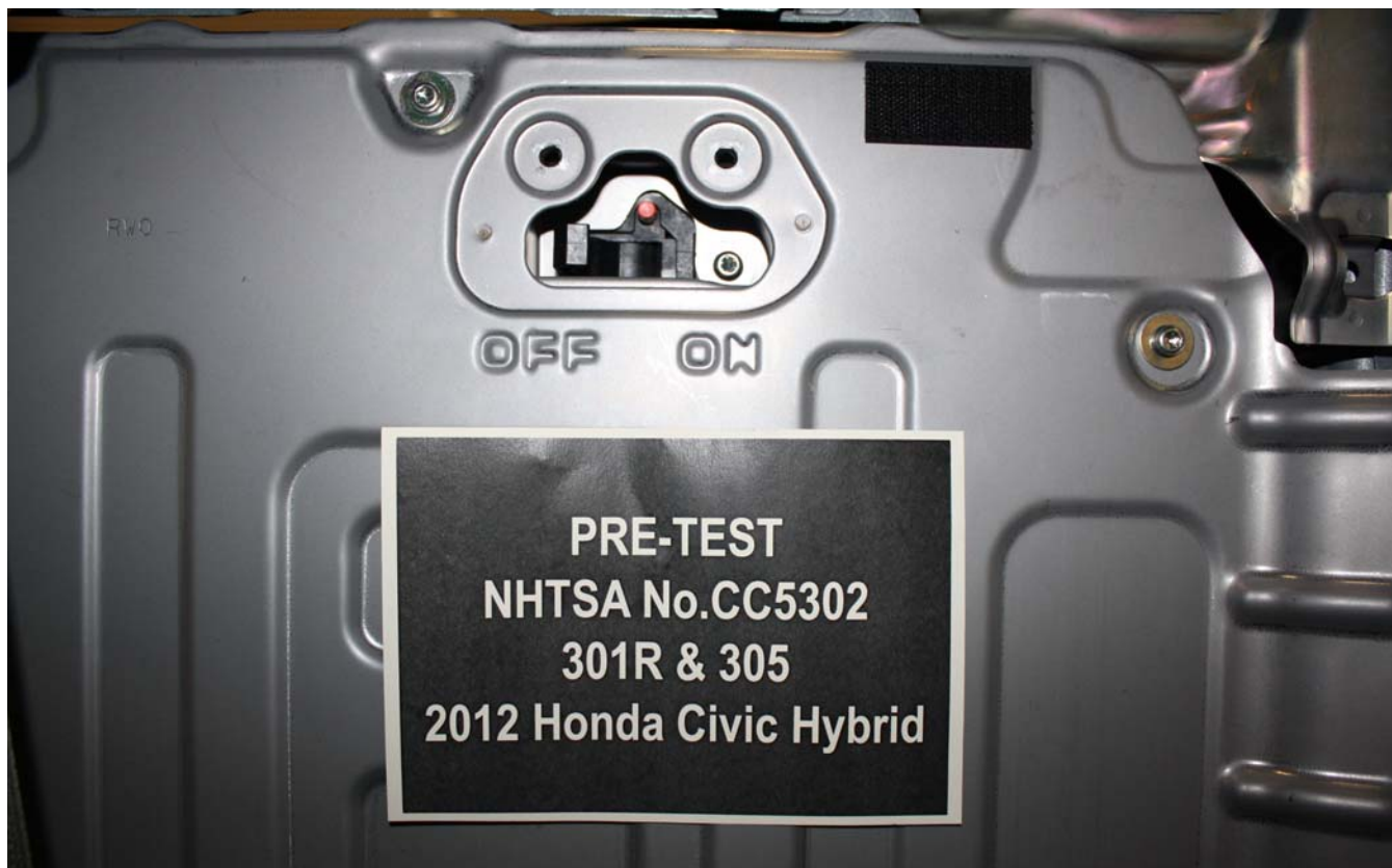
Figure A-47: Manual High Voltage Service Disconnect Removed (Plug)
