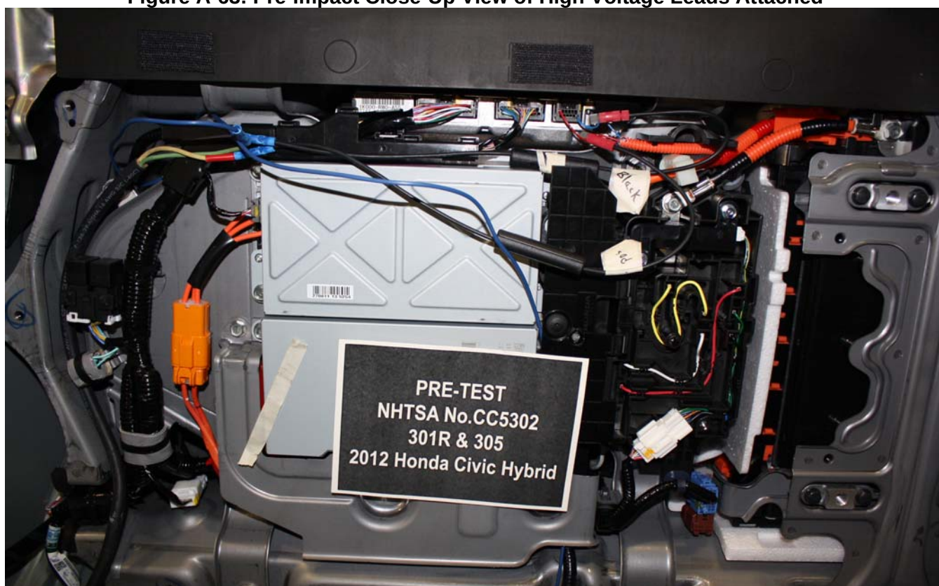
Figure A-64: Pre-Impact View of Installed Test Interface Port
