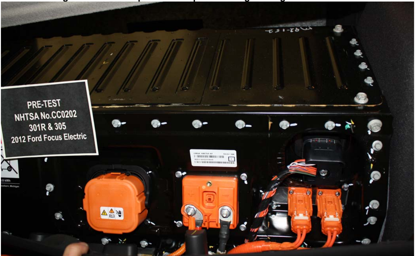
Figure A-64: Pre-Impact View of Installed Test Interface Port
