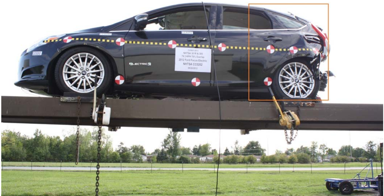
Figure A-75: FMVSS No. 305 Static Rollover at 360° Highlighting Propulsion Battery Location
