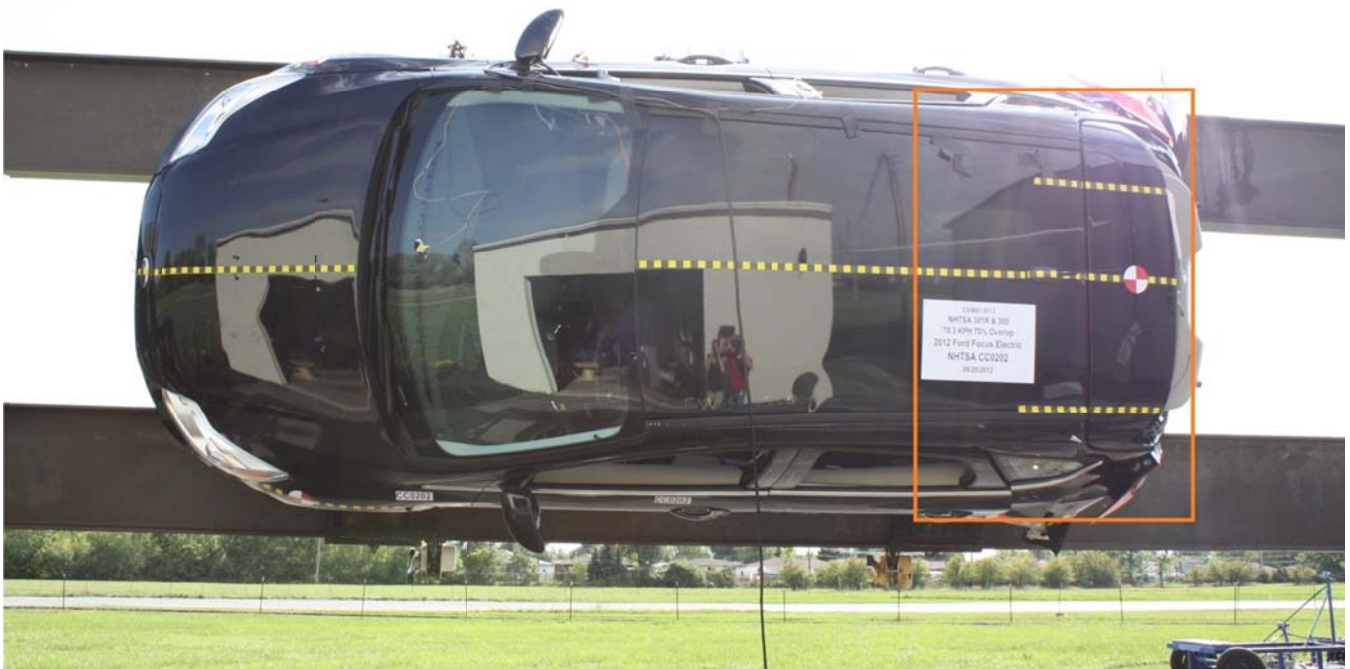
Figure A-74: FMVSS No. 305 Static Rollover at 270° Highlighting Propulsion Battery Location
