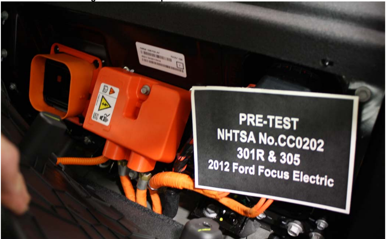
Figure A-62: Pre-Impact View of High Voltage Leads Attached
