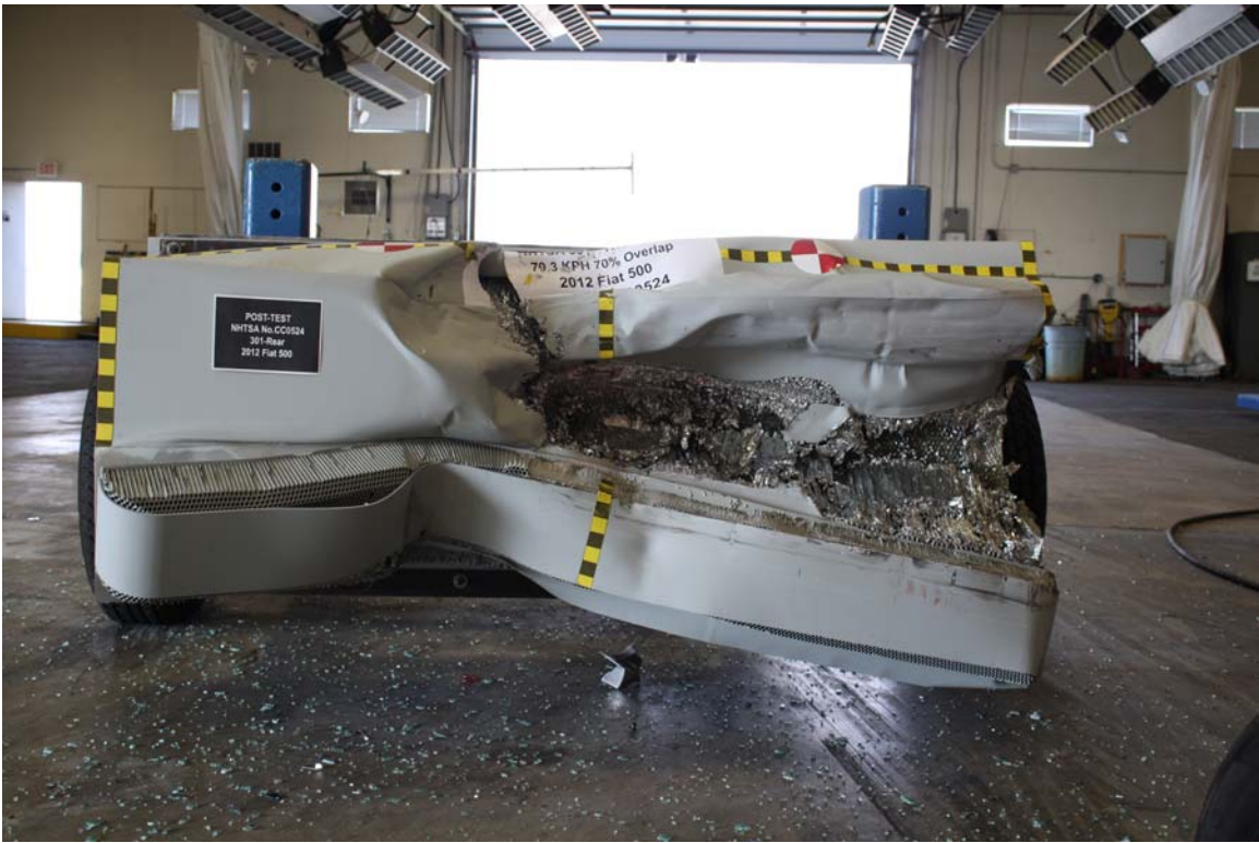
Figure A-21: Post-Test MDB Front View
