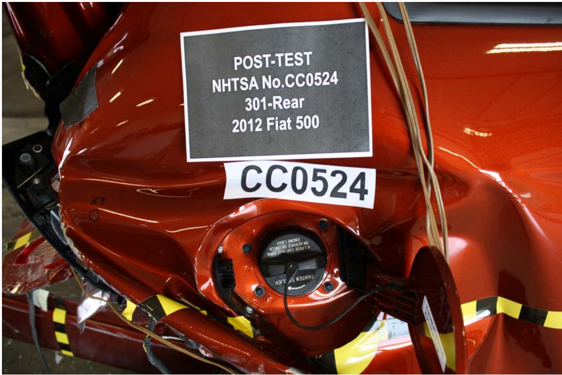
Figure A-37: Post-Test Fuel Filler Cap View
