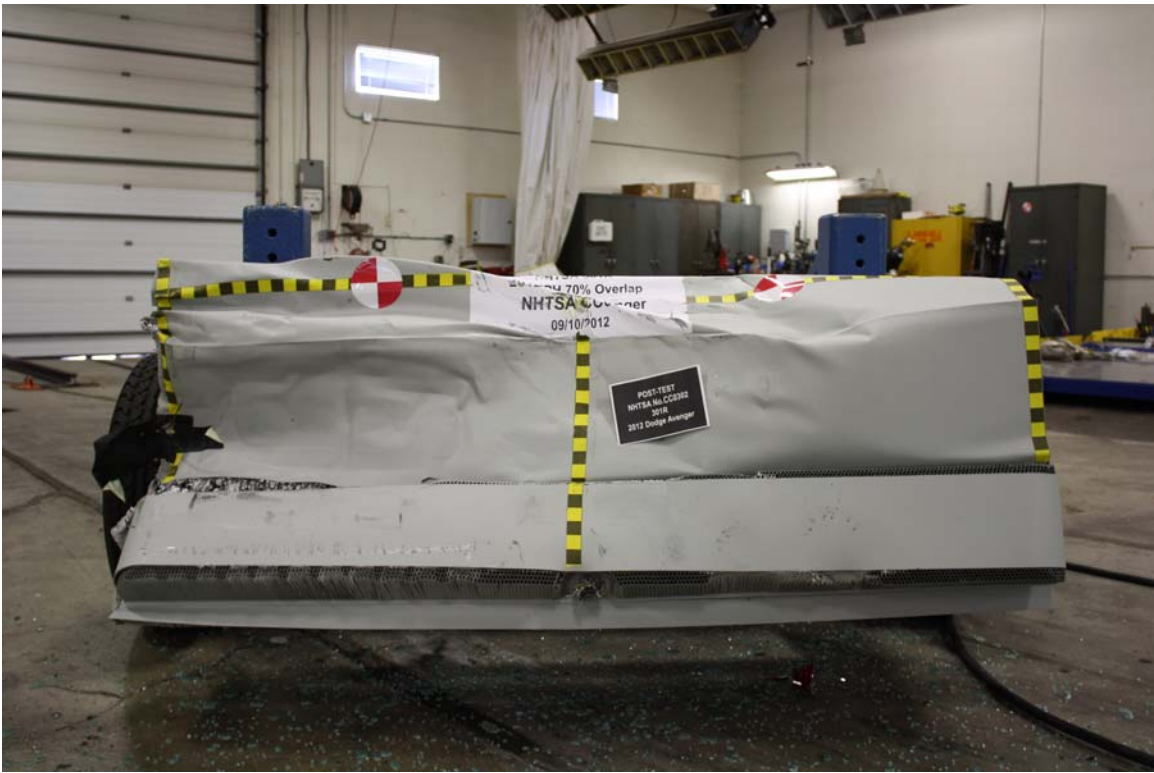
Figure A-21: Post-Test MDB Front View
