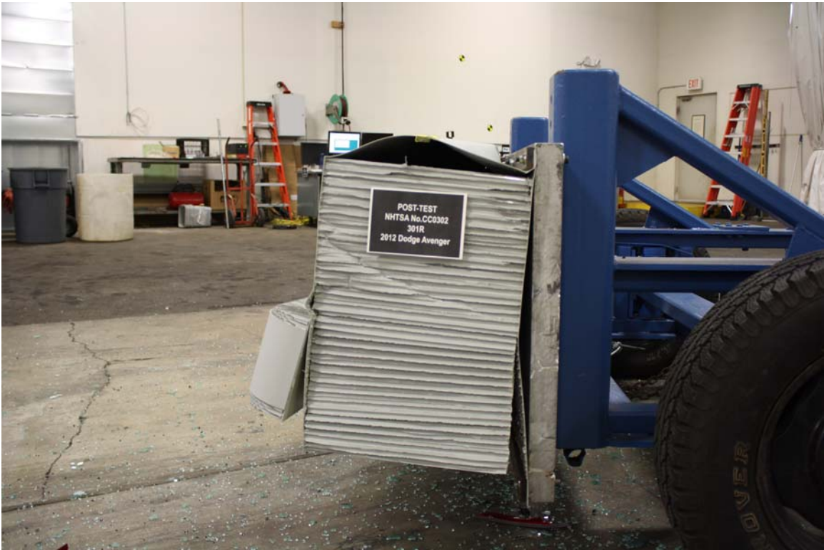
Figure A-23: Post-Test MDB Left Side View
