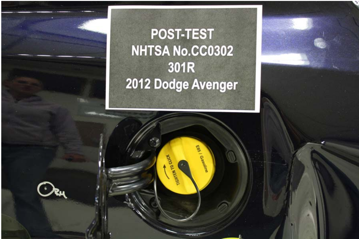
Figure A-37: Post-Test Fuel Filler Cap View
