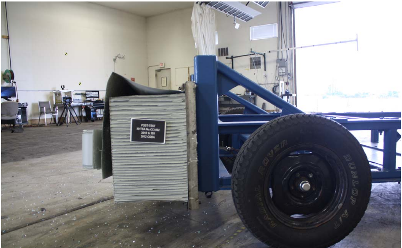
Figure A-24: Post-Test MDB Left Side View
