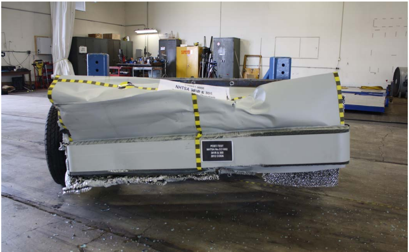
Figure A-22: Post-Test MDB Front View
