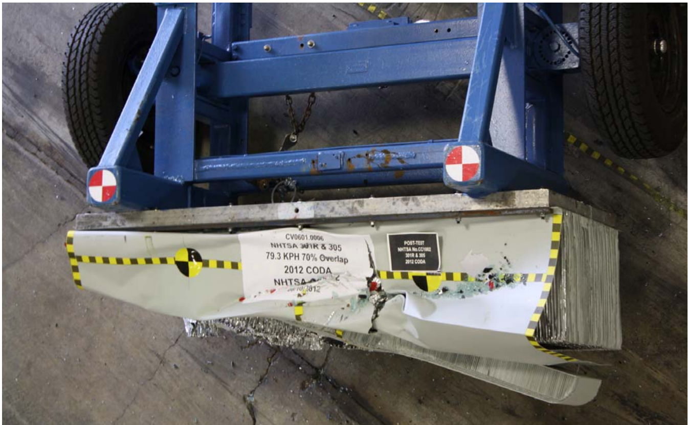
Figure A-28: Post-Test MDB Top View
