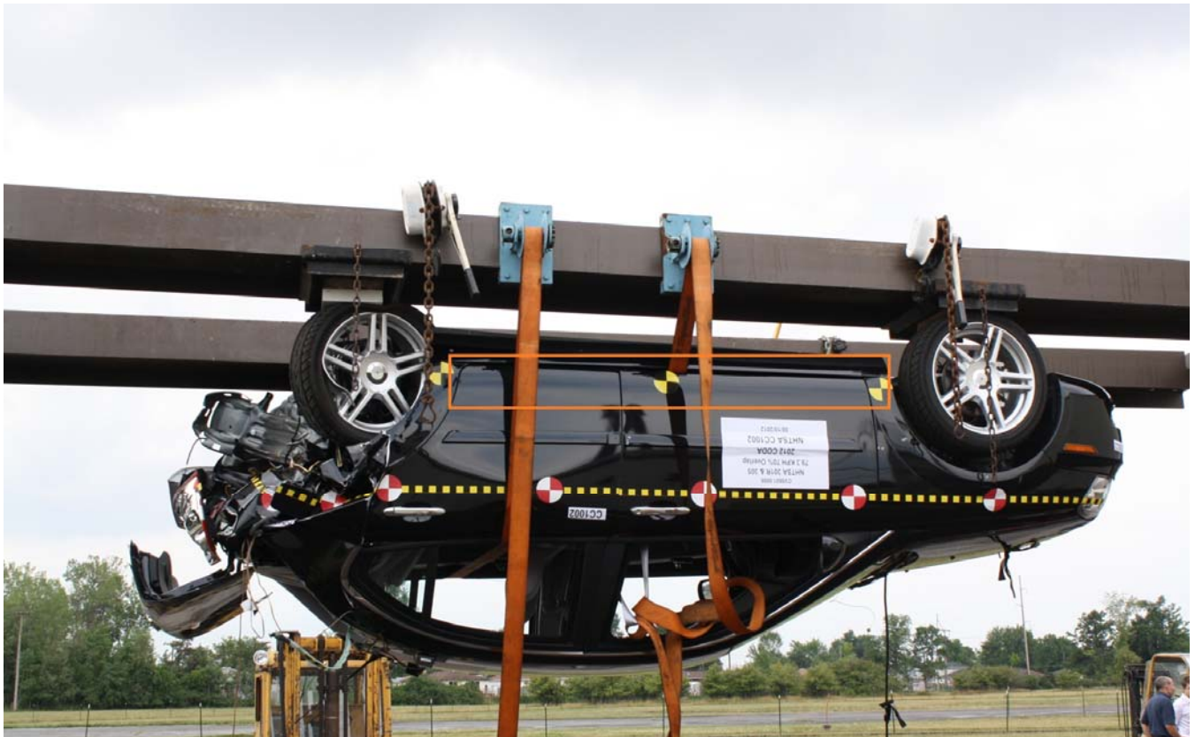
Figure A-73: FMVSS No. 305 Static Rollover at 180° Highlighting Propulsion Battery Location
