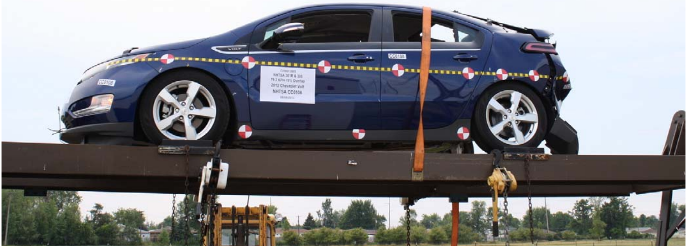
Figure A-75: FMVSS No. 305 Static Rollover at 360° Highlighting Propulsion Battery Location
