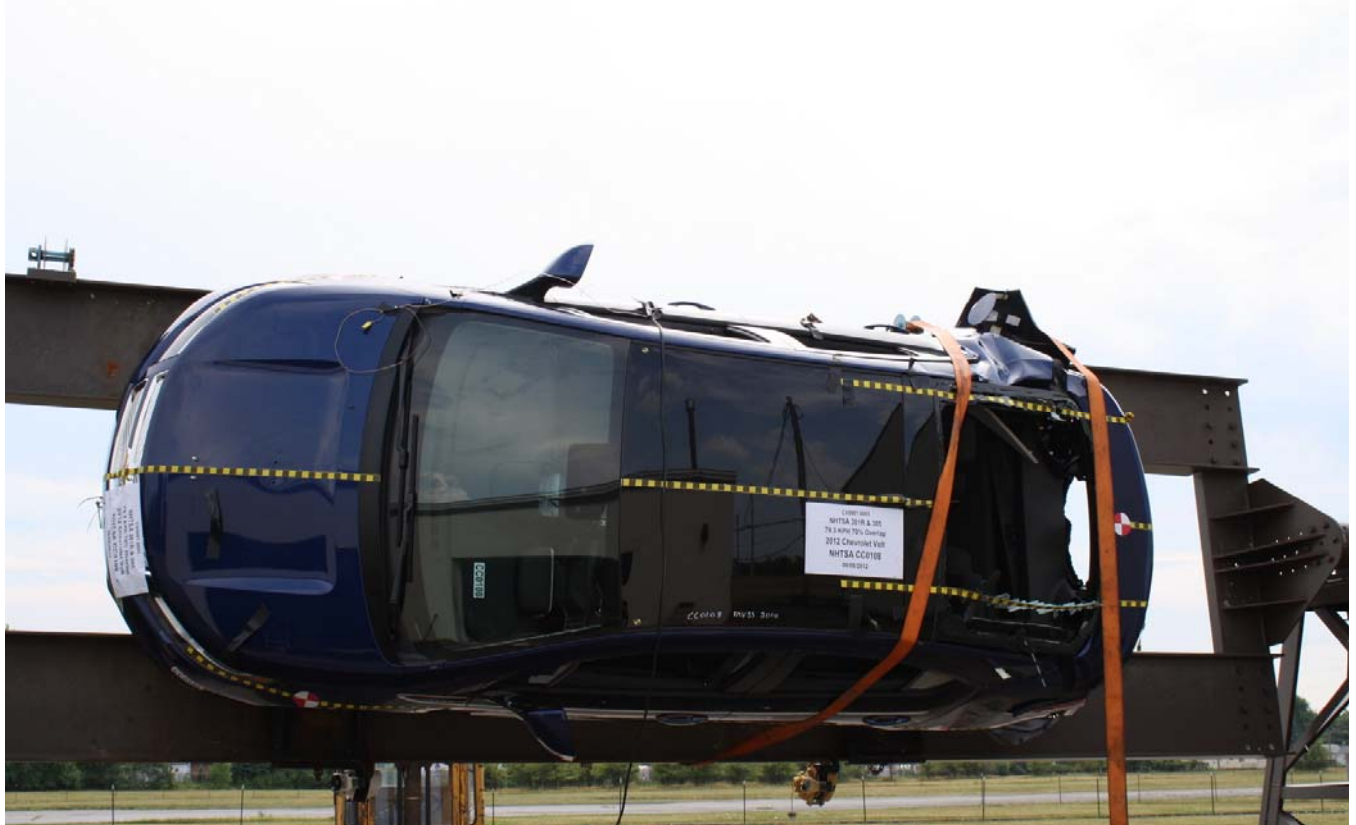
Figure A-74: FMVSS No. 305 Static Rollover at 270° Highlighting Propulsion Battery Location
