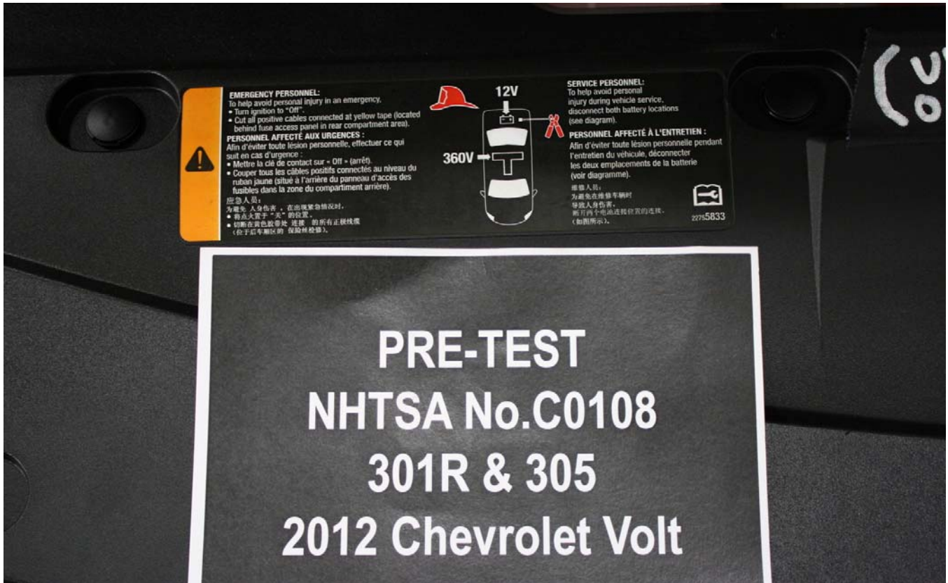
Figure A-43: First Responder Warning Label
