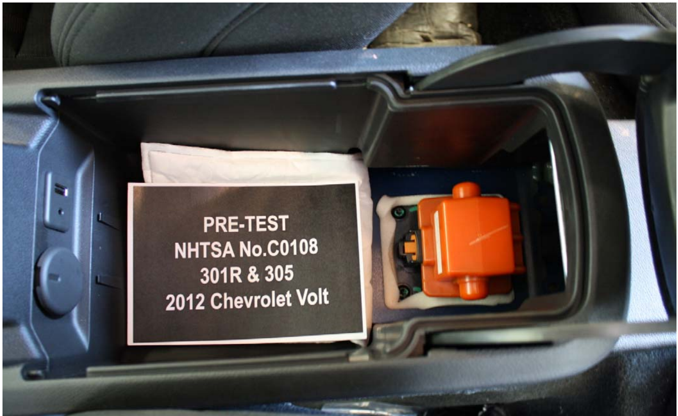
Figure A-46: Manual High Voltage Service Disconnect in Place
