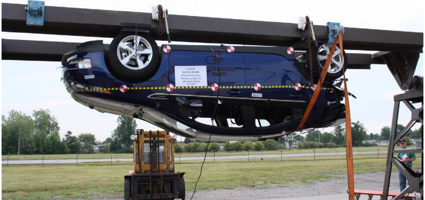
Figure A-73: FMVSS No. 305 Static Rollover at 180° Highlighting Propulsion Battery Location
