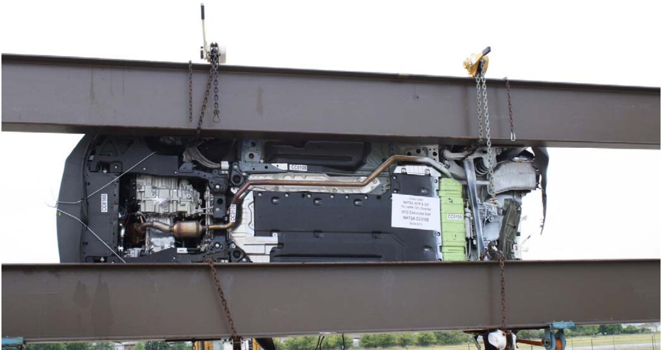
Figure A-72: FMVSS No. 305 Static Rollover at 90° Highlighting Propulsion Battery Location
