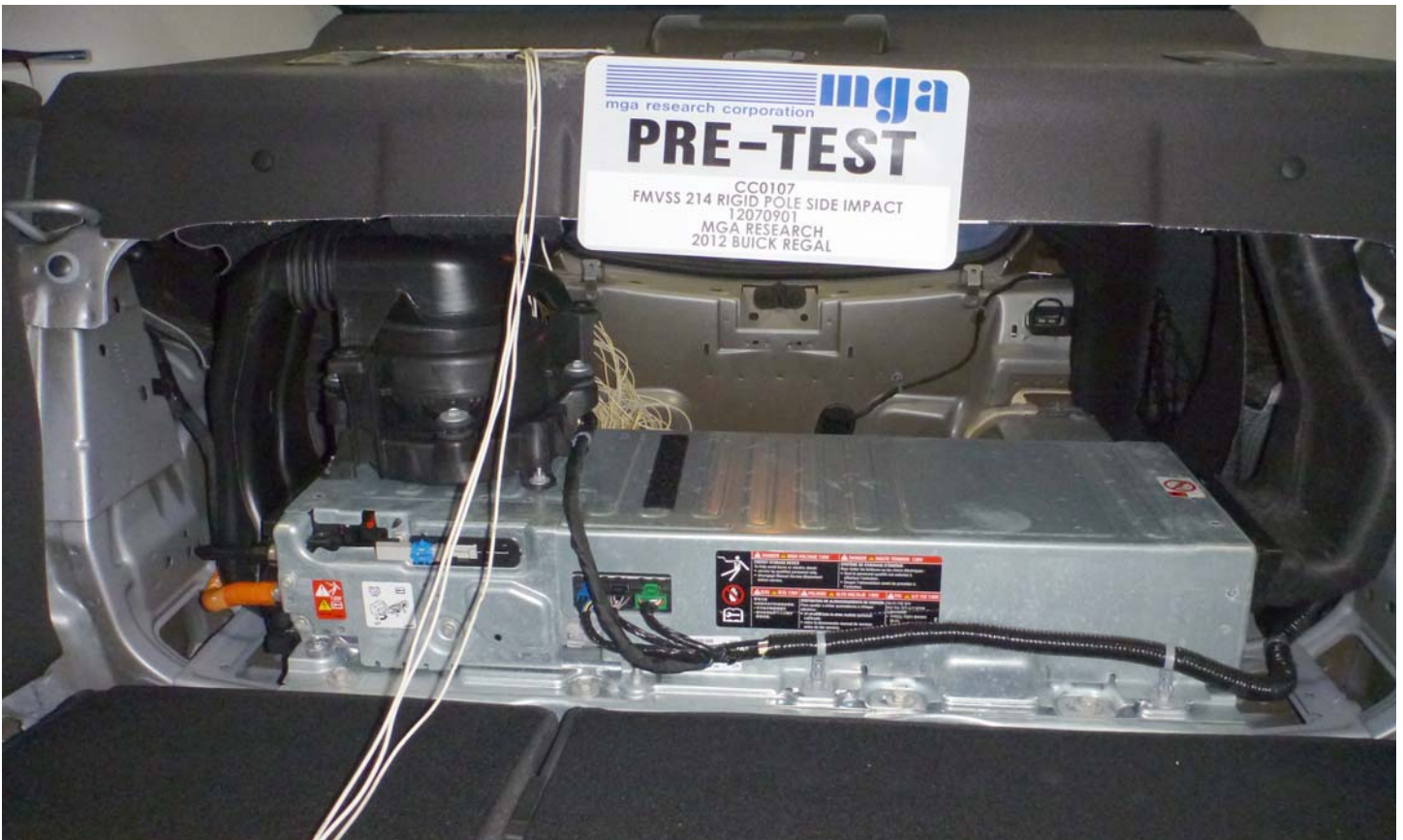
Pre-Impact Front View of Propulsion Battery
