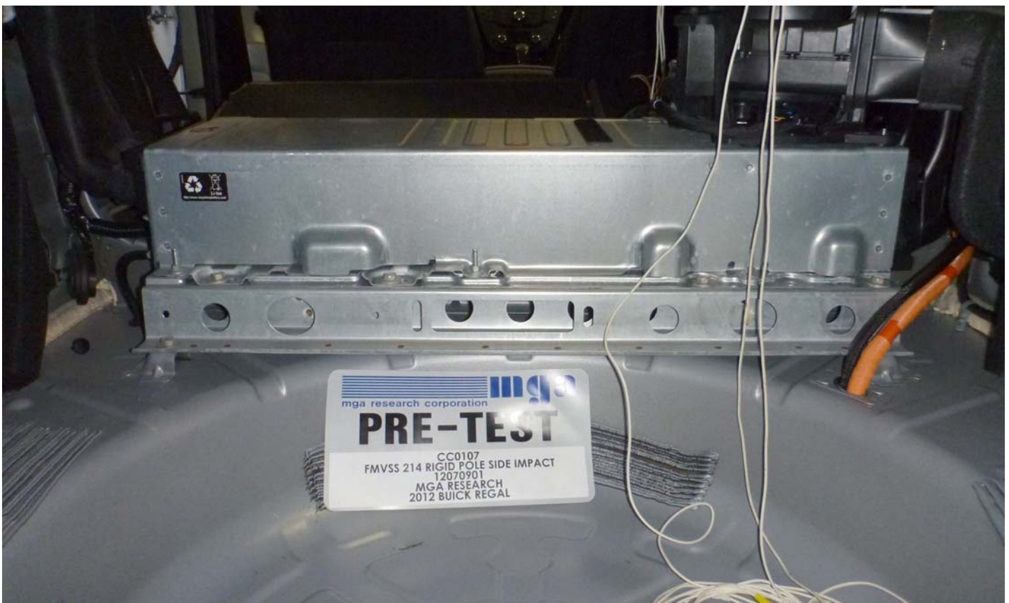
Pre-Impact Rear View of Propulsion Battery
