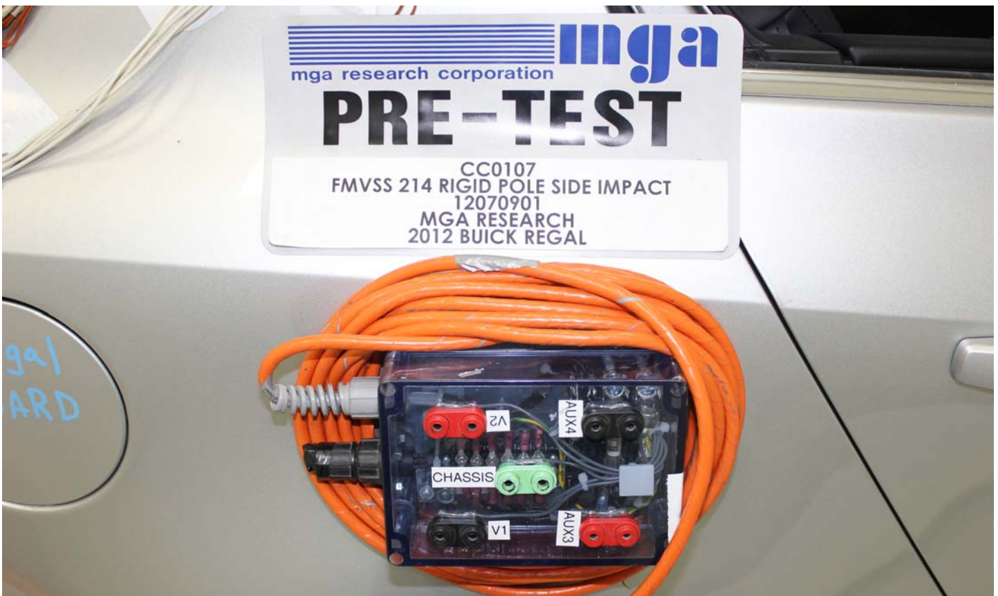
Pre-Impact View of Installed Impact Interface Port
