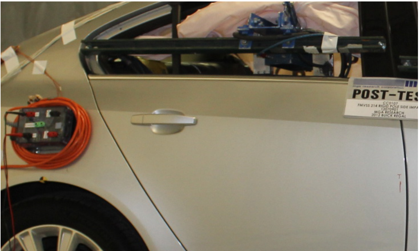
Post-Impact View of Installed Impact Interface Port
