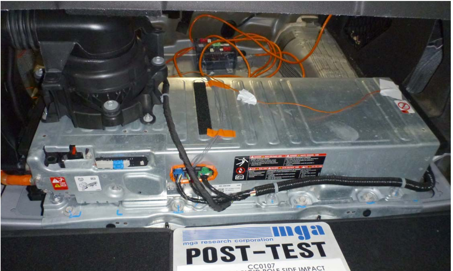
Post-Impact Front View of Propulsion Battery
