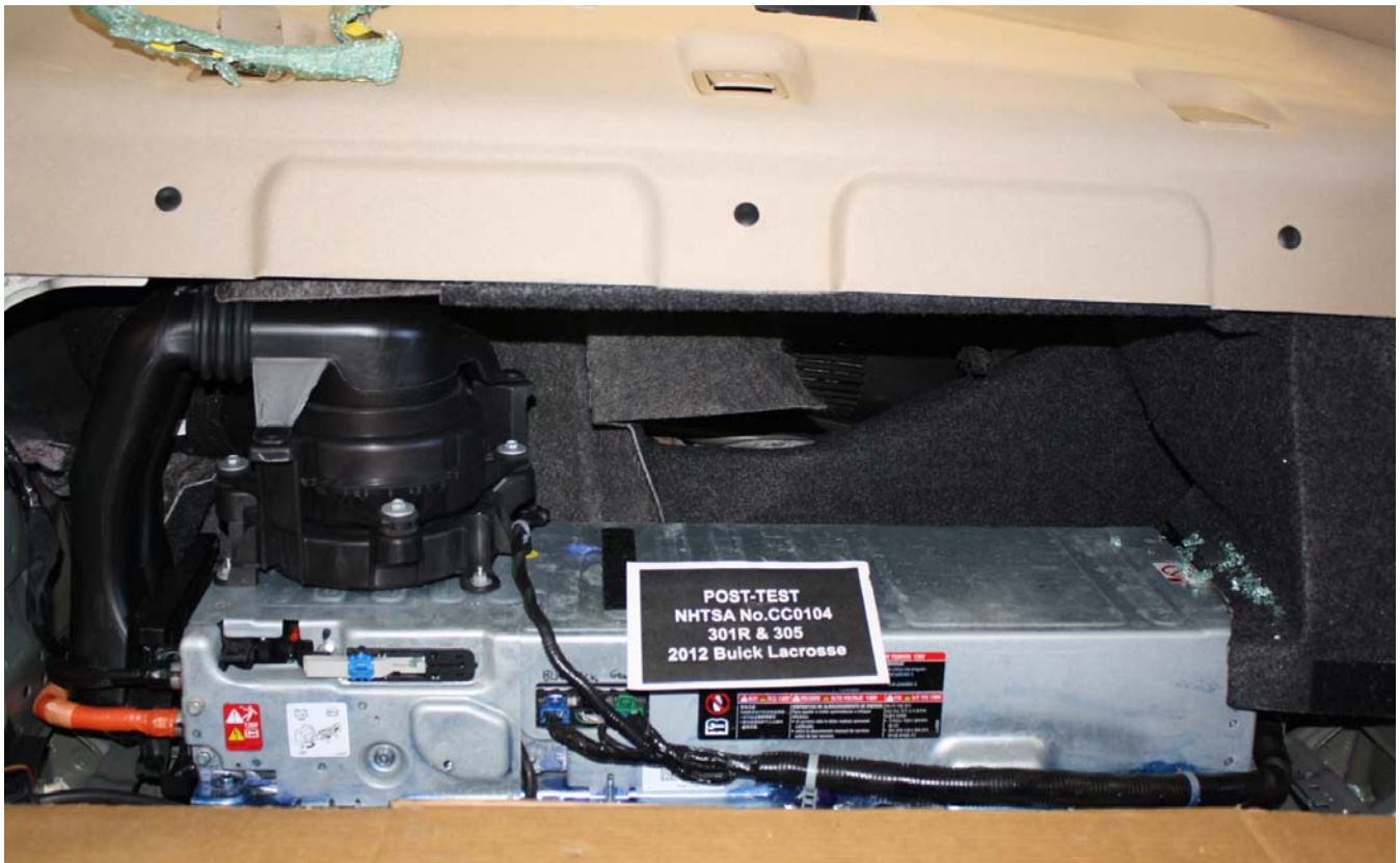
Figure A-50: Post-Impact Front View of Propulsion Battery
