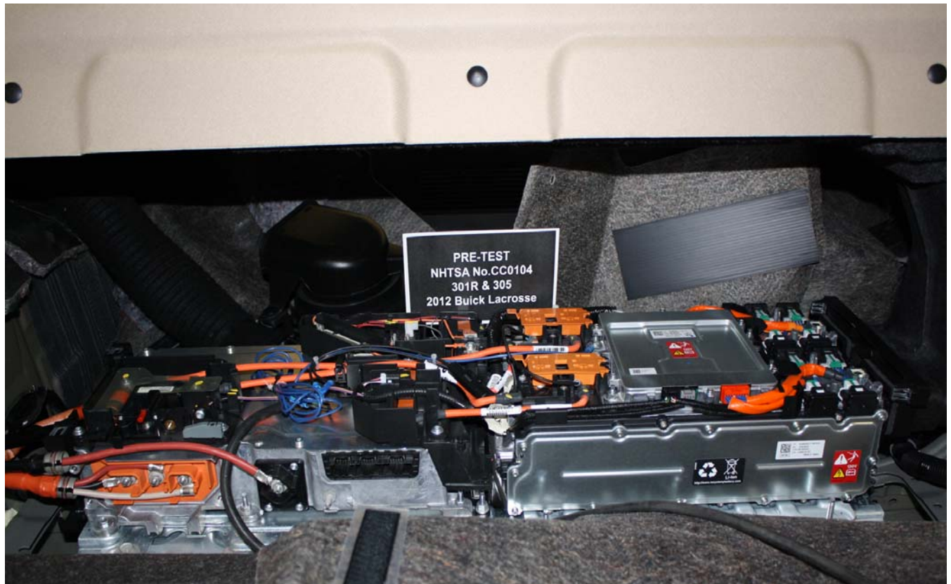
Figure A-54: Pre-Impact View of Propulsion Battery Module(s)
