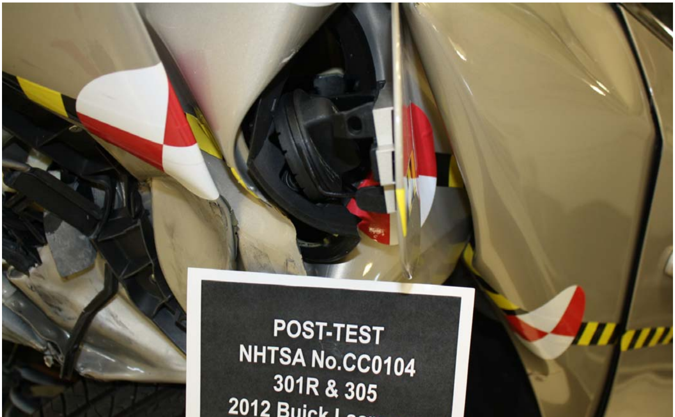
Figure A-38: Post-Test Fuel Filler Cap View
