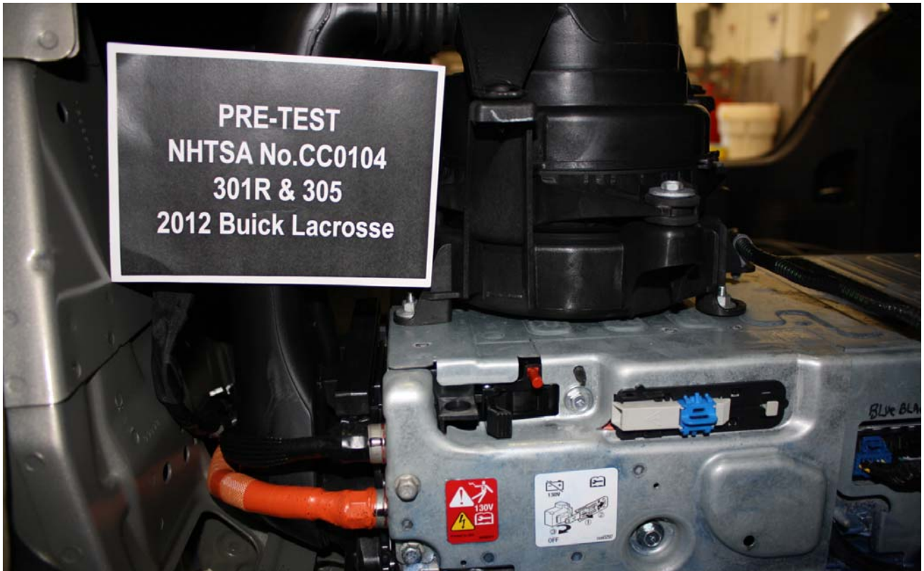
Figure A-47: Manual High Voltage Service Disconnect Removed (Plug)
