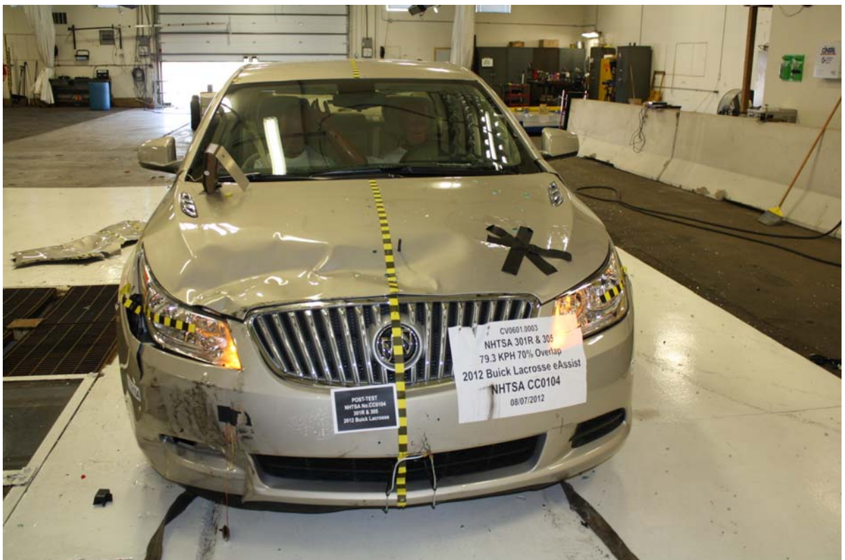
Figure A-6: Post-Test Front View
