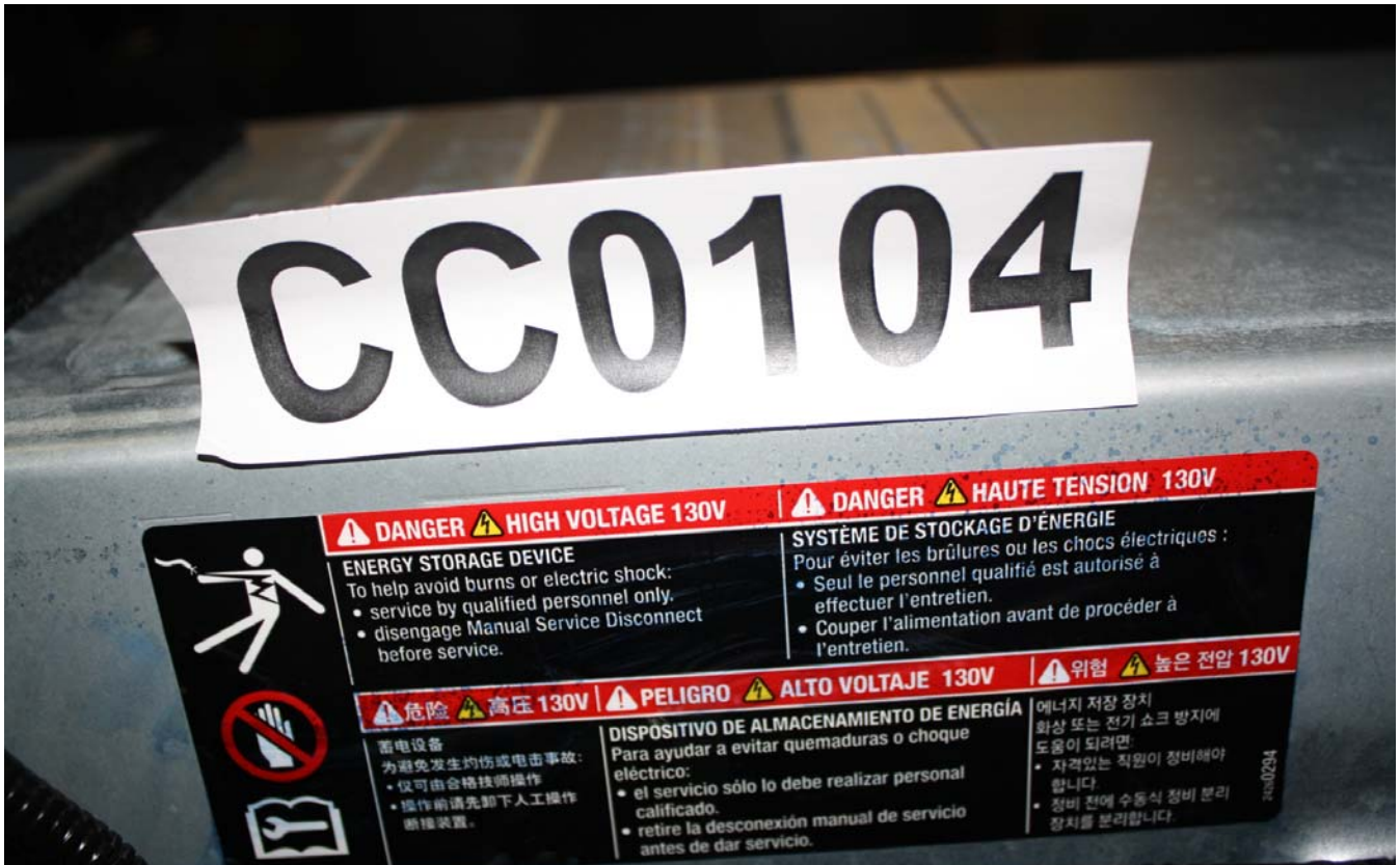
Figure A-41: Auxiliary Power Module Warning Label
