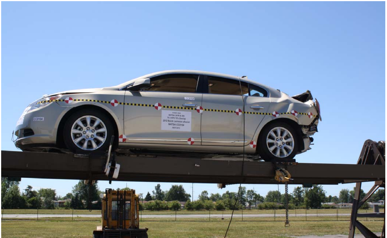
Figure A-71: FMVSS No. 301 Static Rollover 360° View
