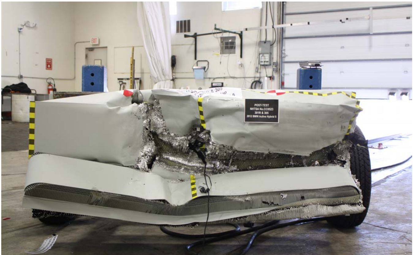
Figure A-22: Post-Test MDB Front View
