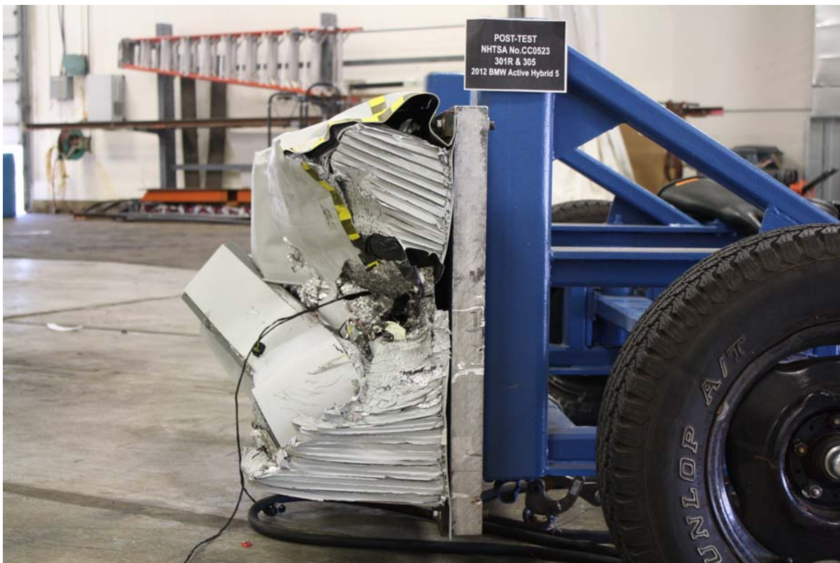
Figure A-24: Post-Test MDB Left Side View
