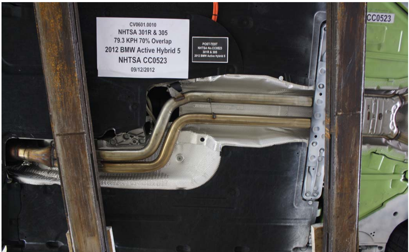
Figure A-34: Post-Test Mid Underbody View
