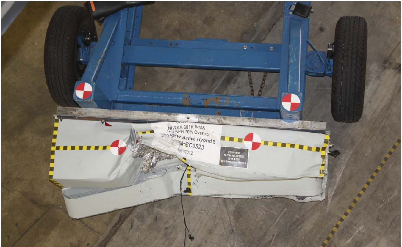
Figure A-28: Post-Test MDB Top View
