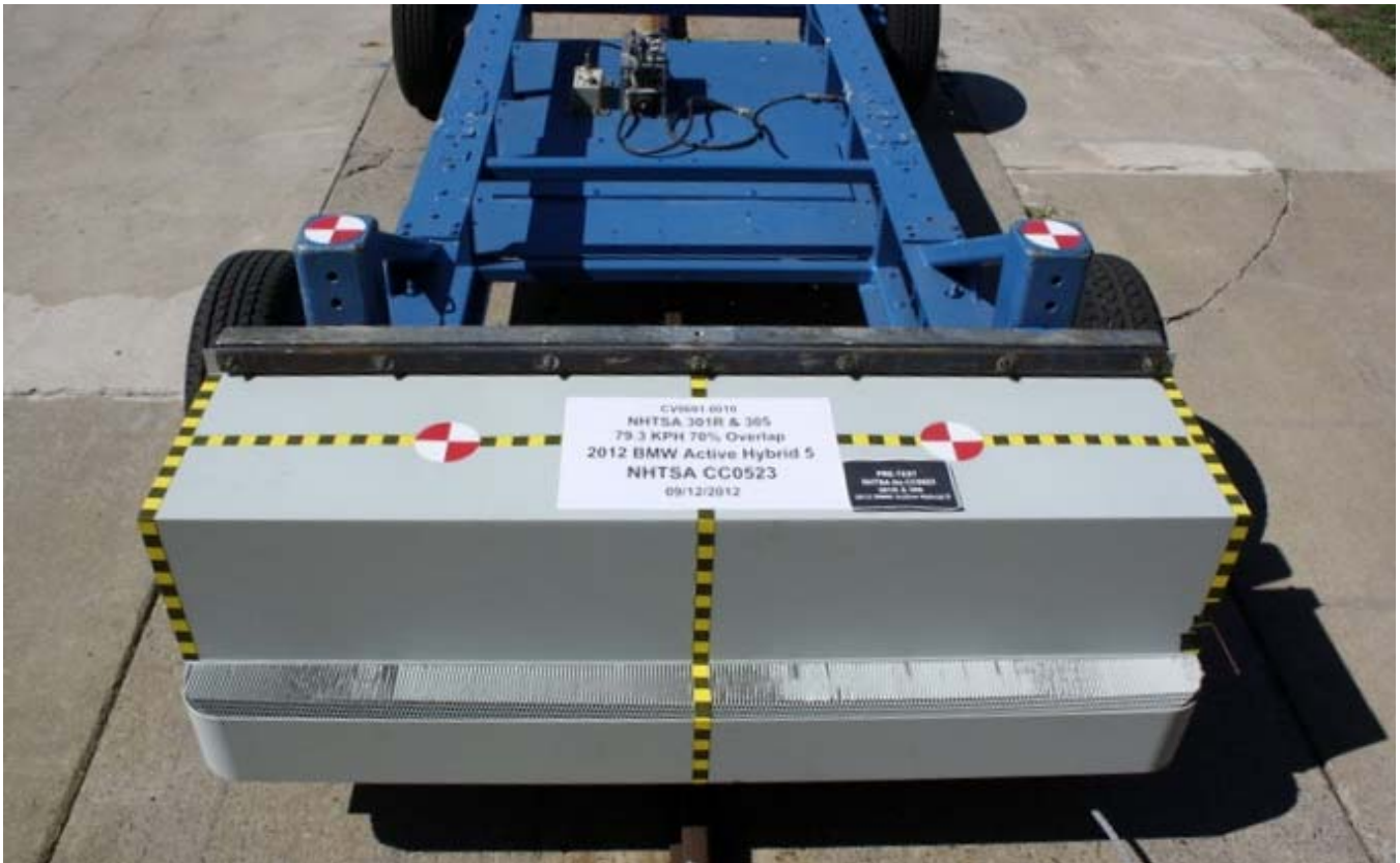
Figure A-27: Pre-Test MDB Top View
