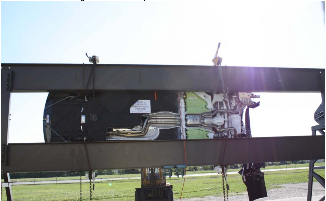
Figure A-68: FMVSS No. 301 Static Rollover 90° View
