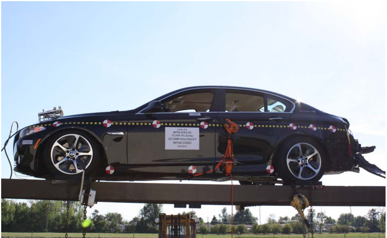
Figure A-71: FMVSS No. 301 Static Rollover 360° View
