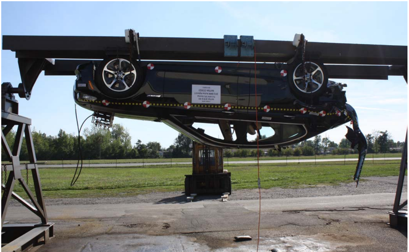
Figure A-69: FMVSS No. 301 Static Rollover 180° View
