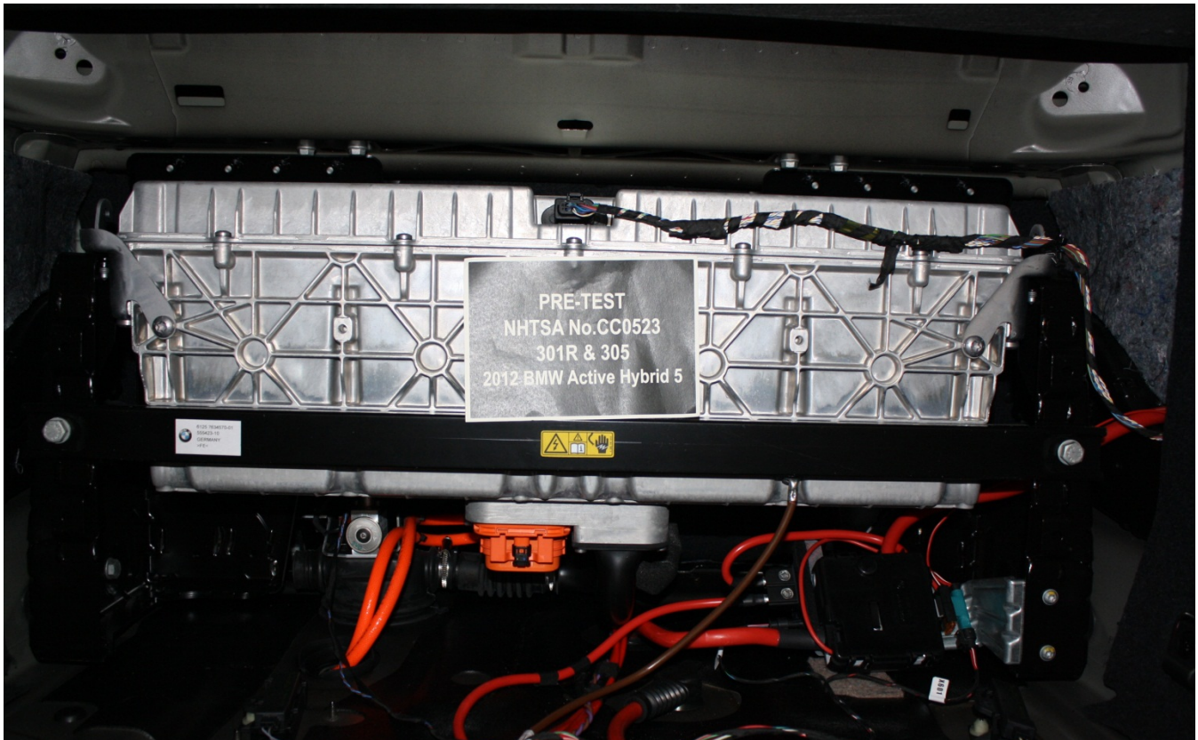
Figure A-49: Pre-Impact View of Propulsion Battery
