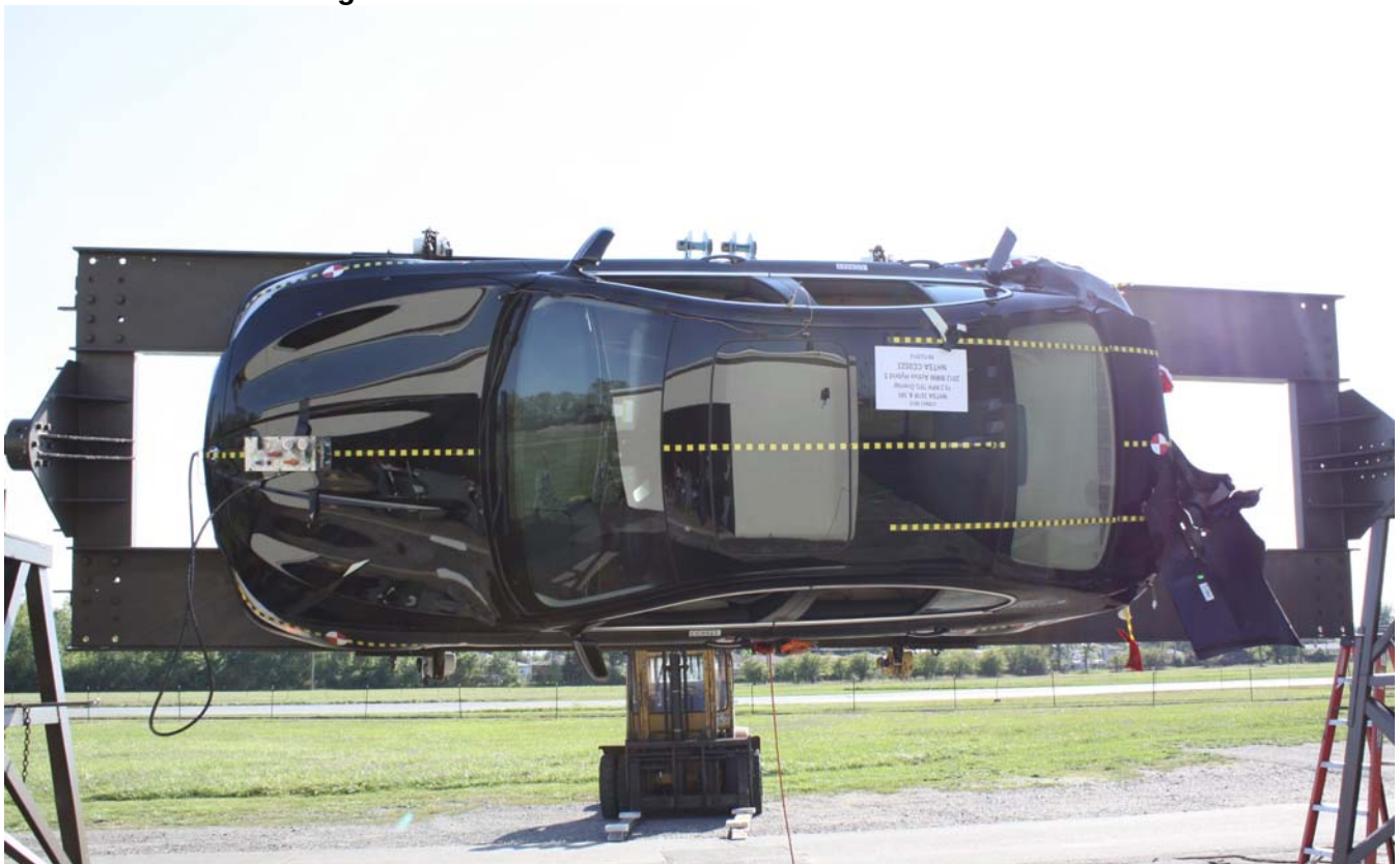
Figure A-70: FMVSS No. 301 Static Rollover 270° View
