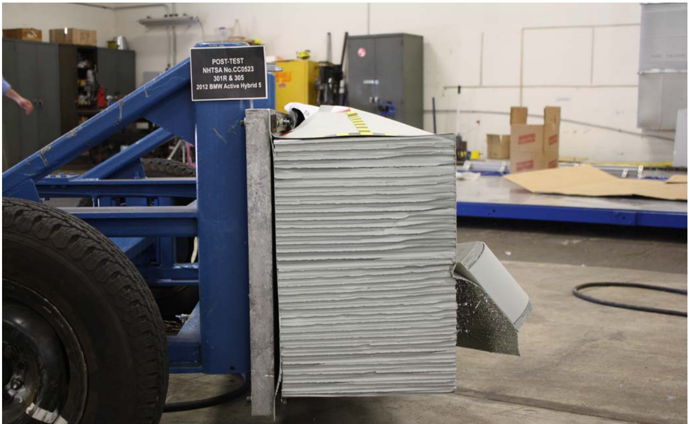
Figure A-26: Post-Test MDB Right Side View
