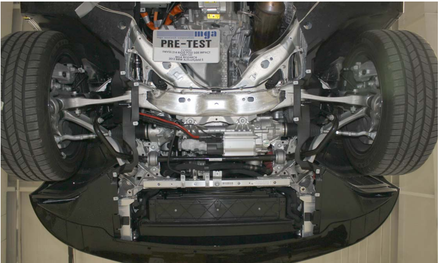
05 Pre-Impact View of Electric Propulsion Drive
