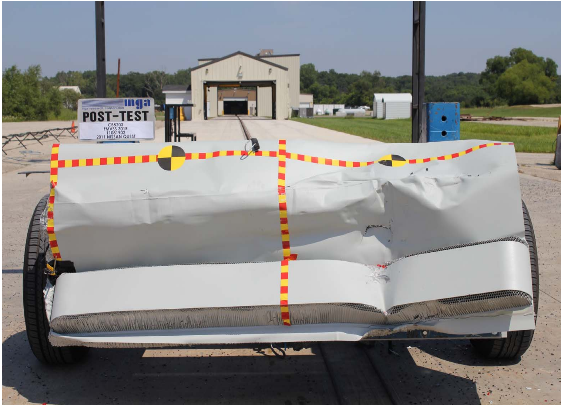
Post-Test Front View of MDB
