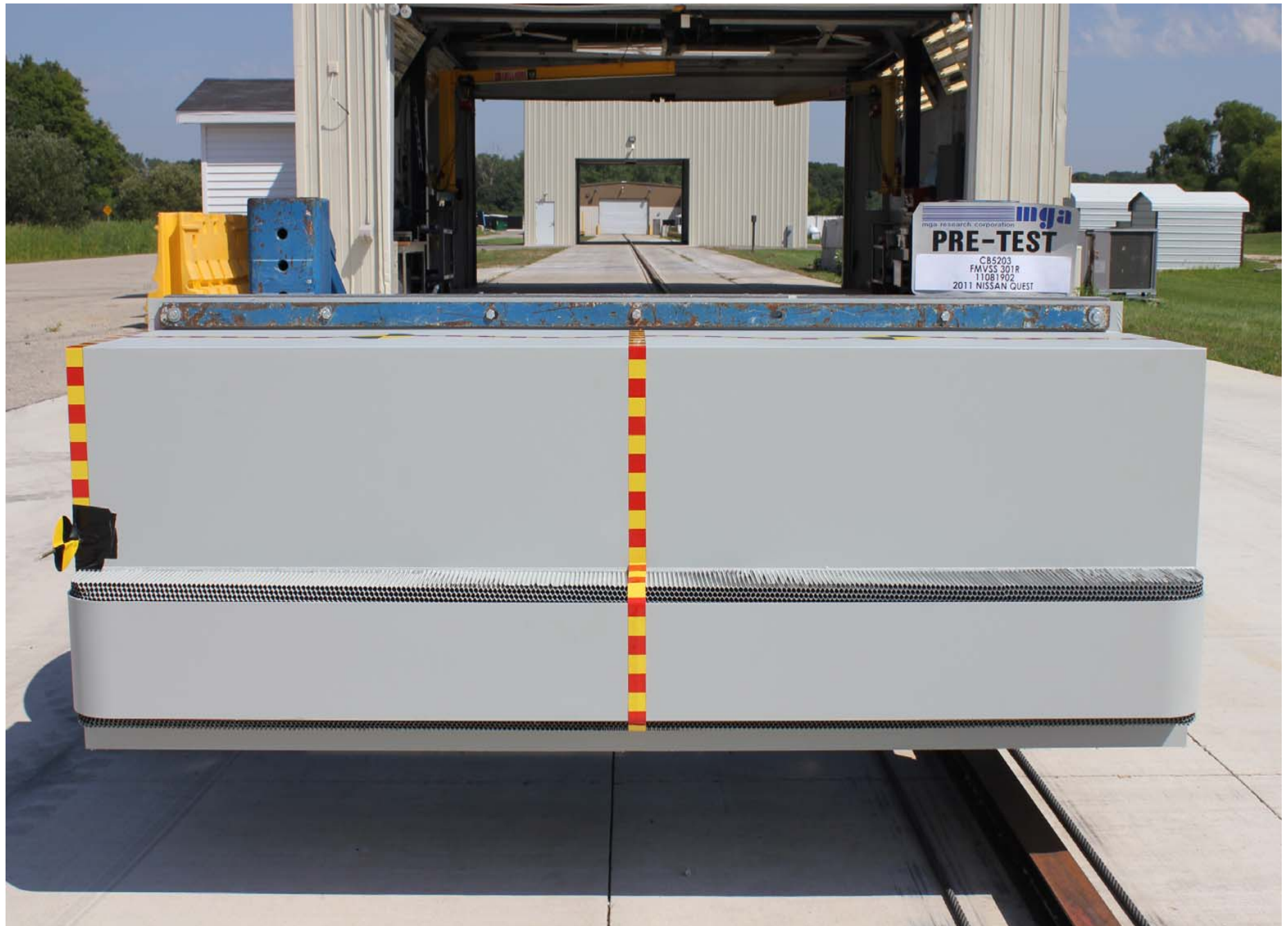
Pre-Test Front View of MDB
