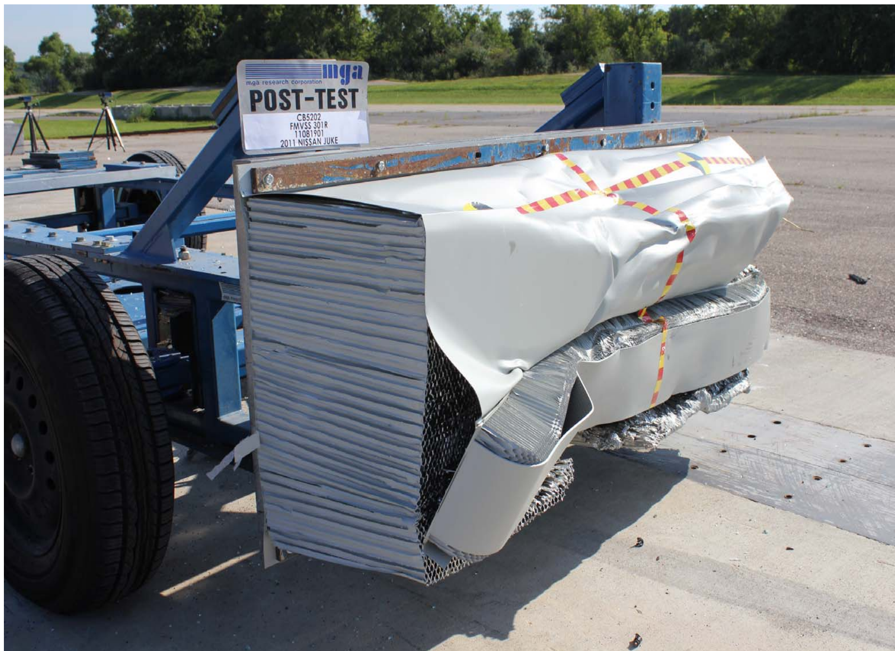
Post-Test ¾ Right Side View of MDB
