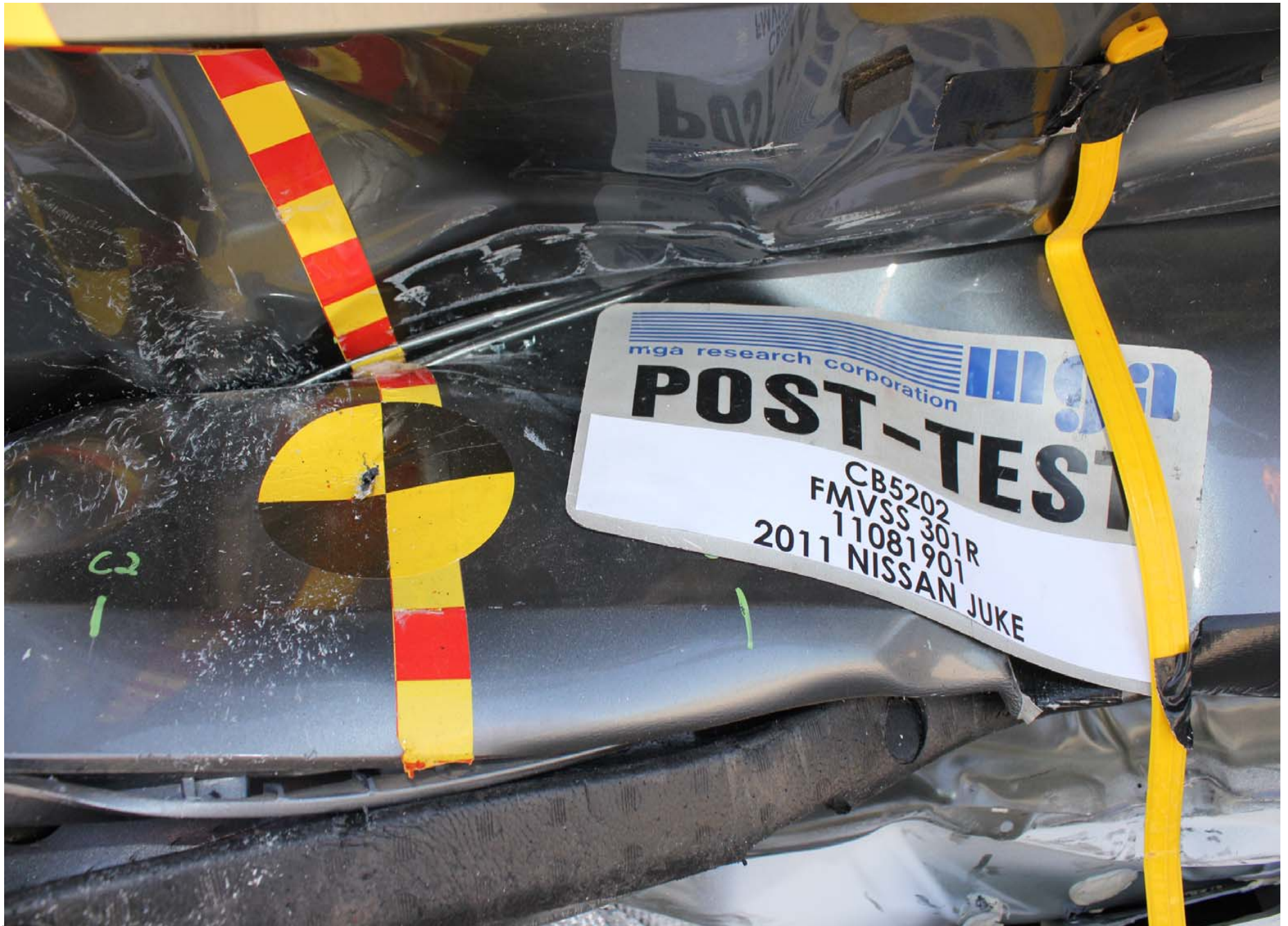
Post-Test Impact Point
