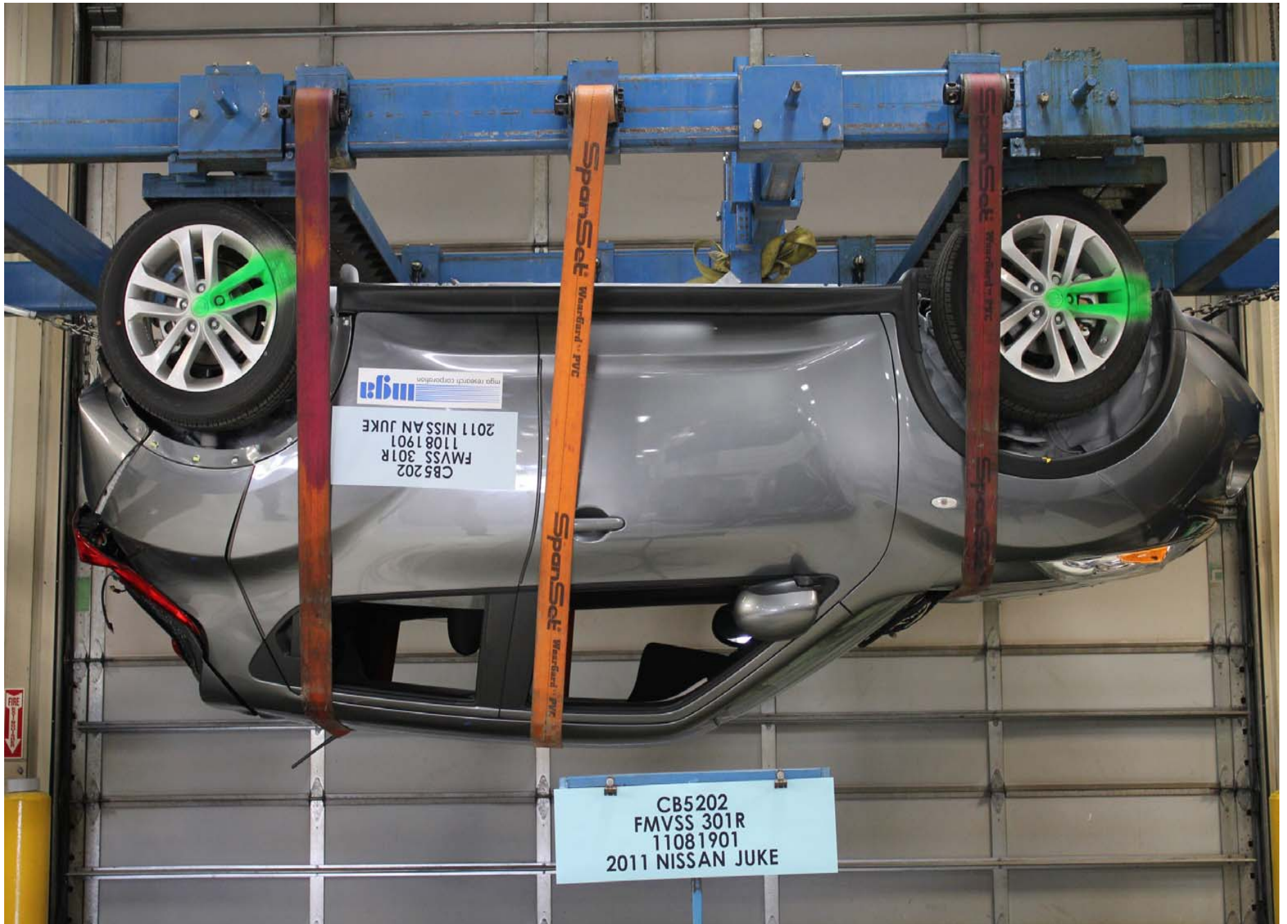
Static Rollover at 180 Degrees
