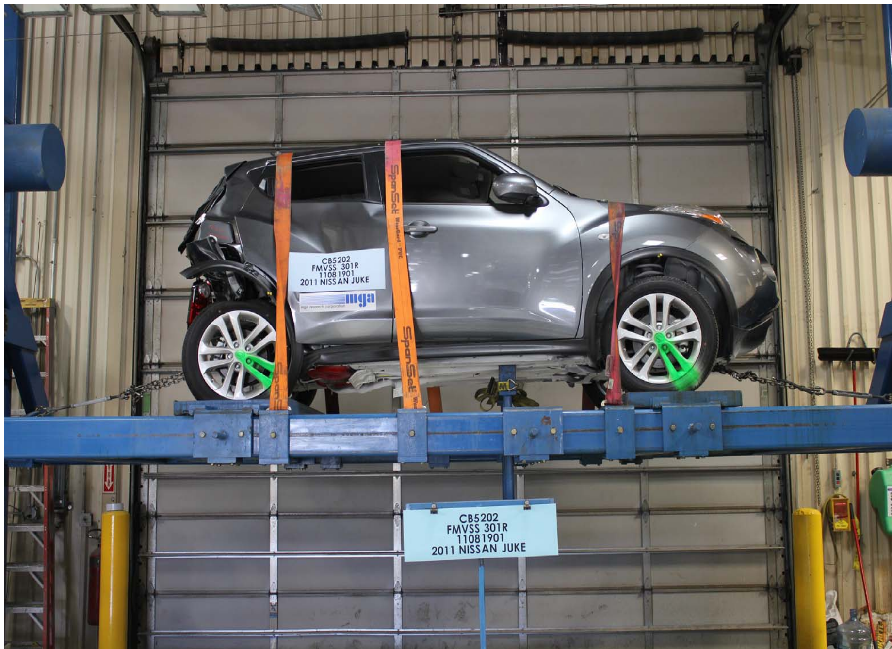
Static Rollover at 360 Degrees
