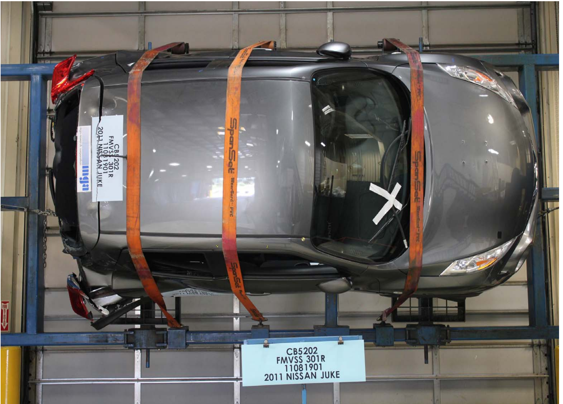
Static Rollover at 90 Degrees
