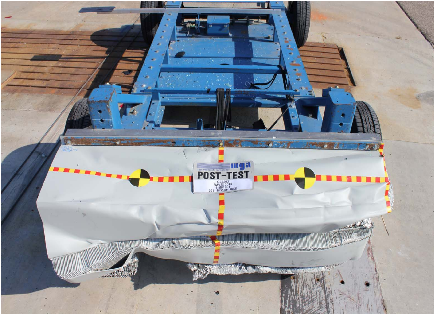
Post-Test Top View of MDB
