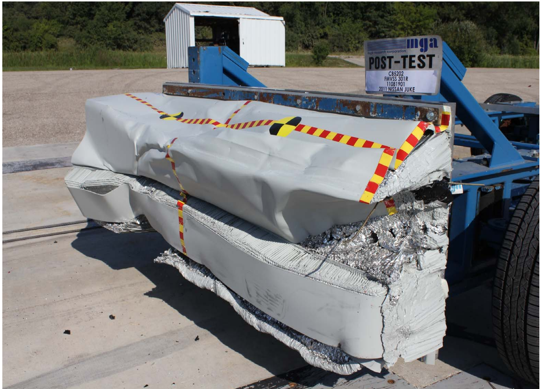
Post-Test \frac{3}{4} Left Side View of MDB
