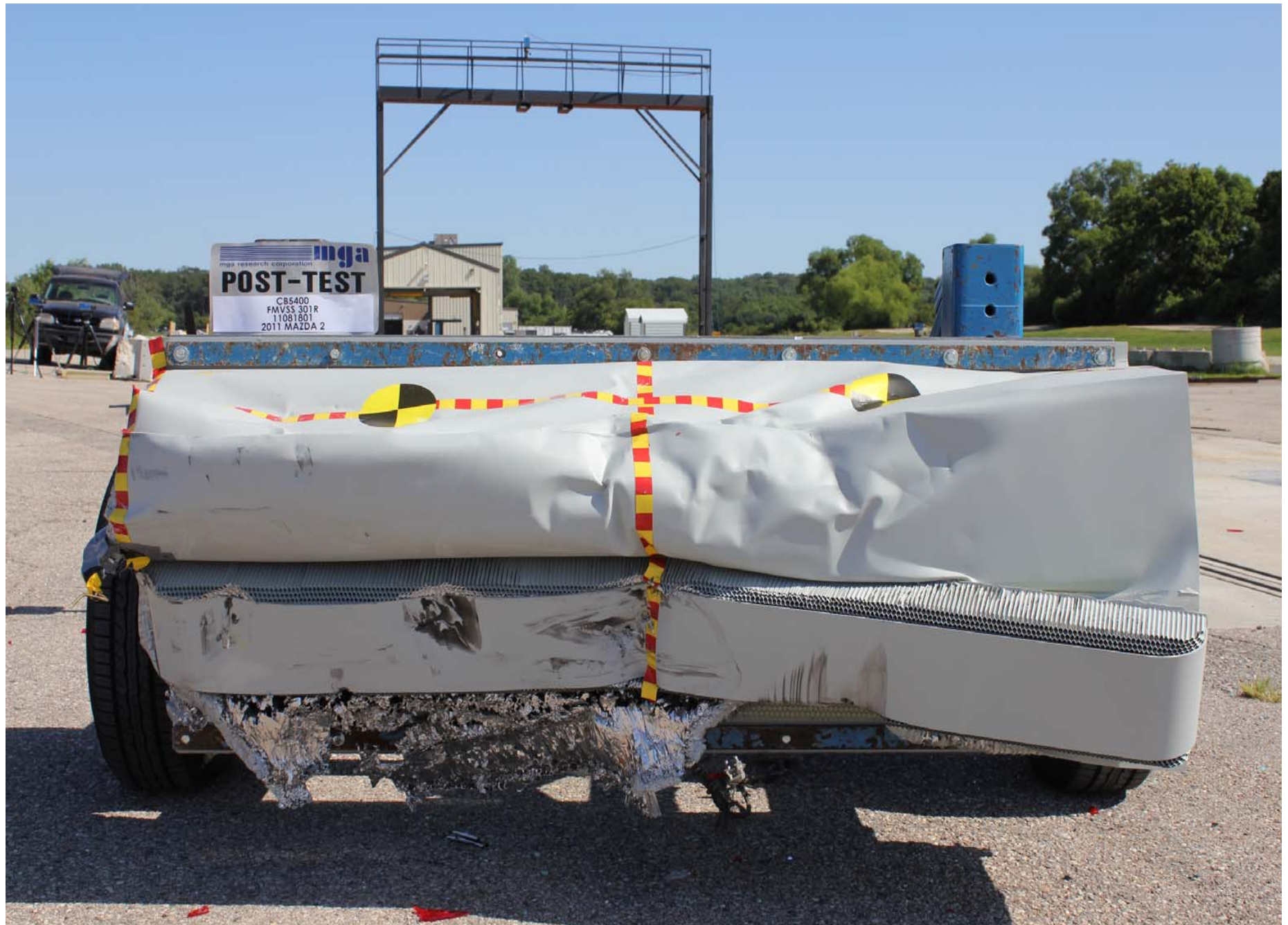
Post-Test Front View of MDB
