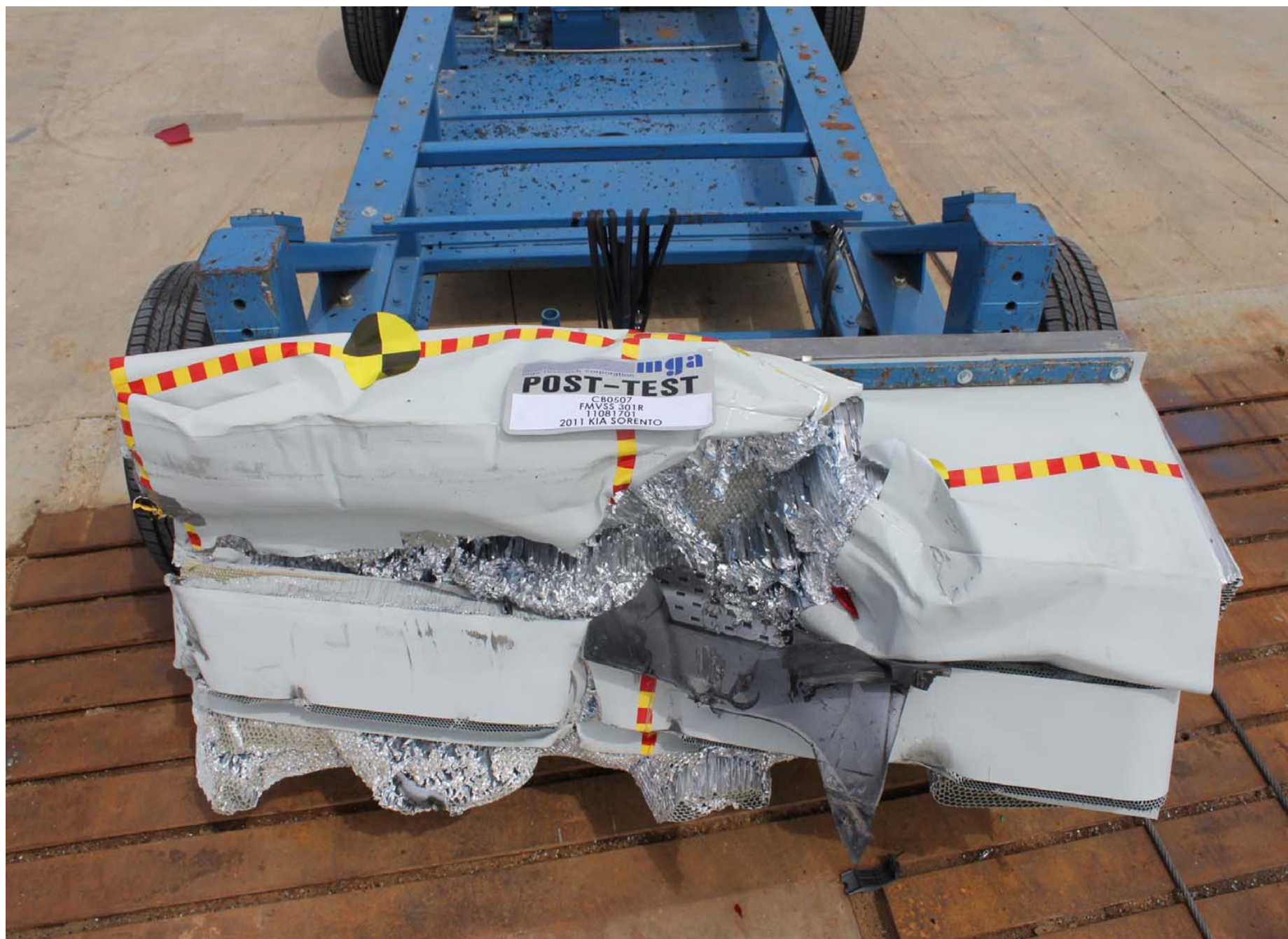
Post-Test Top View of MDB
