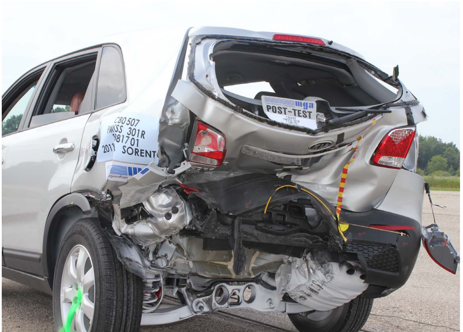
Post-Test Left Rear Close-up View of Vehicle
