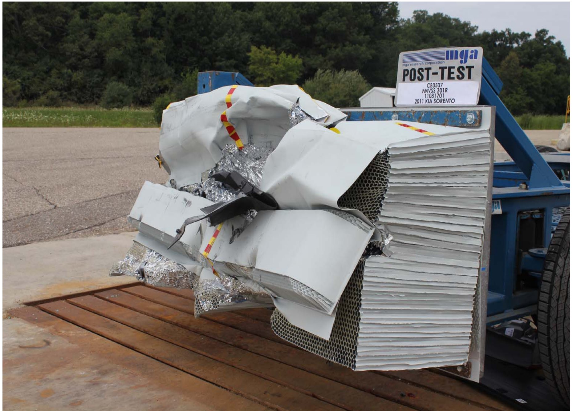
Post-Test \frac{3}{4} Left Side View of MDB
