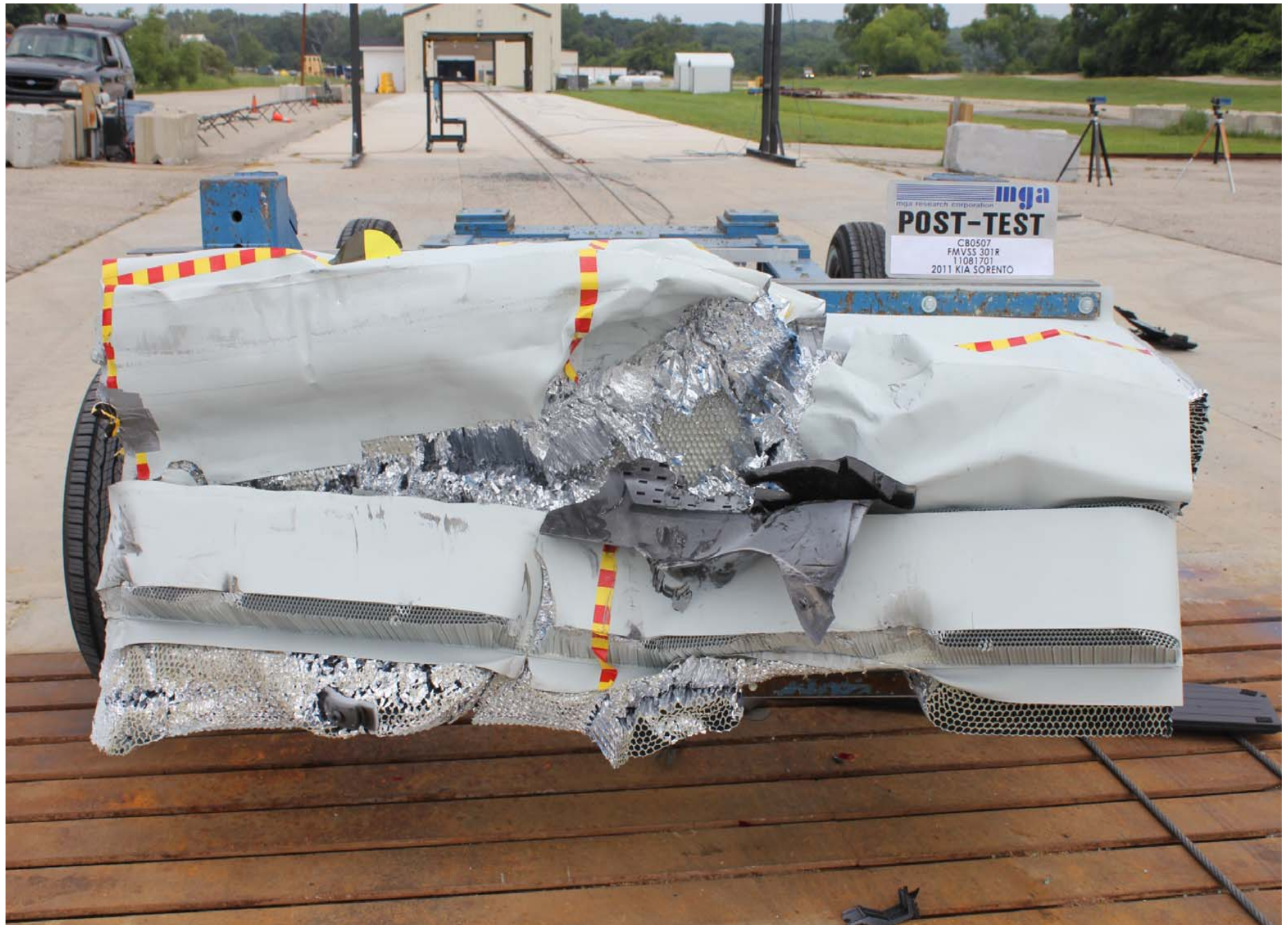
Post-Test Front View of MDB
