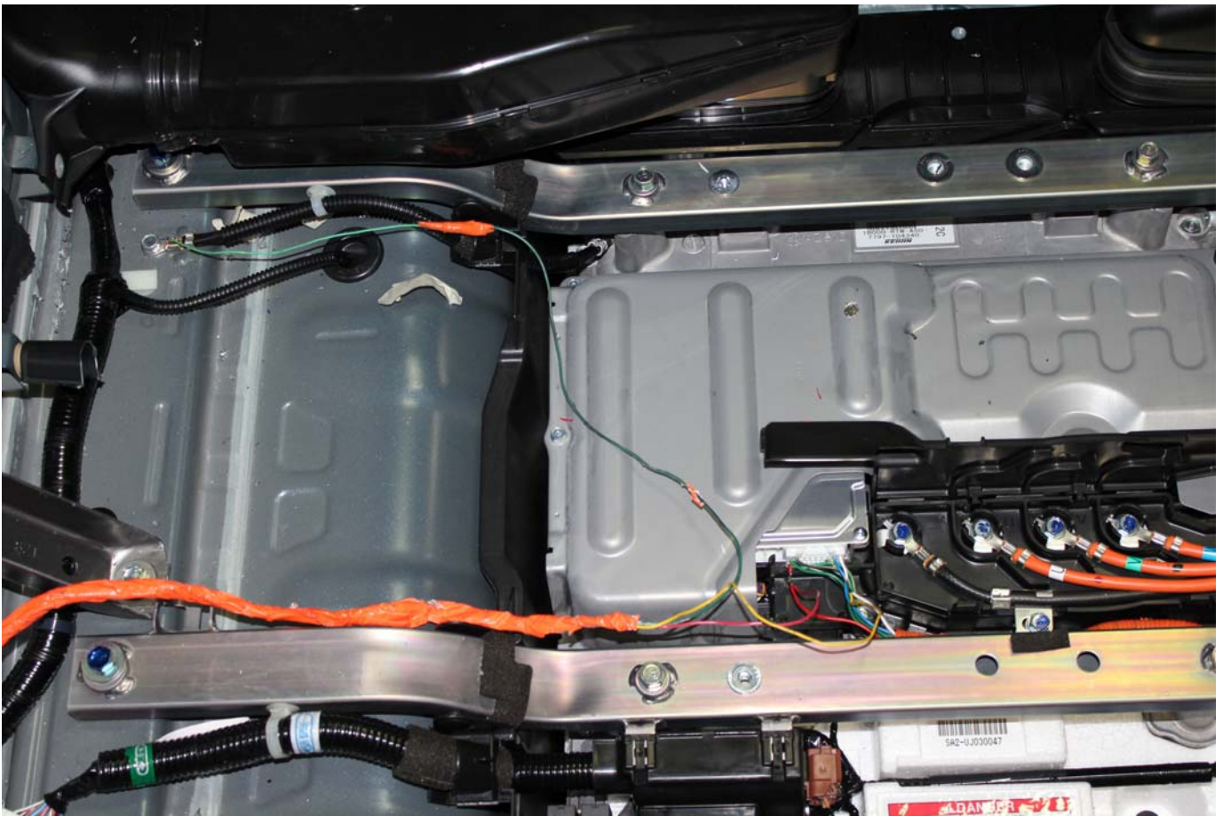
Ground Location/Close-up of Leads Attached
