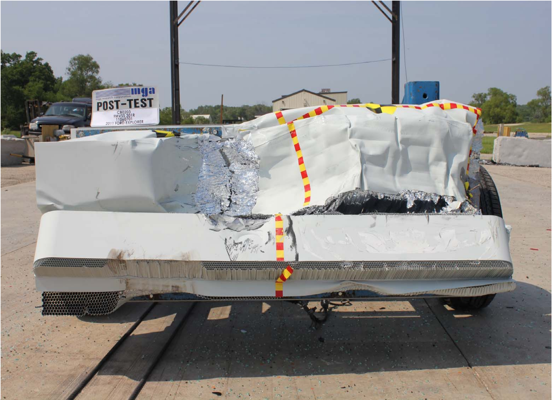
Post-Test Front View of MDB
