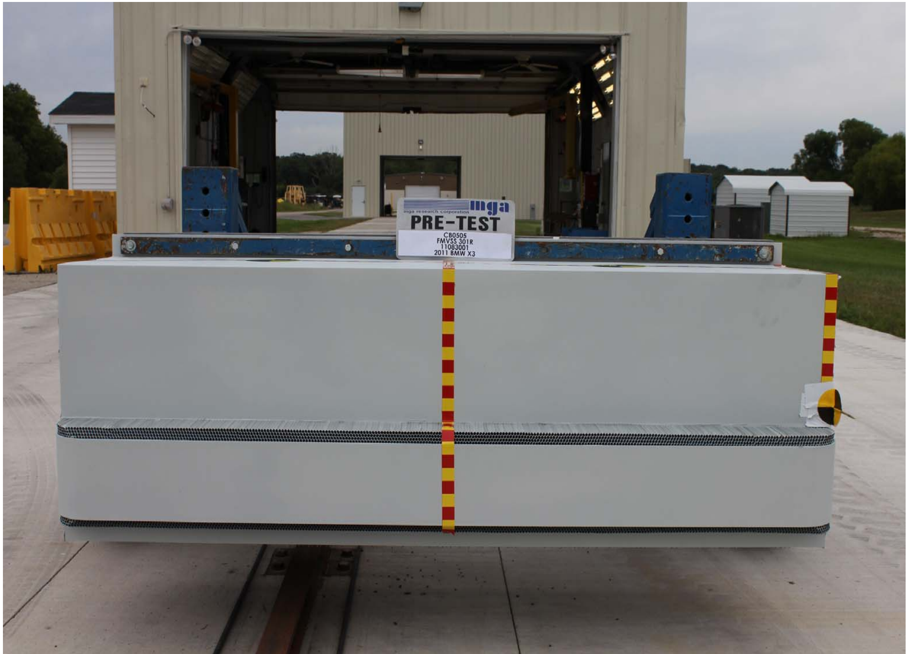
Pre-Test Front View of MDB
