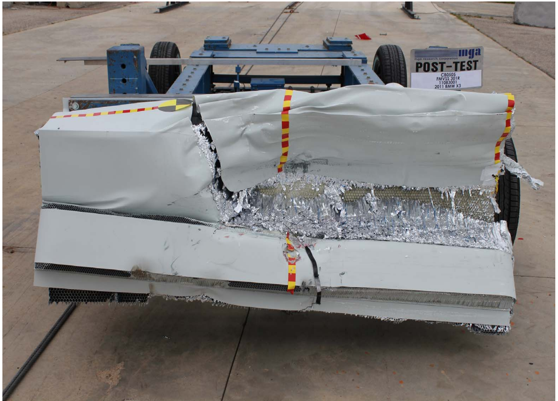
Post-Test Front View of MDB
