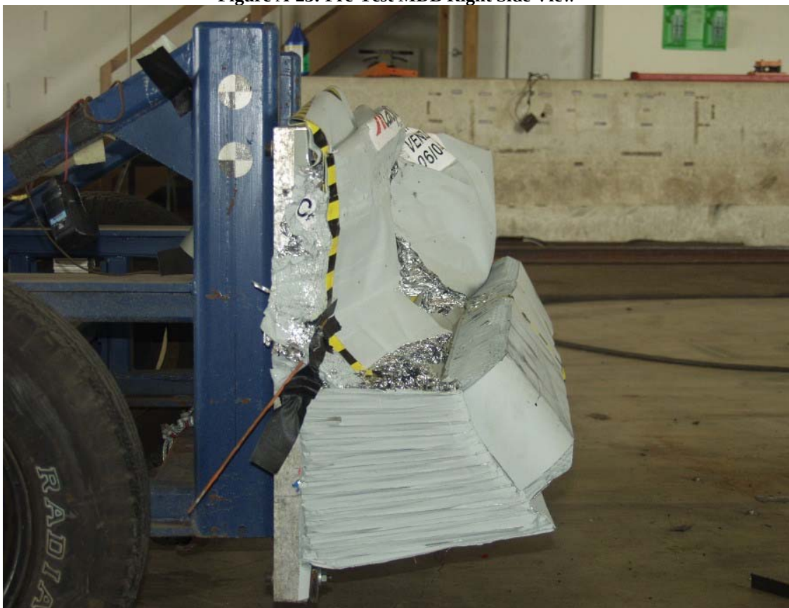
Figure A-24: Post-Test MDB Right Side View
