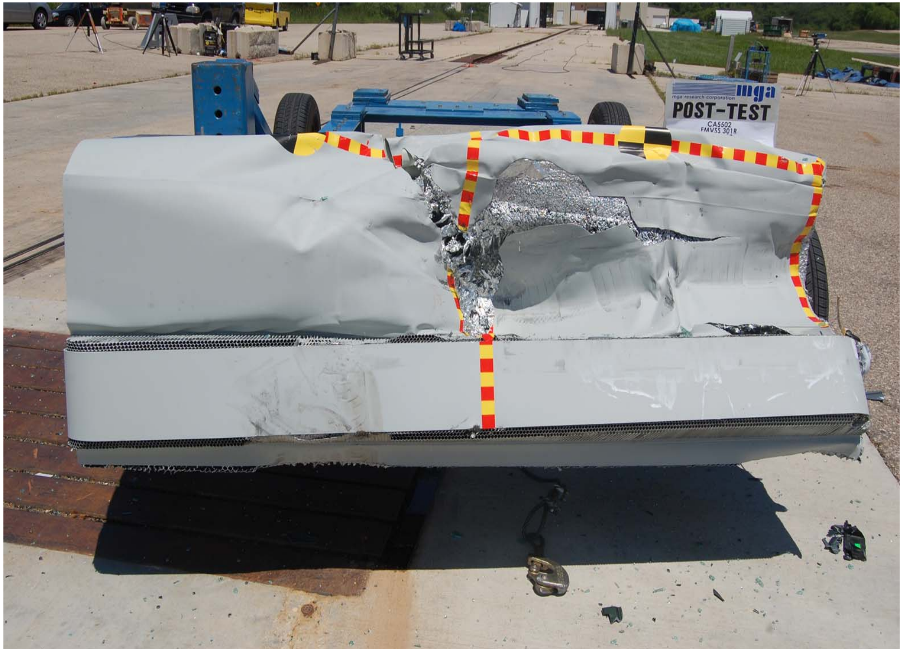
Post-Test Front View of MDB
