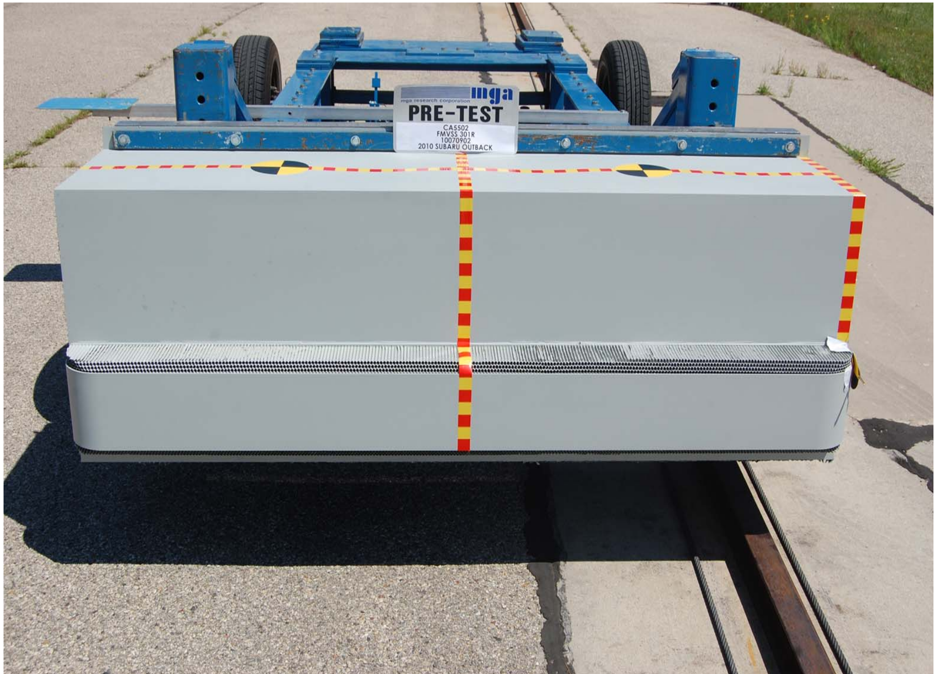
Pre-Test Front View of MDB
