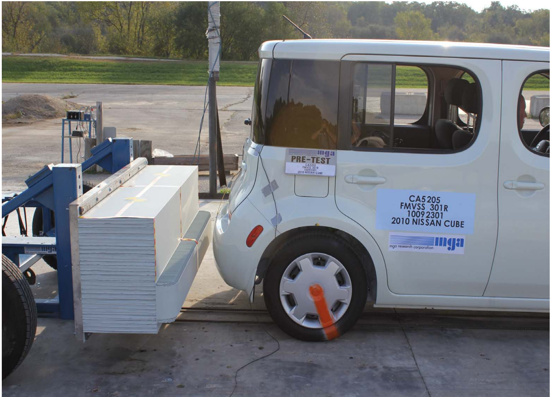
Pre-Test Right Rear Close-up View of MDB and Vehicle
