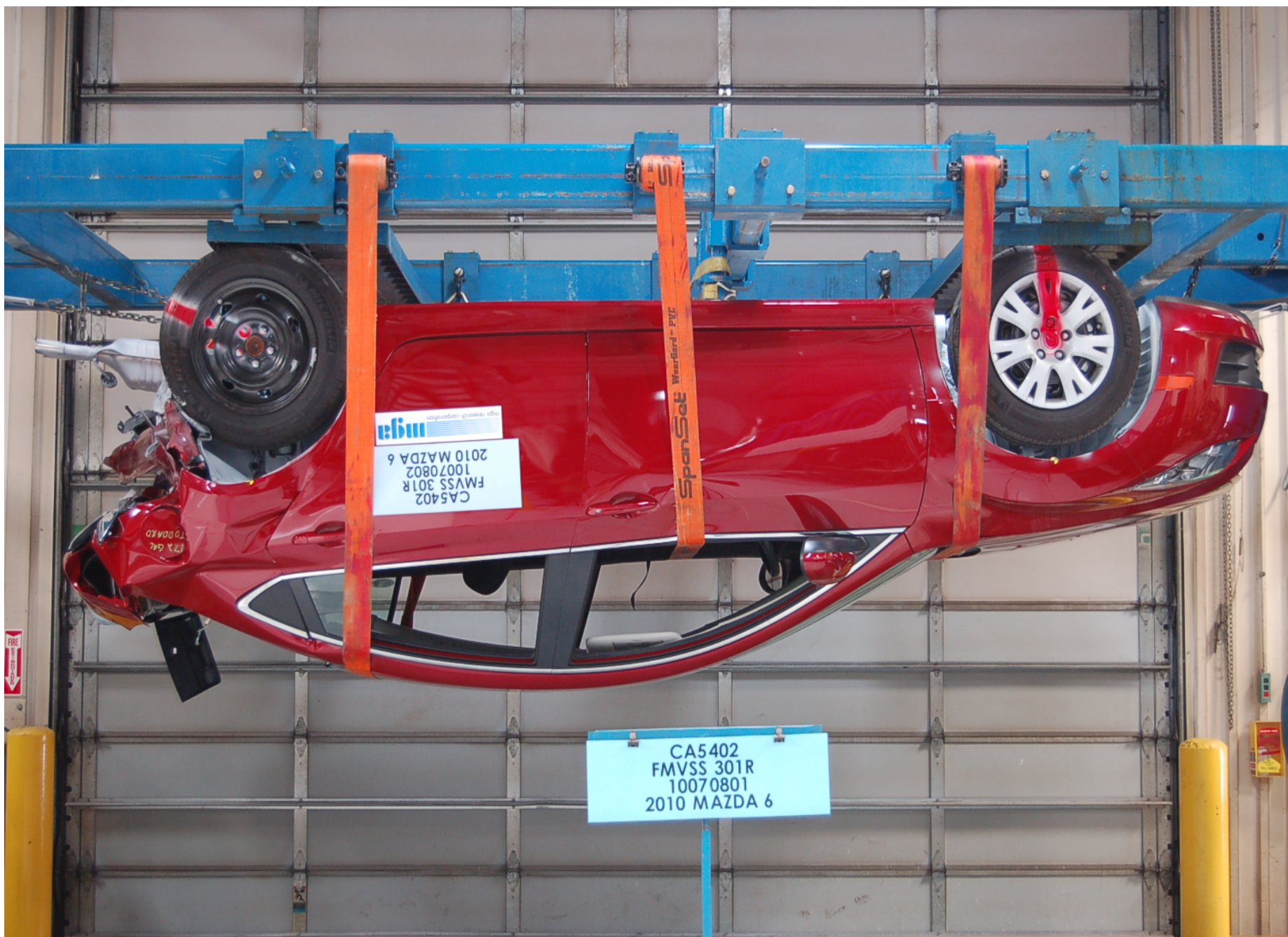
Static Rollover at 180 Degrees
