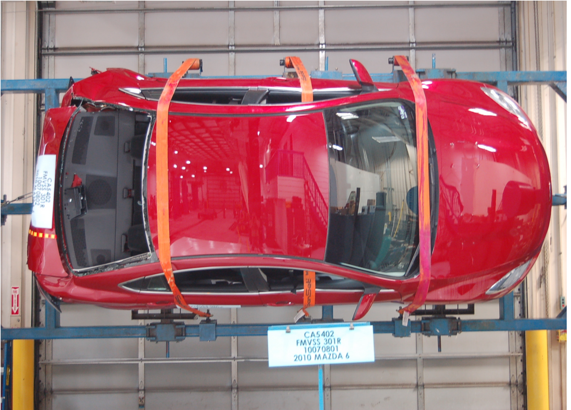
Static Rollover at 90 Degrees
