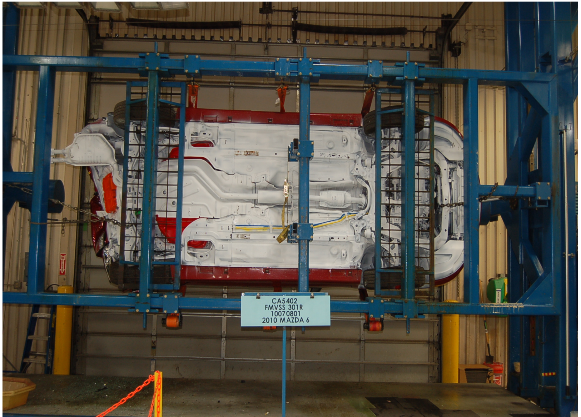
Static Rollover at 270 Degrees
