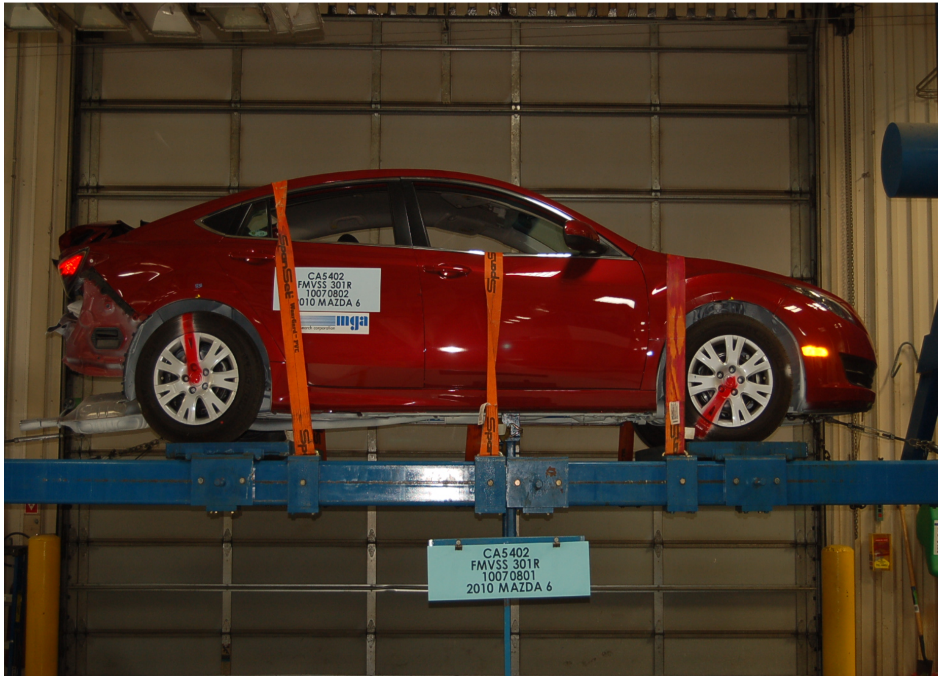
Static Rollover at 360 Degrees
