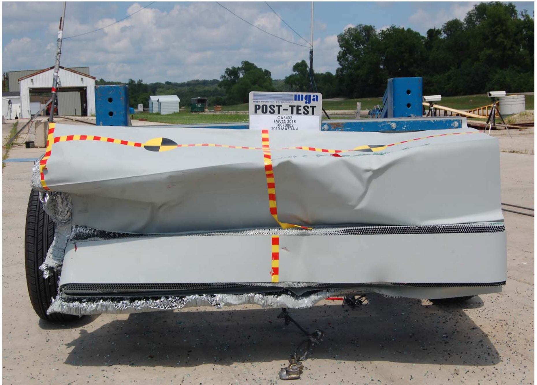
Post-Test Front View of MDB
