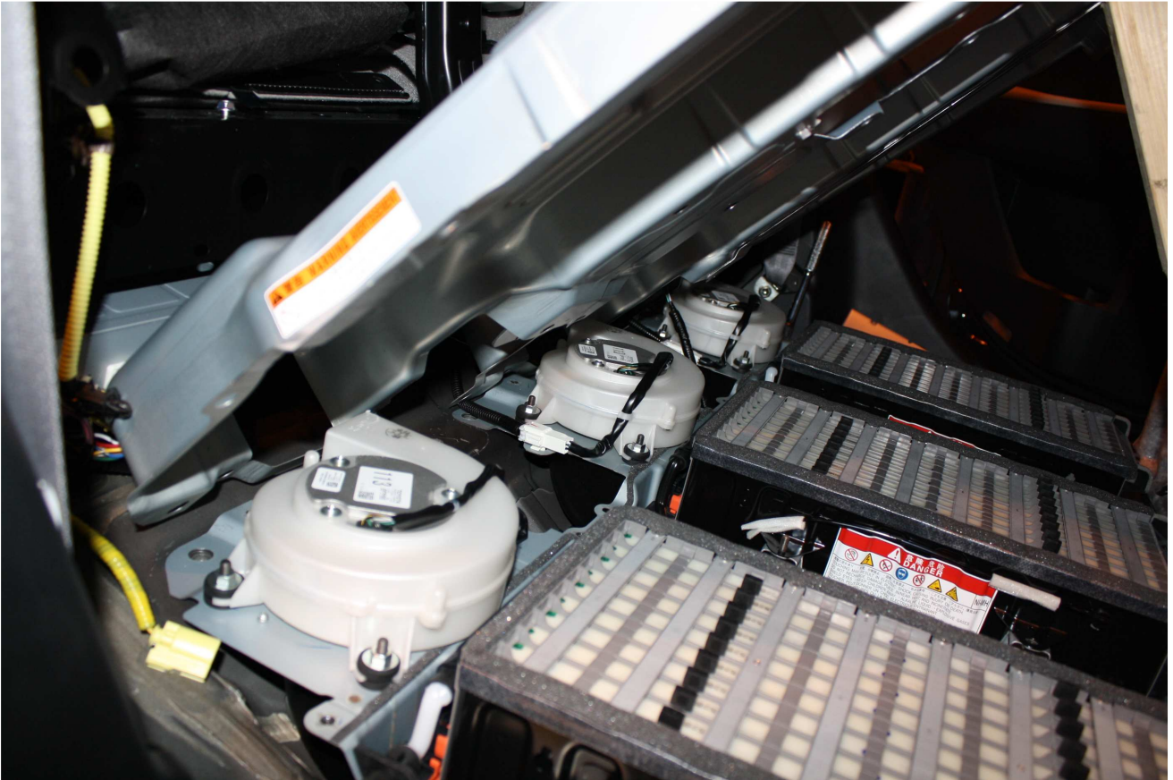
Figure A-35: Pre-Test Propulsion Battery View
