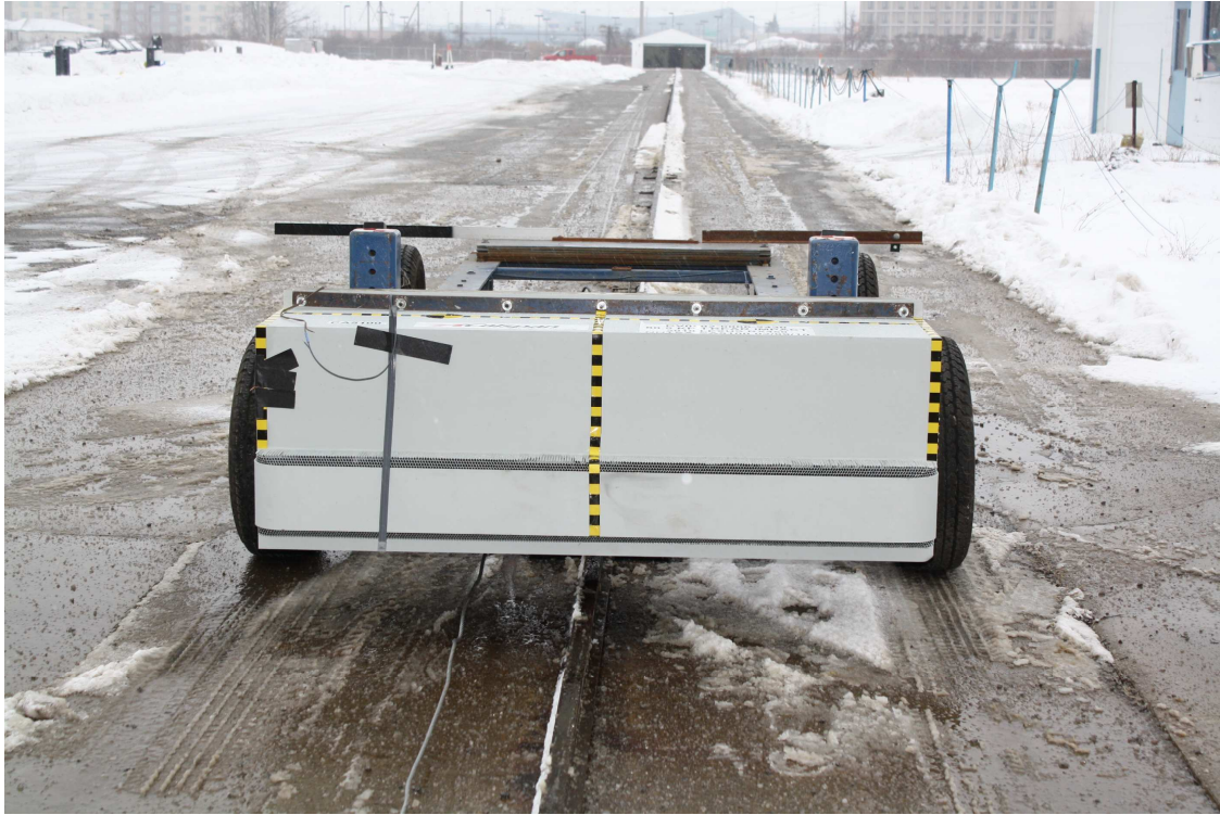
Figure A-23: Pre-Test MDB Front View
