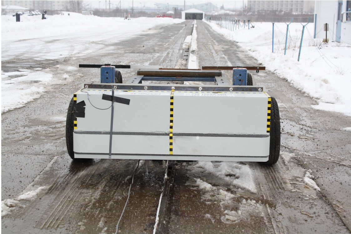
Figure A-19: Pre-Test MDB Front View
