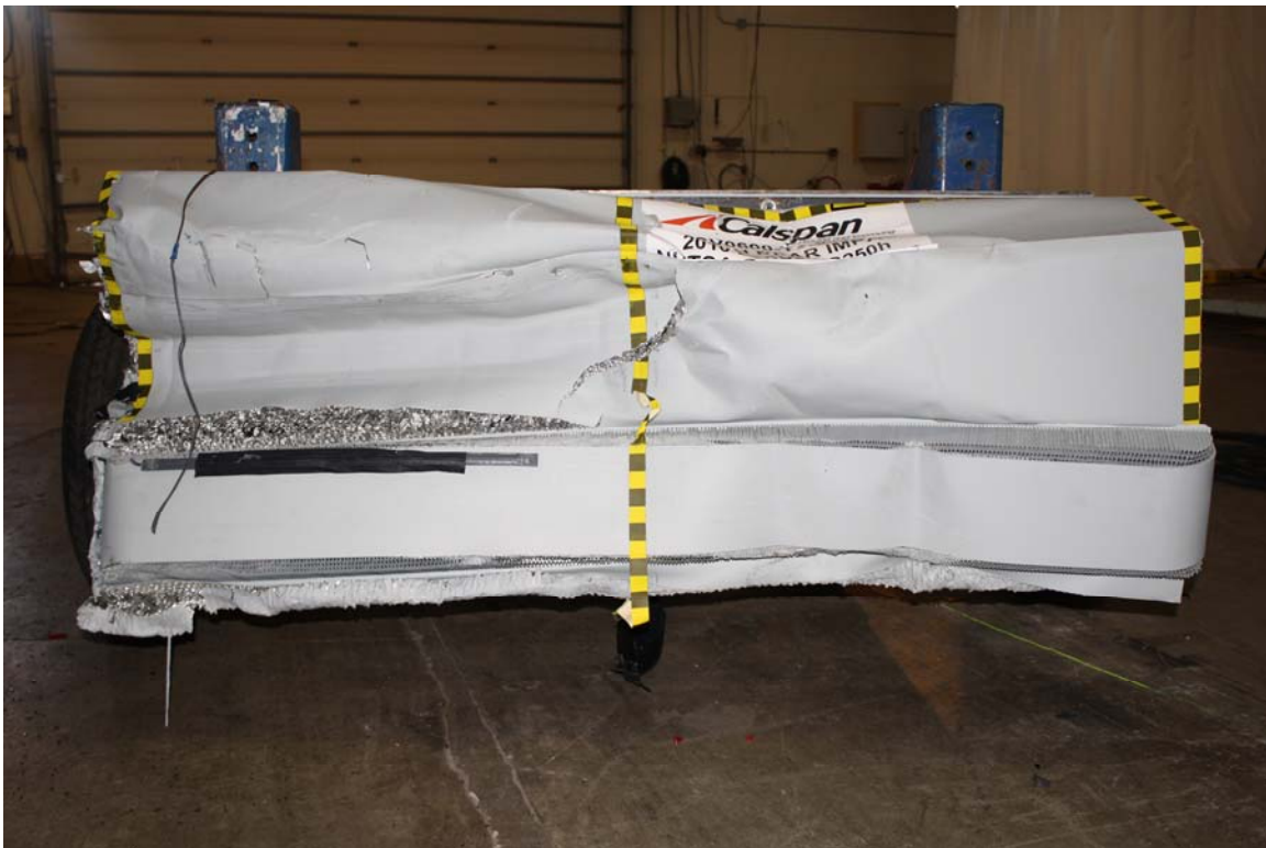
Figure A-20: Post-Test MDB Front View
