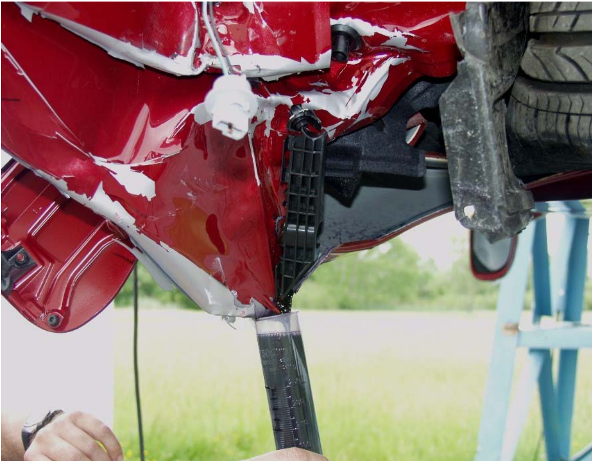
Figure A-42: leak collection at 90°
