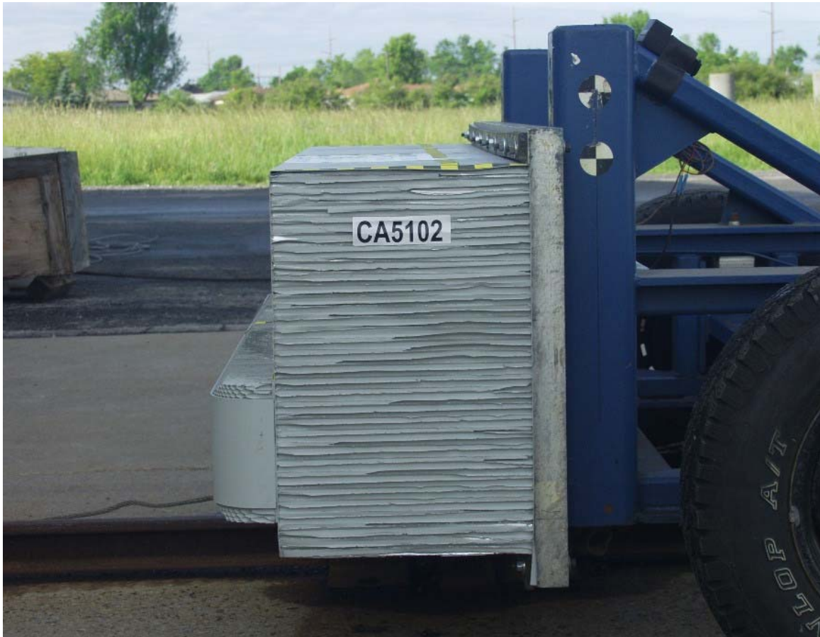
Figure A-21: Pre-Test MDB Left Side View
