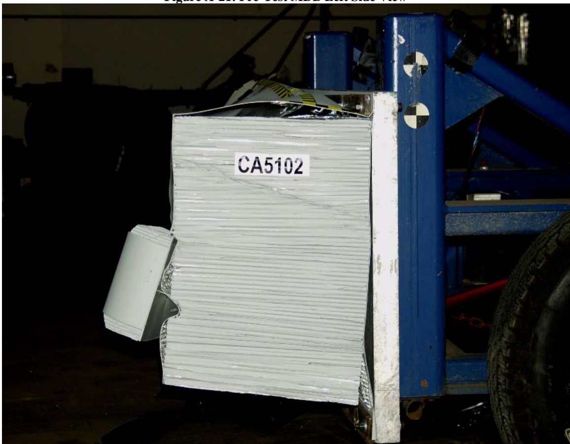
Figure A-22: Post-Test MDB Left Side View
