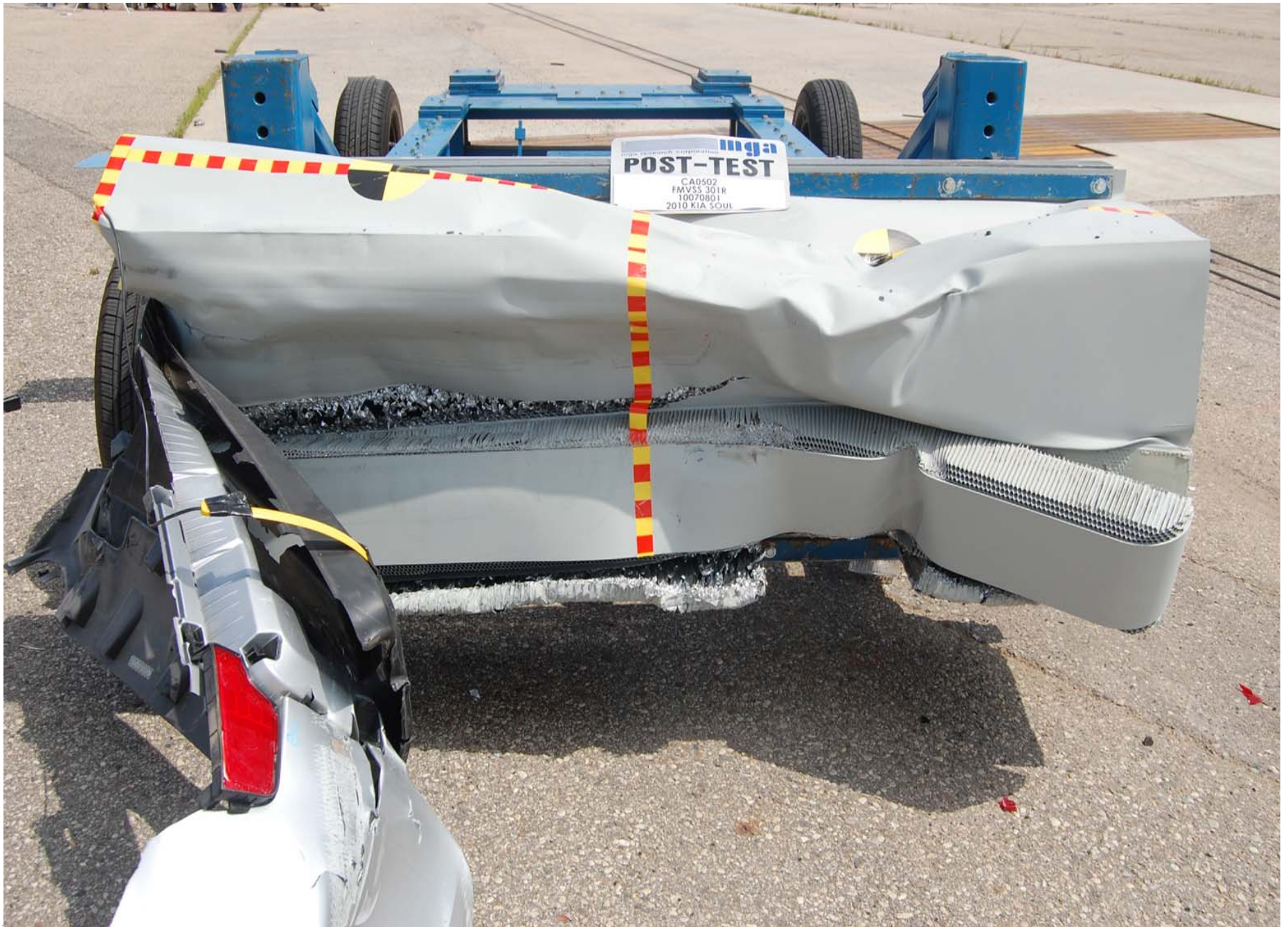
Post-Test Front View of MDB
