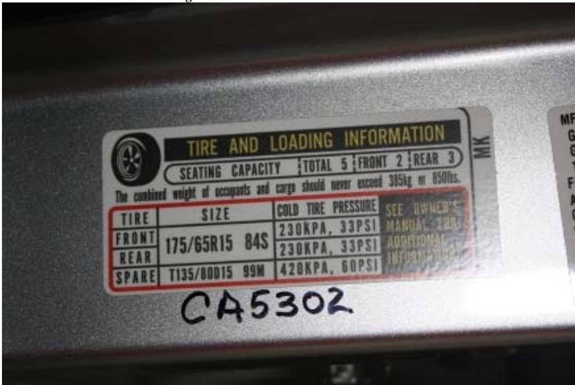
Figure A-2: Vehicle Tire Placard
