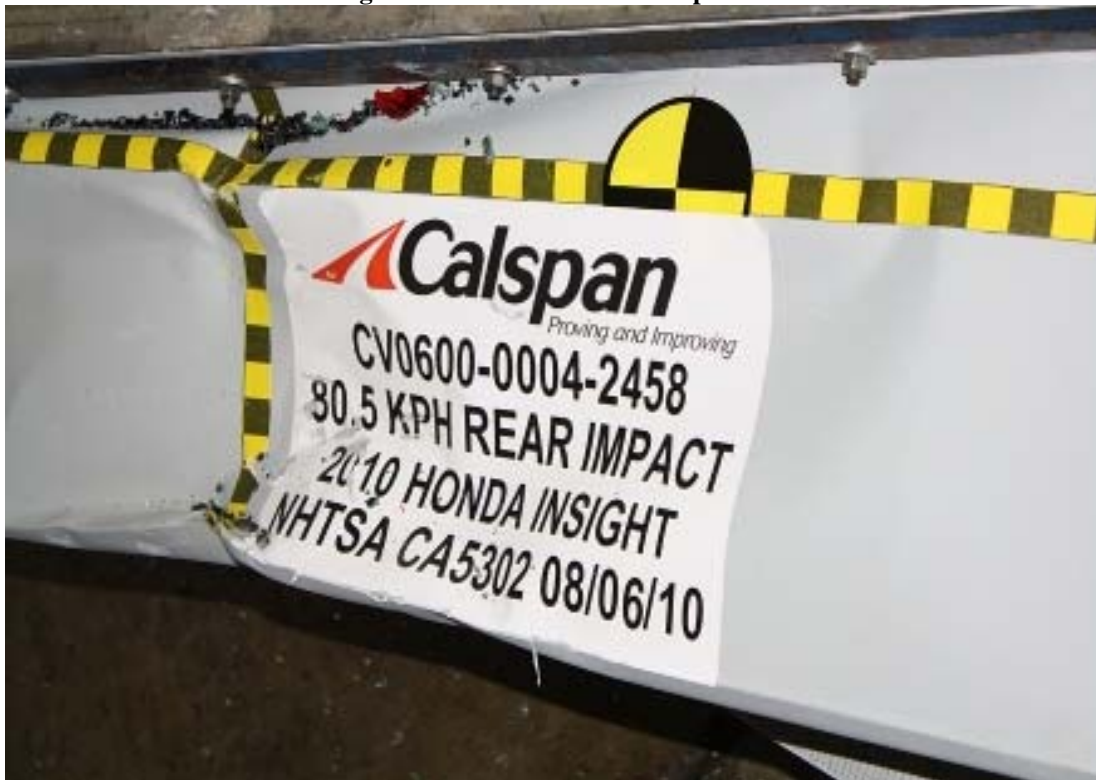
Figure A-26: Post-Test MDB Top View
