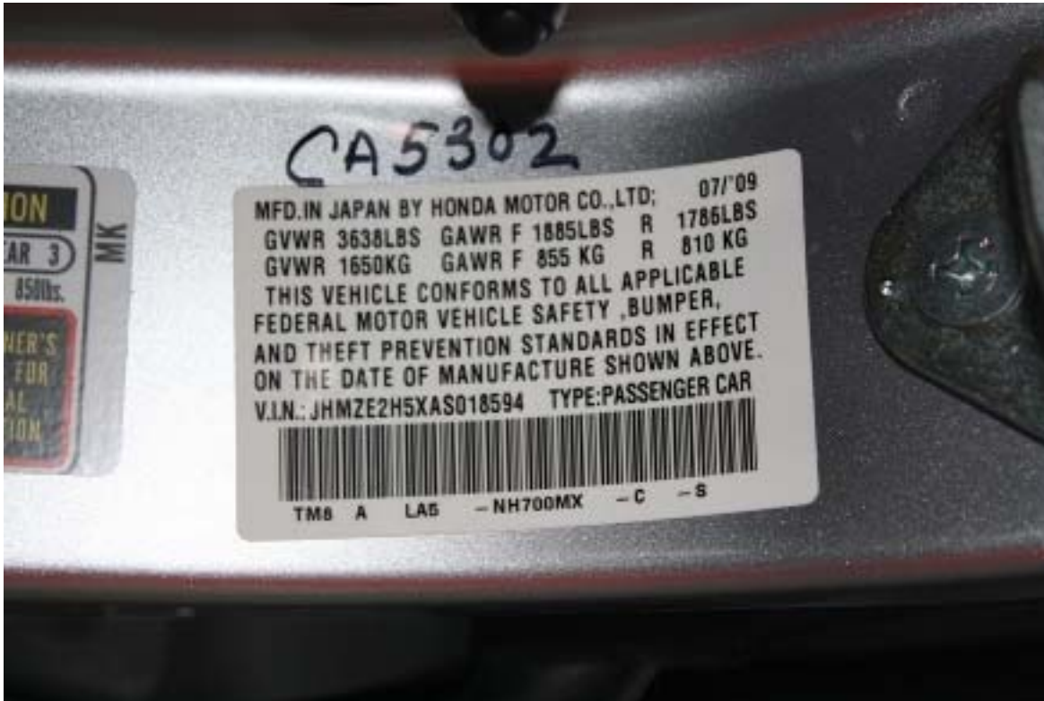
Figure A-1: Vehicle Certification Placard
