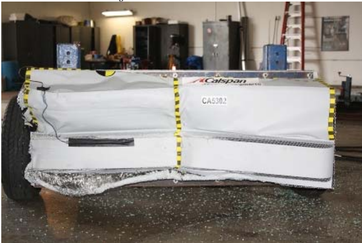
Figure A-20: Post-Test MDB Front View
