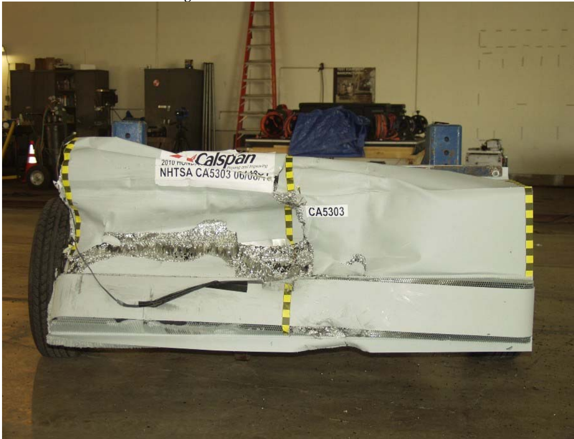
Figure A-20: Post-Test MDB Front View
