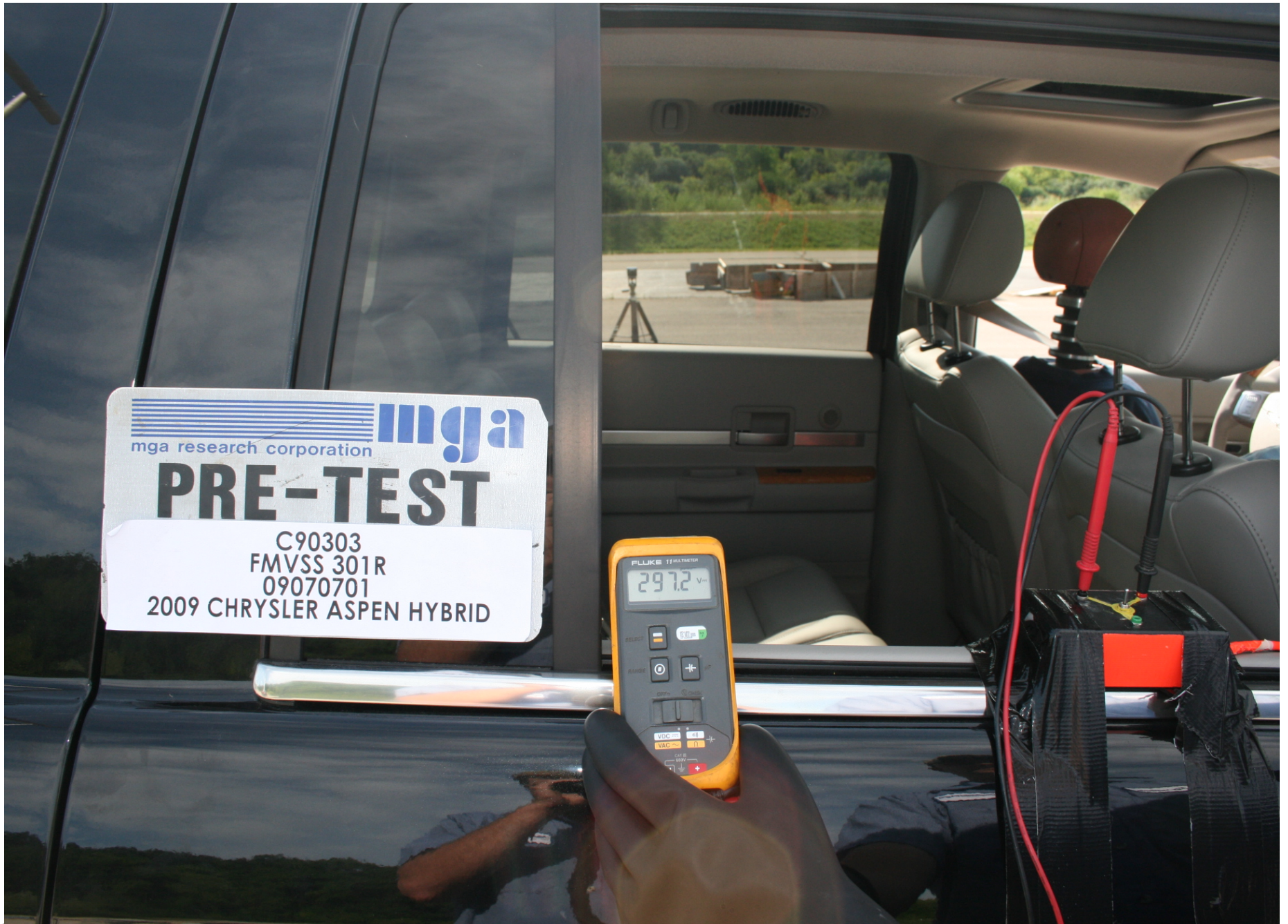
Pre-Test Installed Test Interface Port
