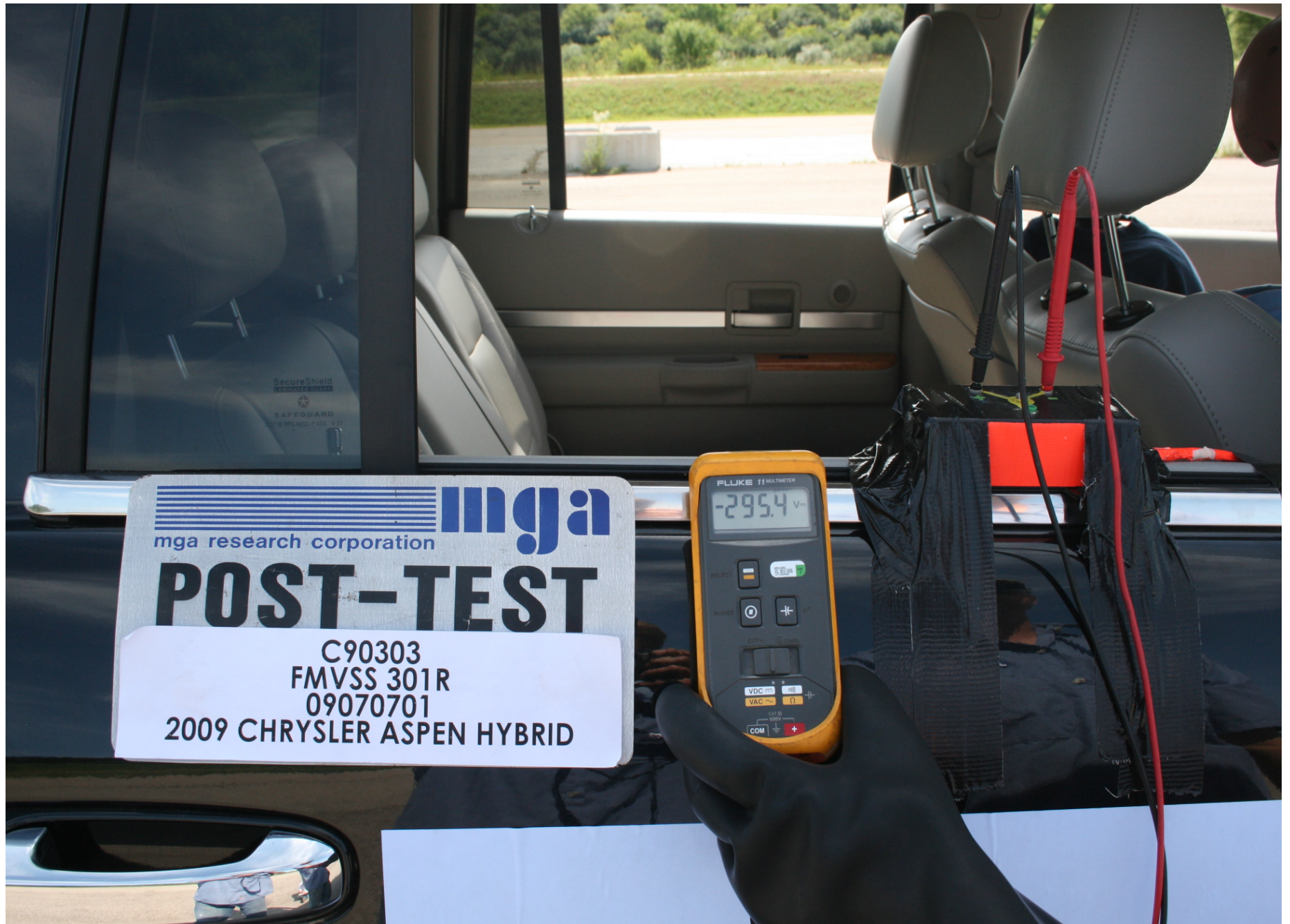
Post-Test Installed Test Interface Port
