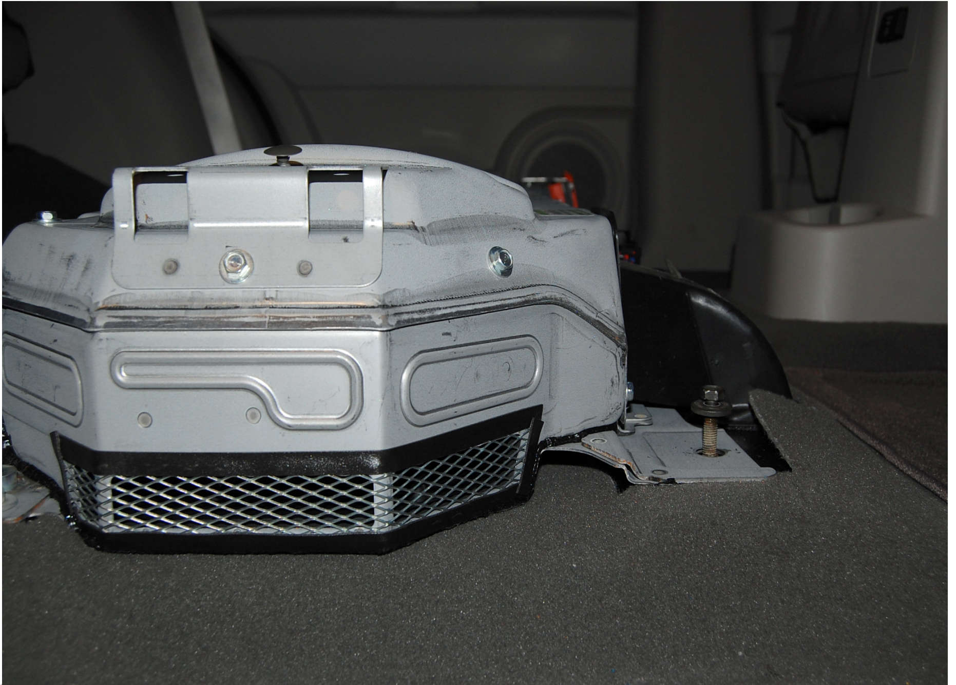
Pre-Test Forced Air Cooling System
