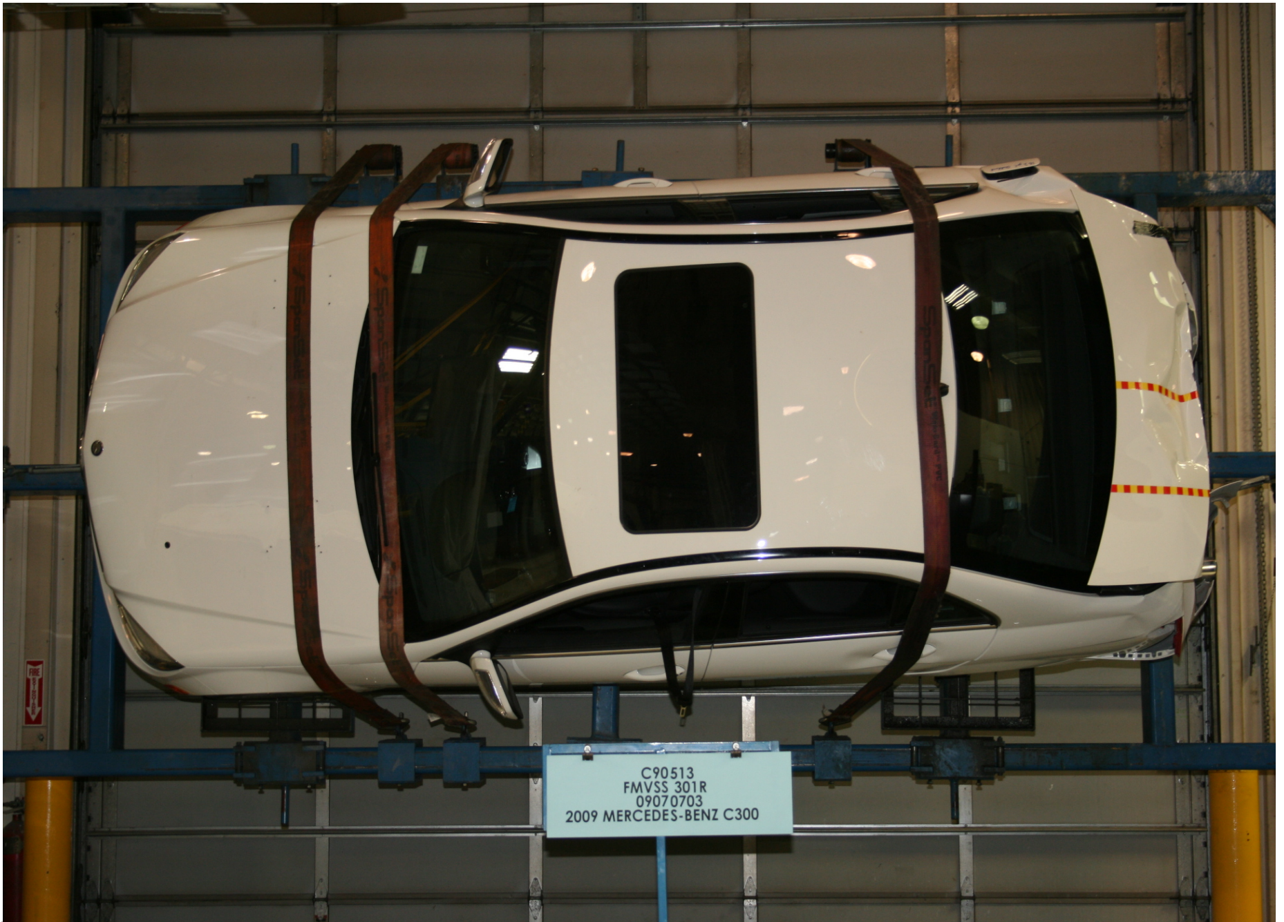
Static Rollover at 270 Degrees
