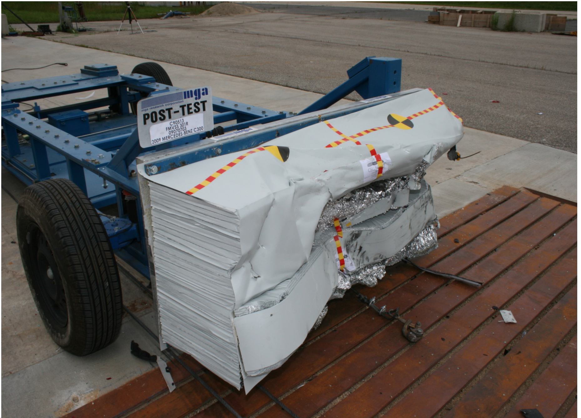
Post-Test ¾ Right Side View of MDB
