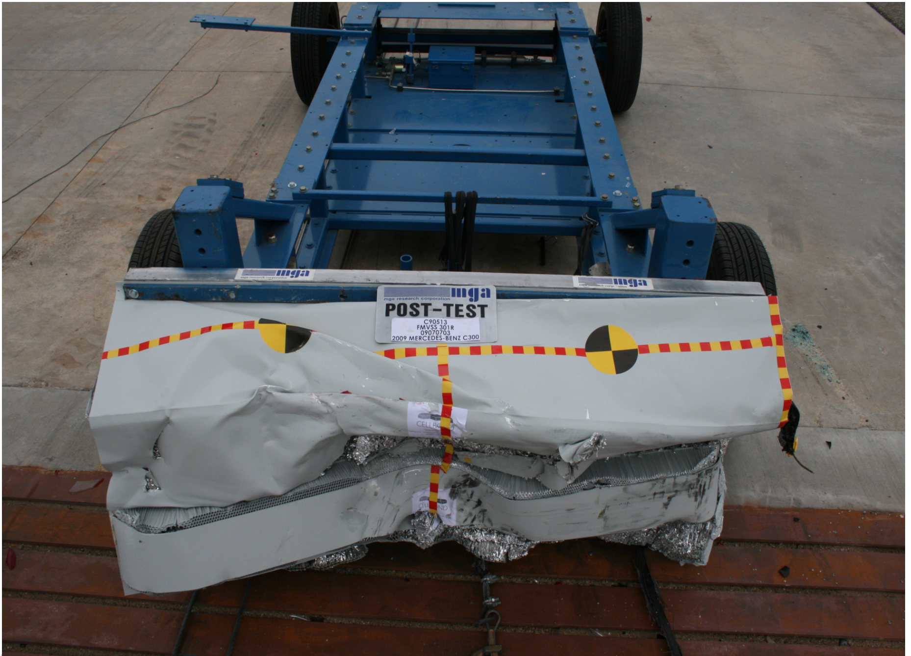
Post-Test Top View of MDB
