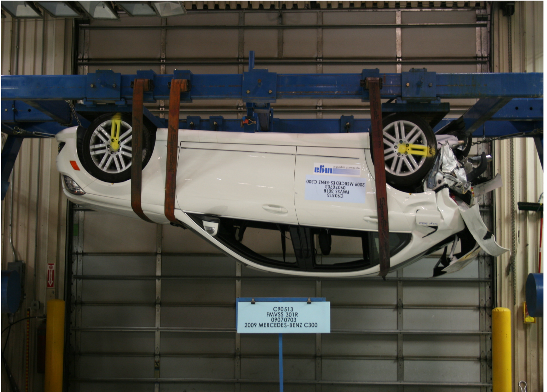
Static Rollover at 180 Degrees
