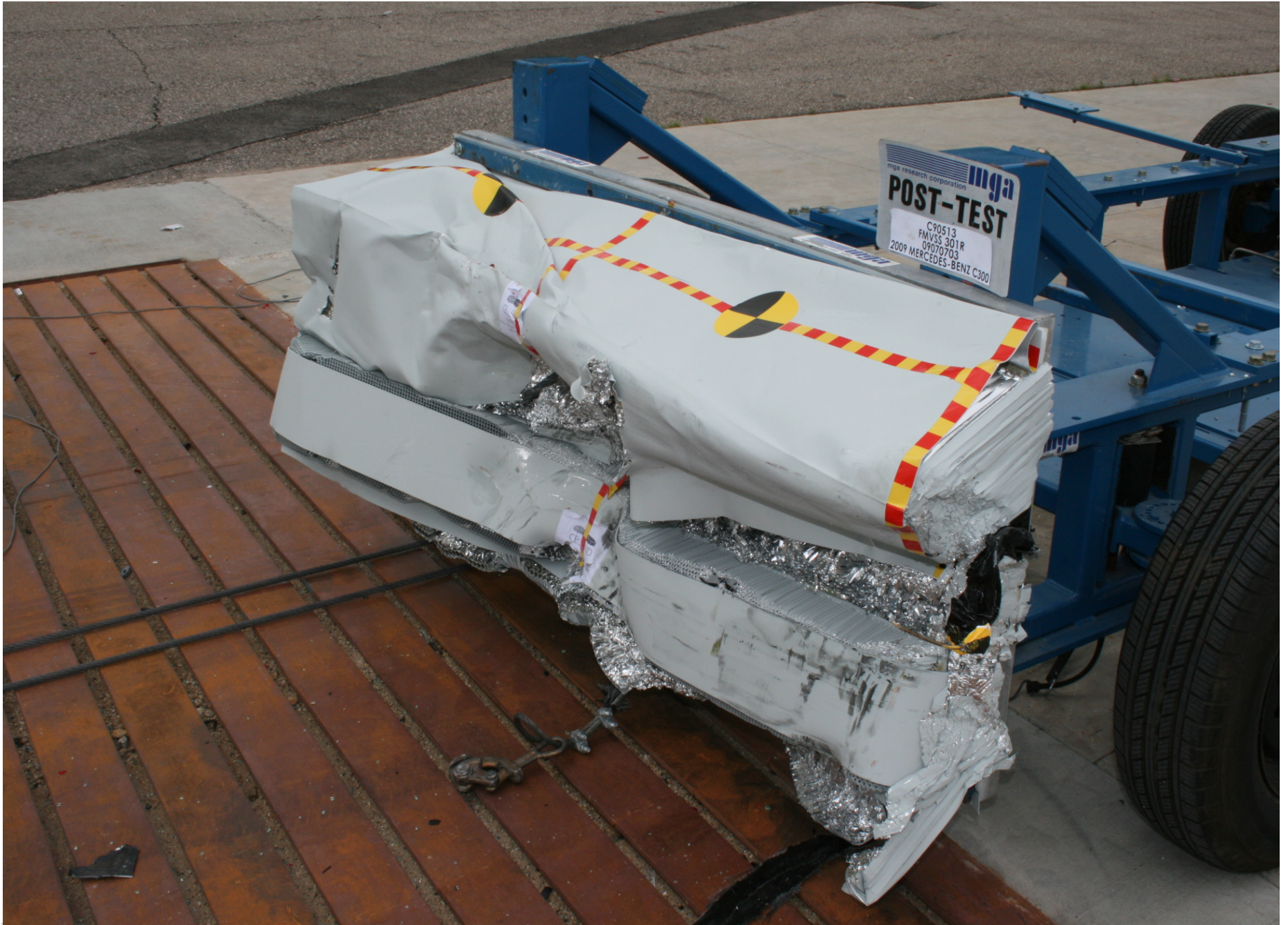
Post-Test \frac{3}{4} Left Side View of MDB
