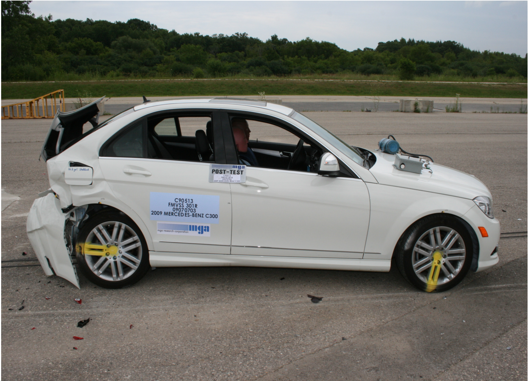
Post-Test Right Side View of Vehicle
