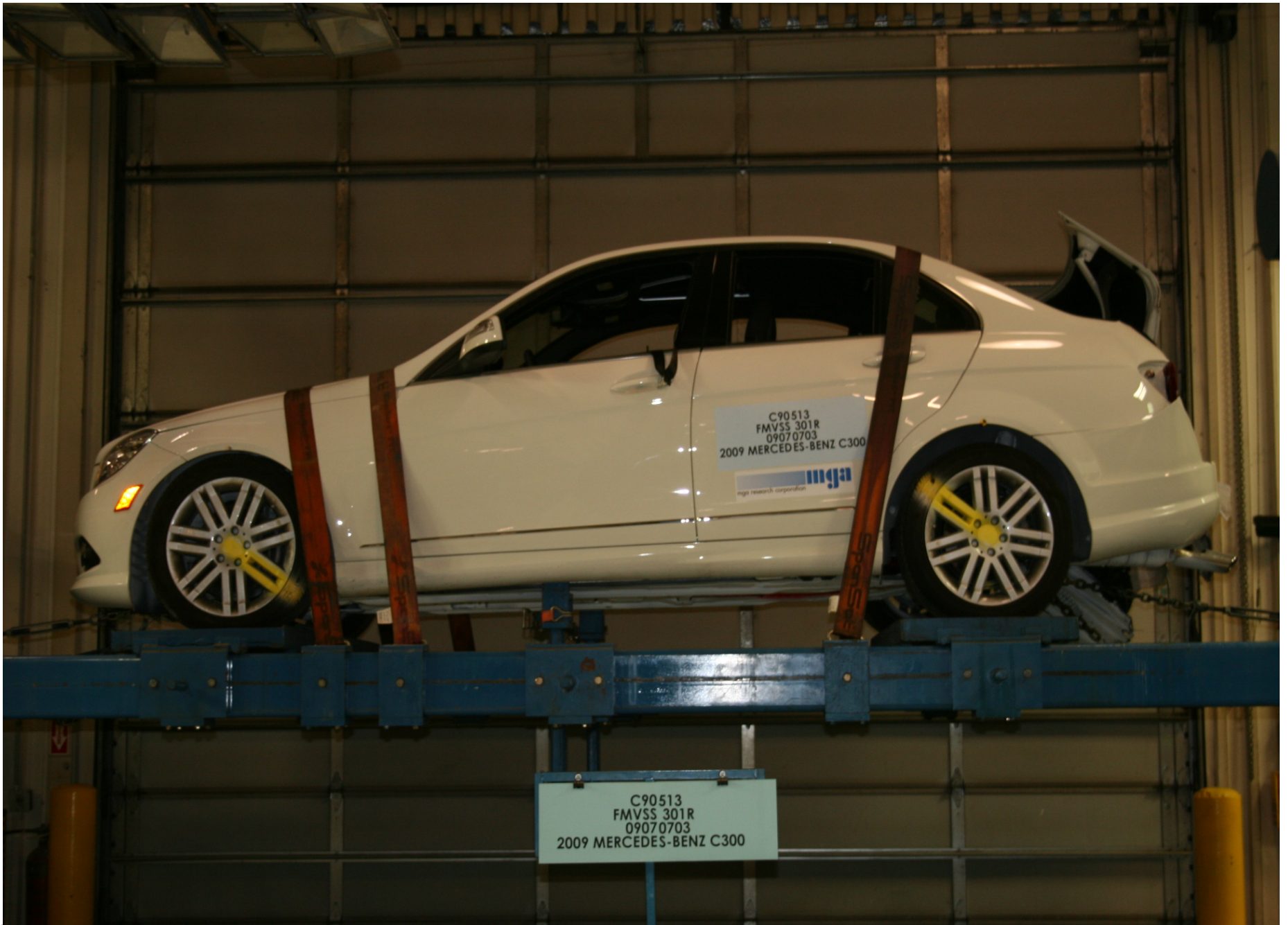
Static Rollover at 360 Degrees
