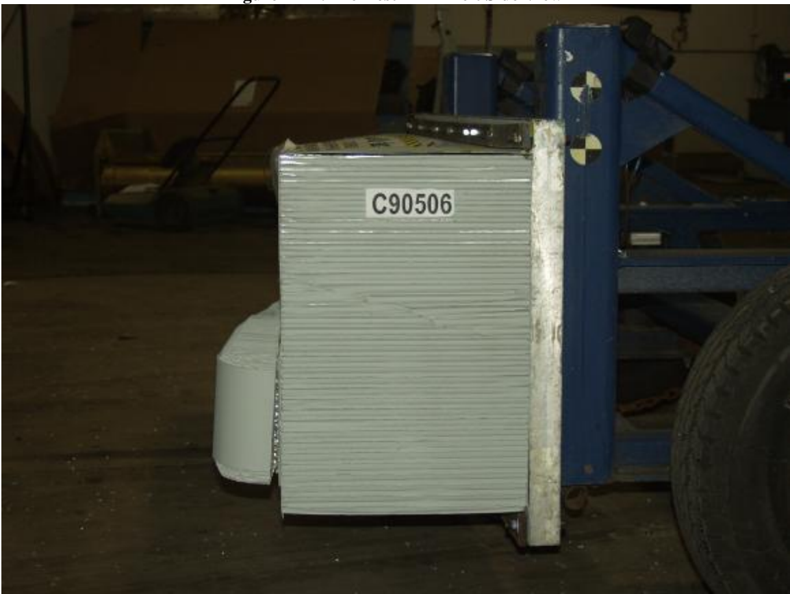
Figure A-22: Post-Test MDB Left Side View
