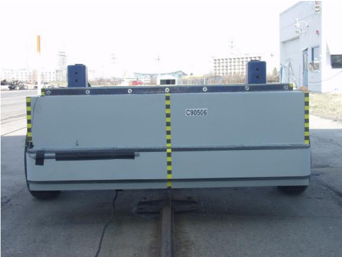
Figure A-19: Pre-Test MDB Front View
