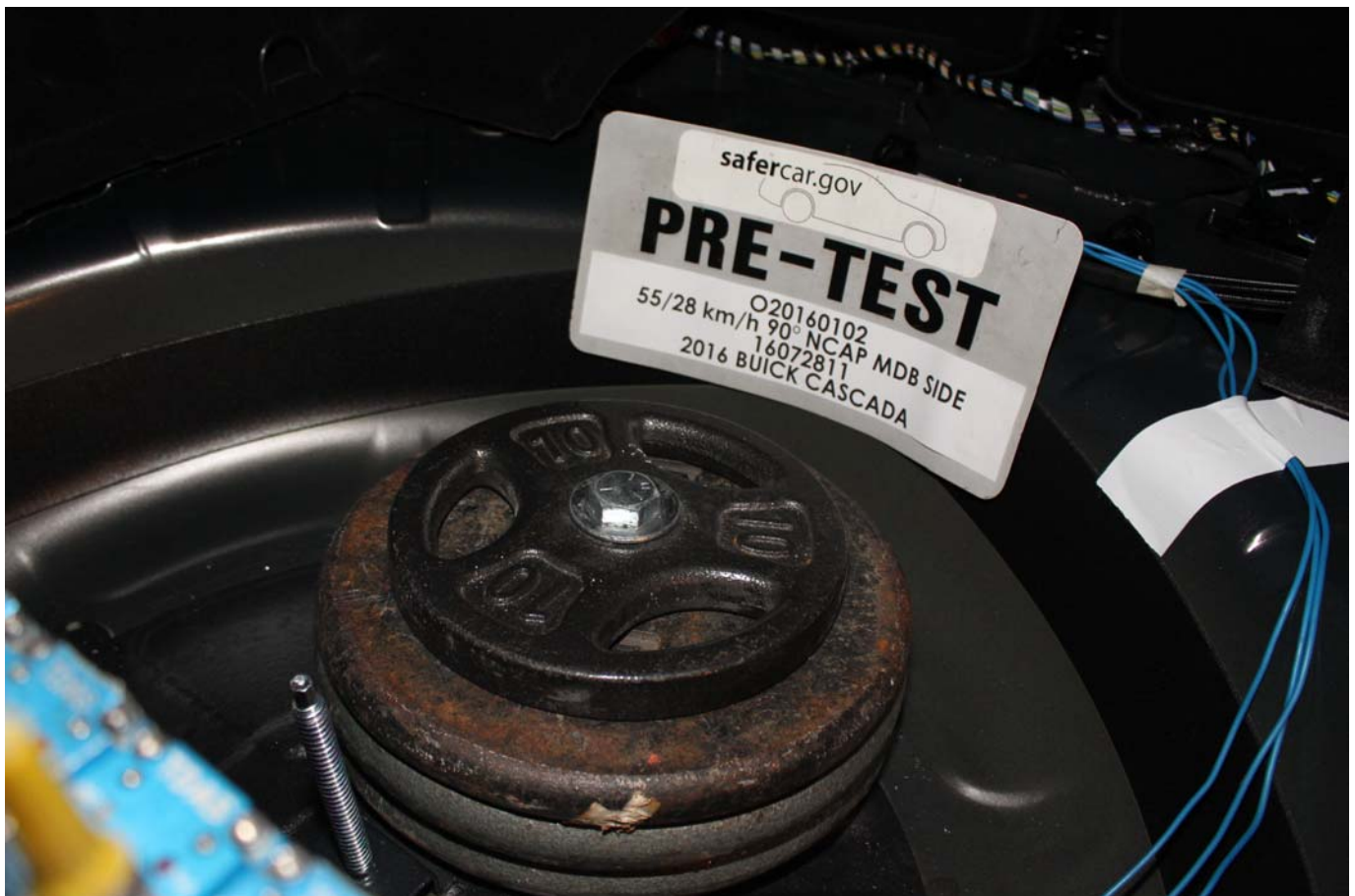
Photo No. 094 - Pre-Test Ballast View
