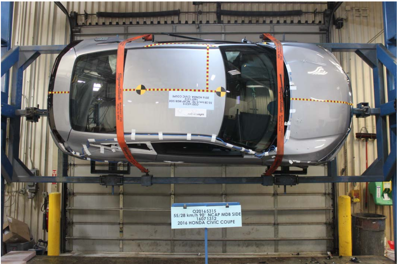
Photo No. 099 - FMVSS No. 301 Static Rollover 270 Degrees
