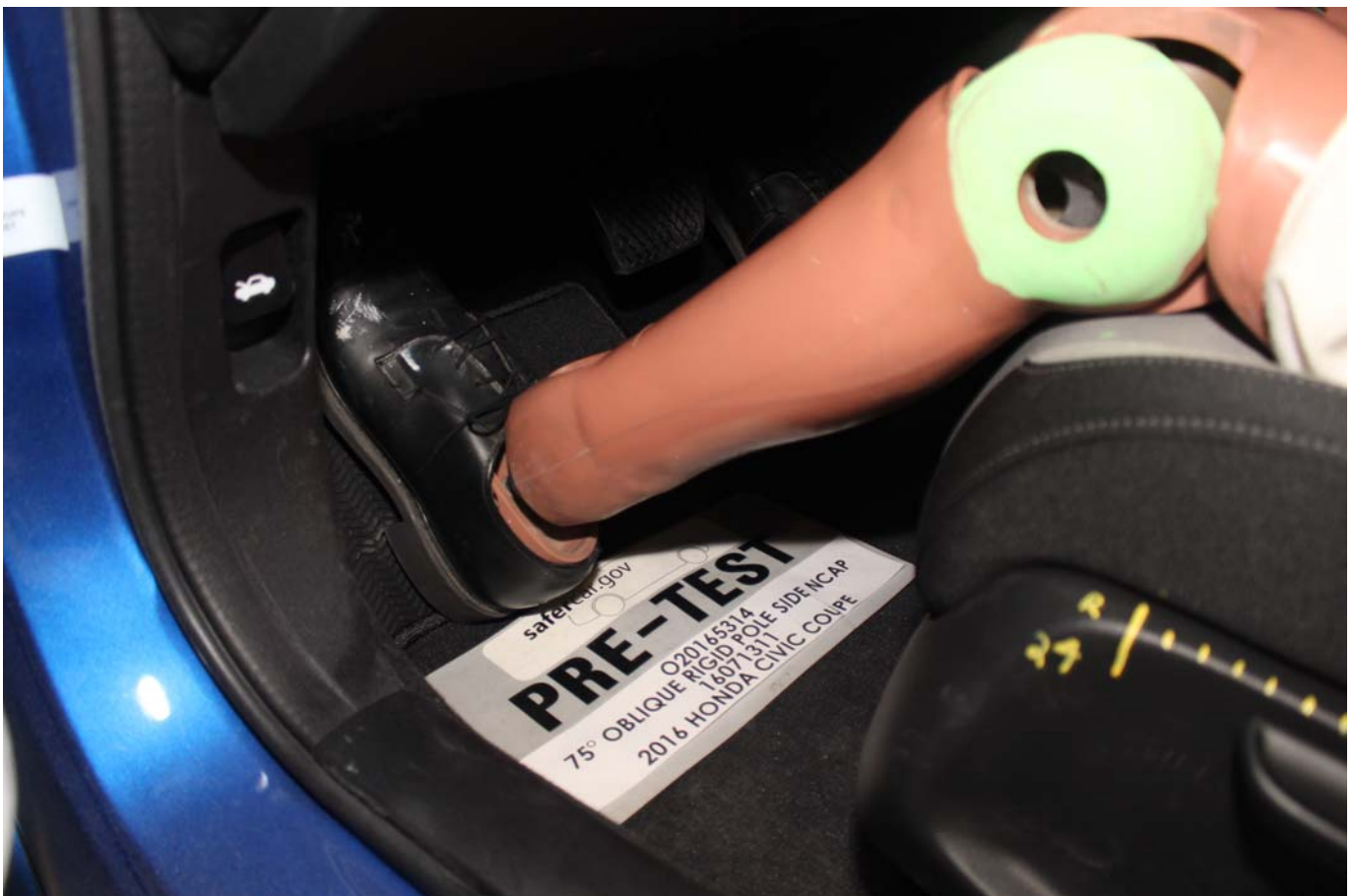
Photo No. 032 - Pre-Test Placement of Dummy's Feet
