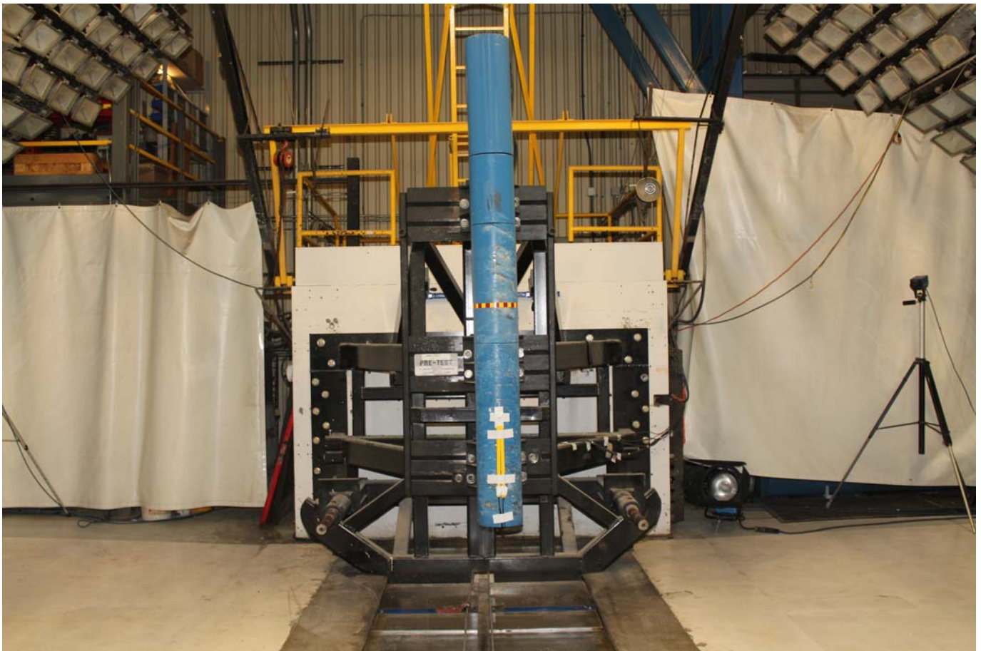
Photo No. 057 - Pre-Test Pole Barrier Front View
