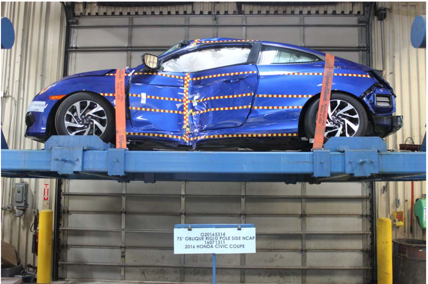
Photo No. 063 - FMVSS No. 301 Static Rollover 0 Degrees
