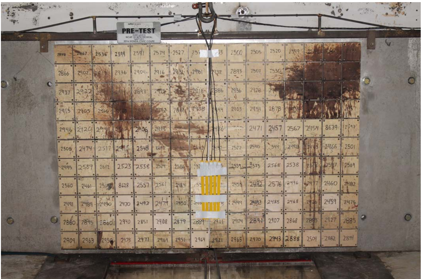
Photo No. 002 - Pre-Test Load Cell Wall
