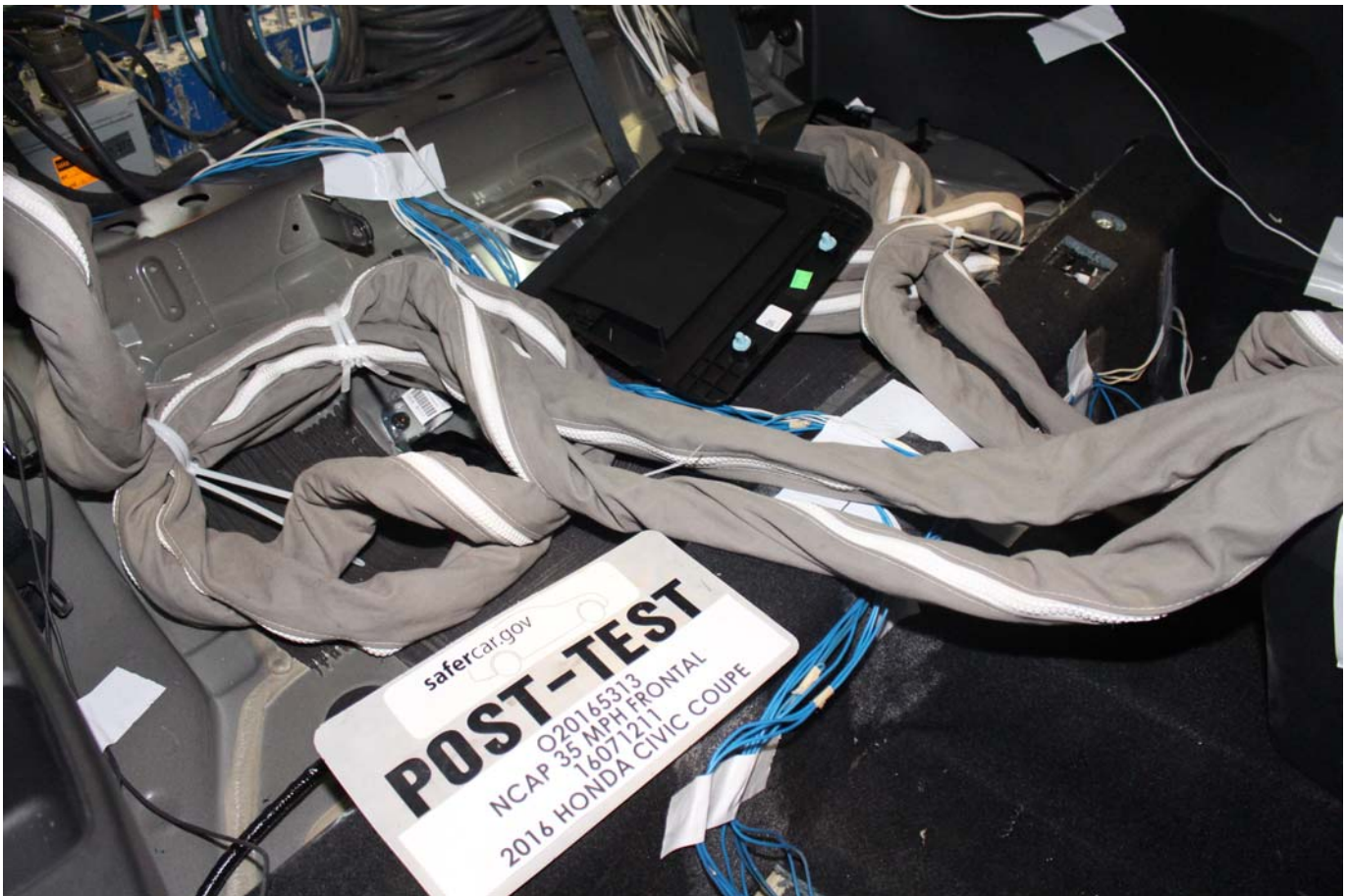
Photo No. 029 - Post-Test Dummy Cable Routing
