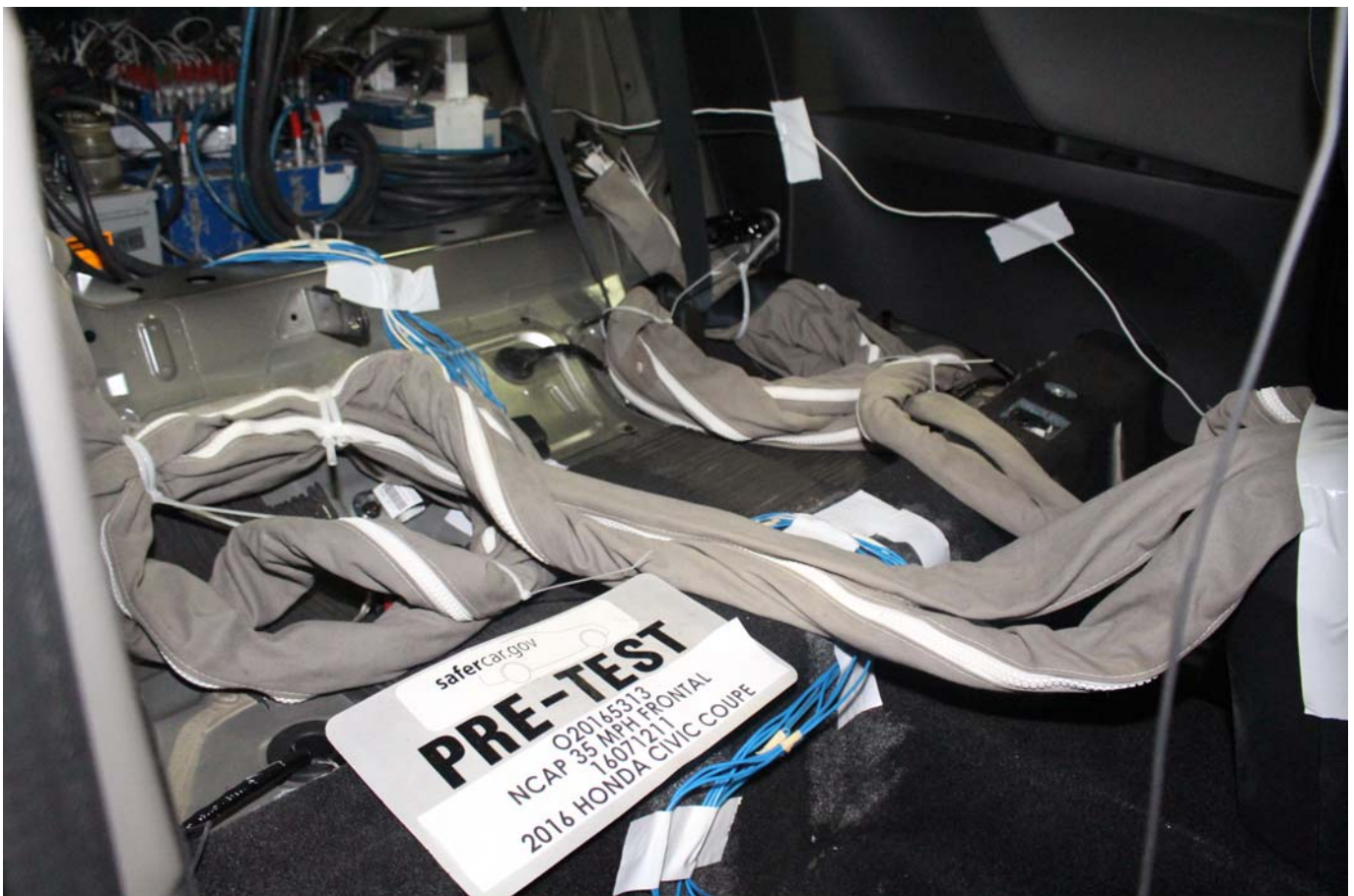
Photo No. 028 - Pre-Test Dummy Cable Routing
