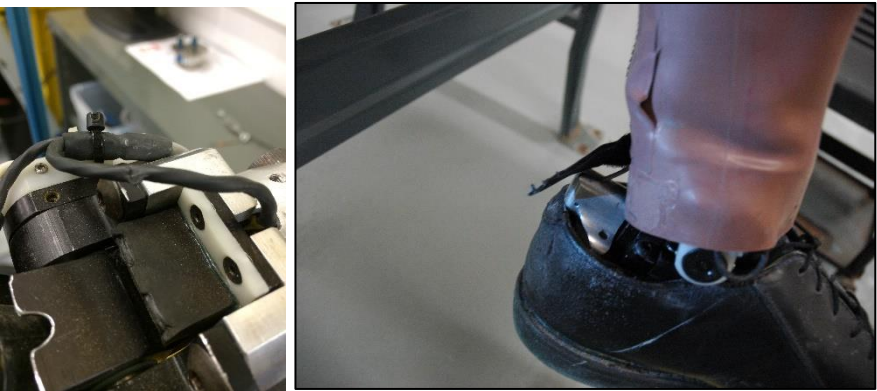
Ankle Z Potentiometer wire is pinched. Velcro strap torn from LH tibia flesh at ankle
