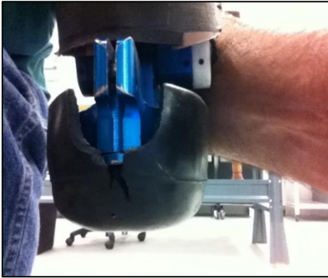
Left hand thumb cracked at base of thumb and pointer finger merge, Left hand cut at base of pointer finger outboard at knuckle
