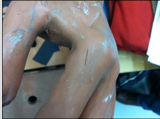
Left hand thumb cracked at base of thumb and pointer finger merge, Left hand cut at base of pointer finger outboard at knuckle
