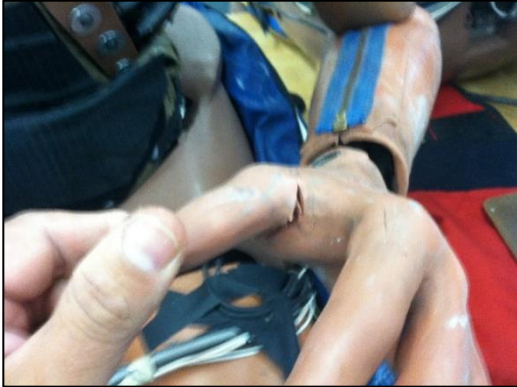
Left hand thumb cracked at base of thumb and pointer finger merge, Left hand cut at base of pointer finger outboard at knuckle
